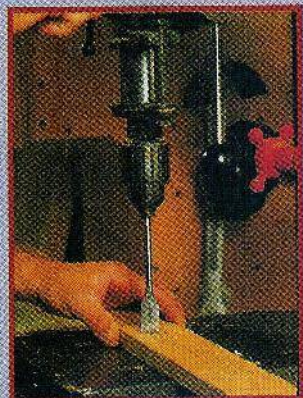
Fig. 2. Using the spade bit to countersink for the "T" nuts.
