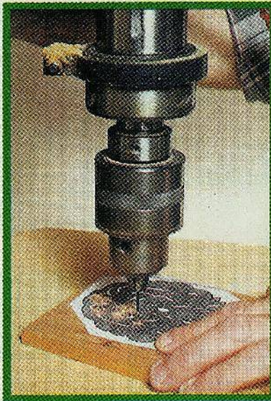
Fig. 1. Drill blade entry holes for the interior cuts.
