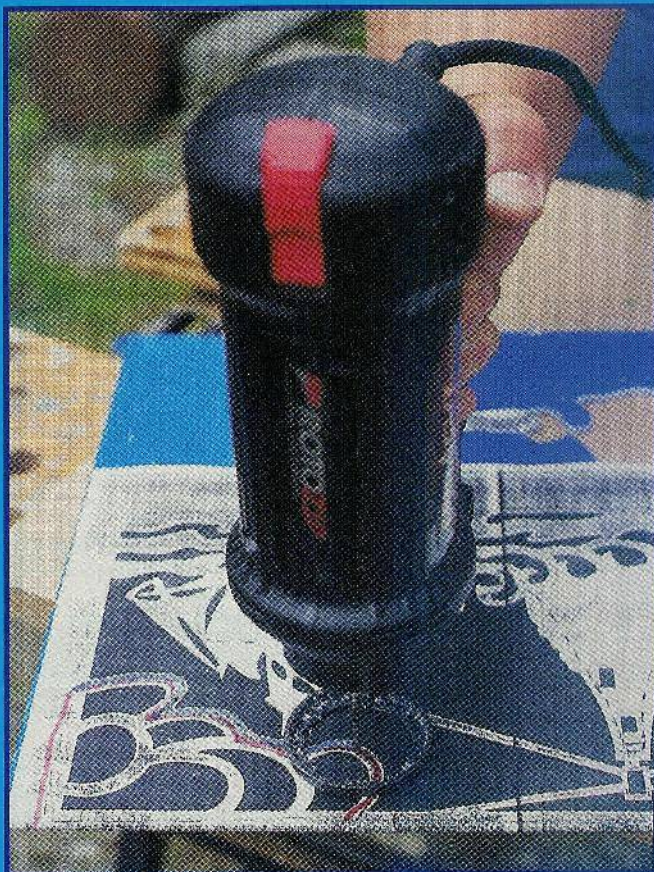
Fig. 1. Use the Rotozip SpirAcut spiral saw (or your scroll saw) to cut out the Plexiglas pieces.
