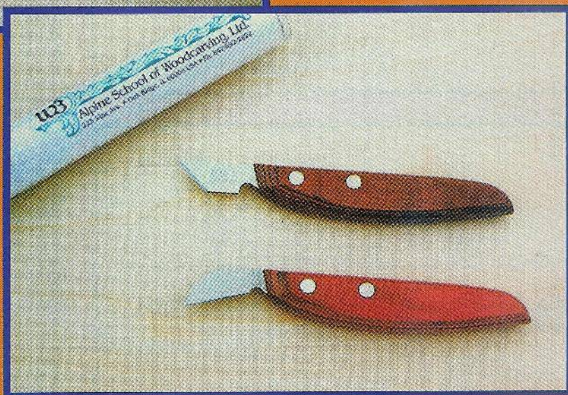
Fig. 2. Chip carving knives. The cutting knife (bottom) is primarily used to remove wood while the stab knife (top) is used for decorative purposes.
