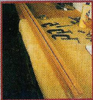
Fig. 1. Before cutting the two strips to final size, position them with their ends touching so that any space between them (caused by bowing) is kept at their mutual center. This is how the strips should be positioned in the finished Quilt Hanger.
