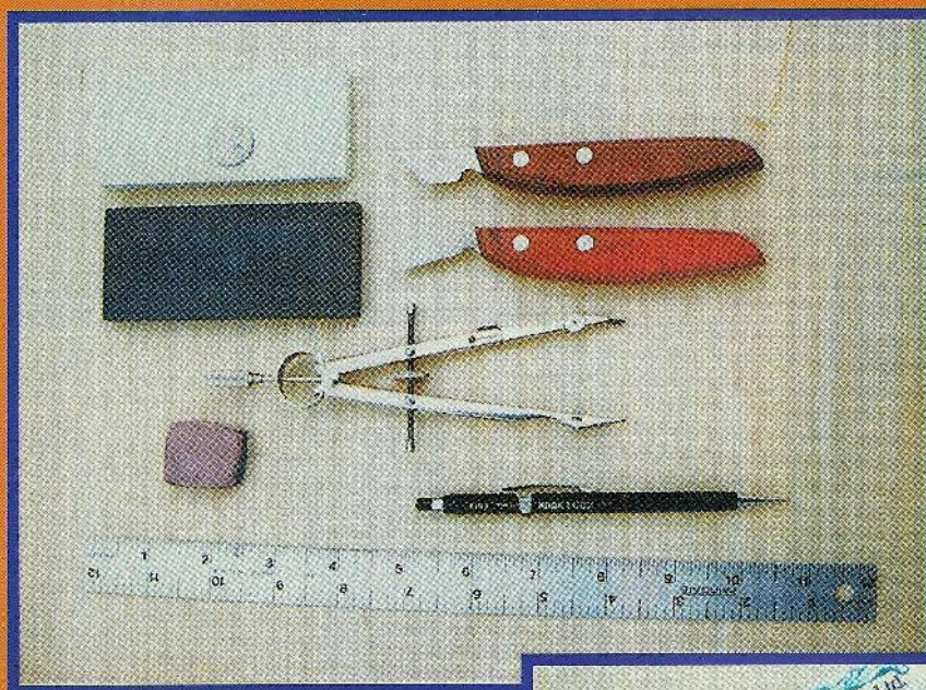
Fig. 1. For most chip carving projects, the only tools you need are: ceramic sharpening stones in medium grade and ultra-fine grade; a dime (to approximate the sharpening angle); a stab knife; a cutting knife; a compass; a mechanical pen; a ruler; an eraser.
