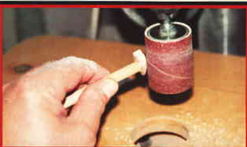
Fig. 4. Create a handle on small parts with a dab of hot glue on the end of a dowel rod. Leave the tongue attached until it's painted; cut through the glue line with a sharp knife to remove.
