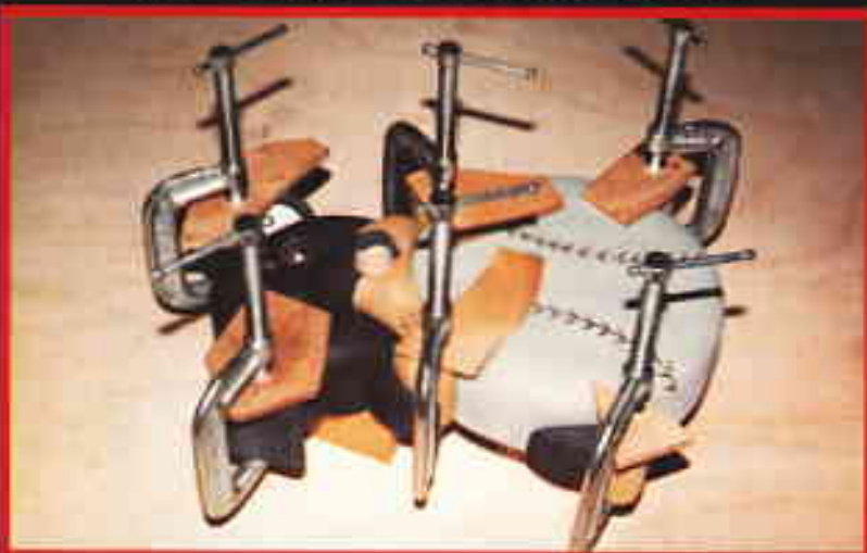
Fig. 6. A few C-clamps, with scraps of plywood to protect the surface, will insure a good bond to the backboard.
