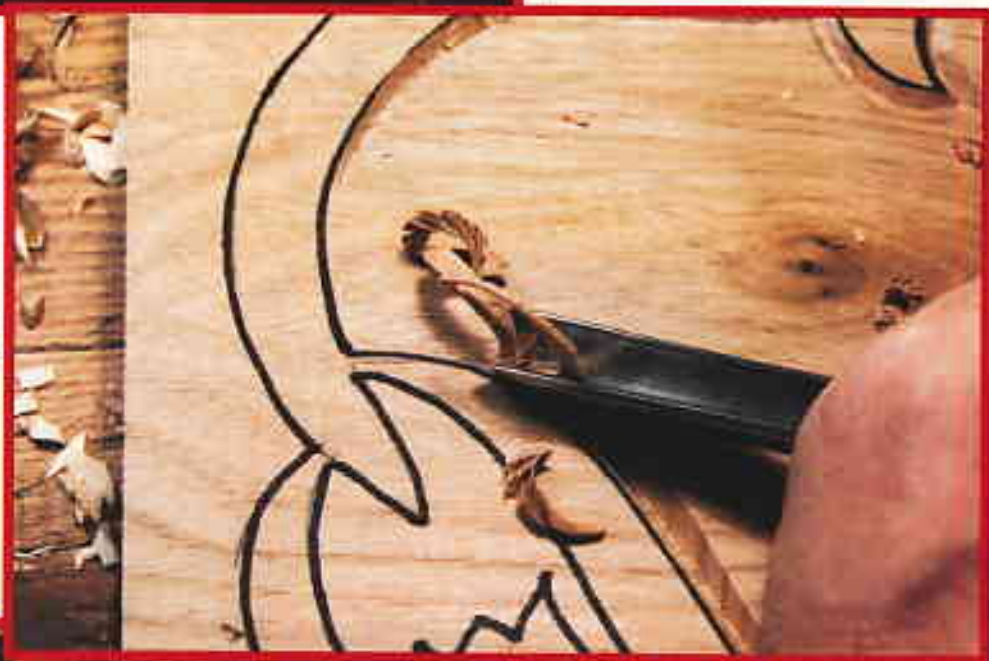
Fig. 2. Making a stop cut. Always use the largest tool you can (in this case, the 16mm V-tool).
