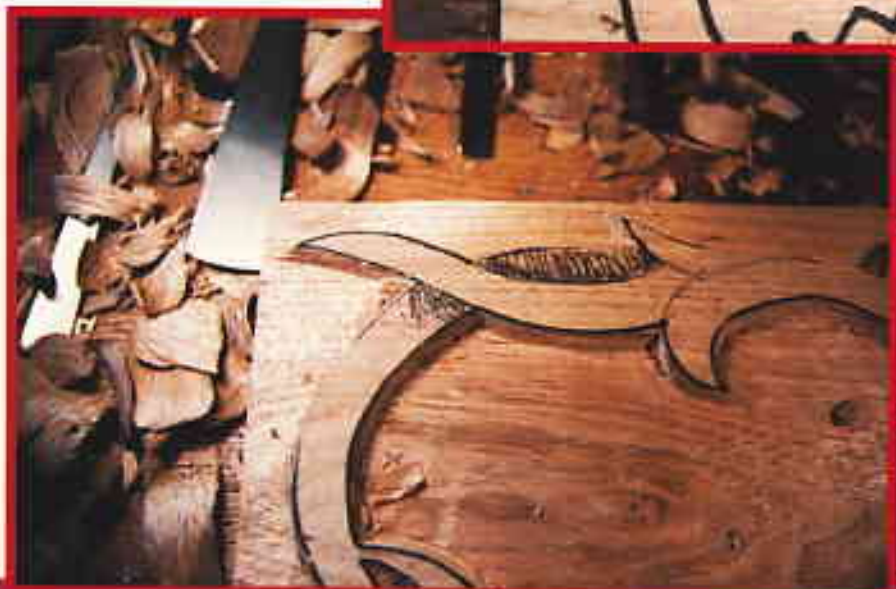
Fig. 3. After removing the background wood, study the different levels of the pattern. In better discern each level of the pattern, shade the lower portion of each overlap.
