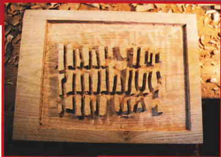
Fig. 1. Trace the pattern onto the wood. When routing out the back, be sure to leave a few islands to support the piece while carving.
