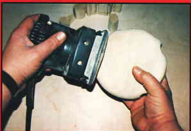
Fig. 3. Use a finish sander to contour and smooth the ball and puppy's head.
