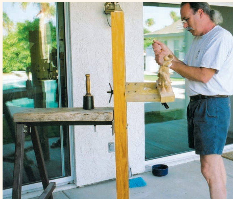
A carver's frame allows the carving to be rotated both horizontally and vertically.
