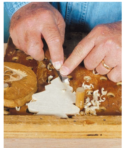
A carver's bench hook uses cam clamps to secure a carving without getting in the way of the tools.
