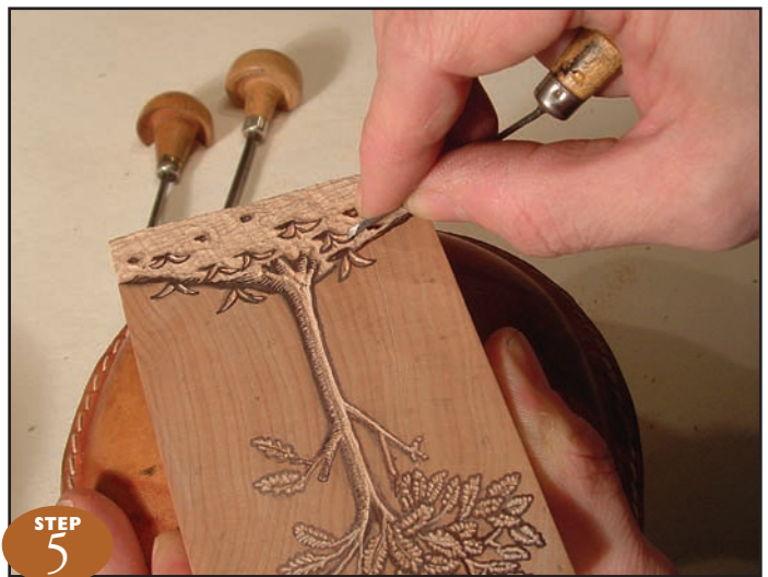
STEP 5 Detail the engraving with the burin and the spitssticker.
