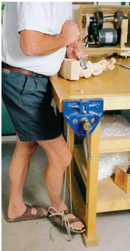
A rope clamp is a cost-saving device that puts a strong hold on a carving.
