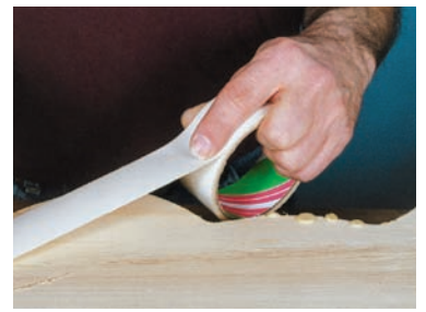
Double-sided carpet tape offers a secure bond between a large relief project and its backing board.
