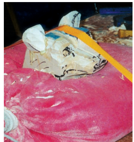
Russ Robinson's sandbag and web clamp make for a sturdy, but flexible, holding fixture.
