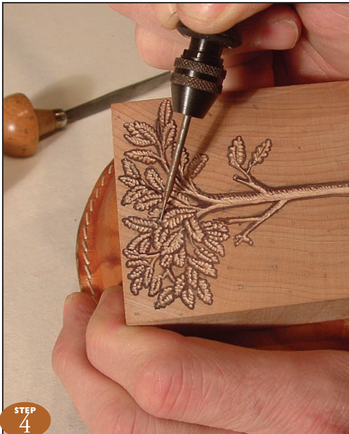
STEP 4 Use a \frac{1}{32} "-diameter ball-tipped bur to rough-out the smaller, open areas.
