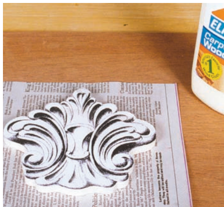
Newspaper and glue secure a small relief project to a backing board.
