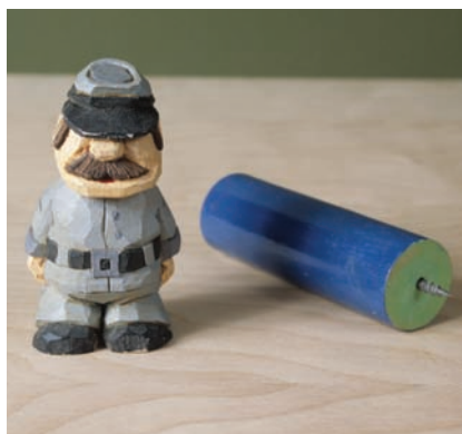
Elmer Jumper's hand vise has a screw on one end to accommodate a small project for carving or painting.
