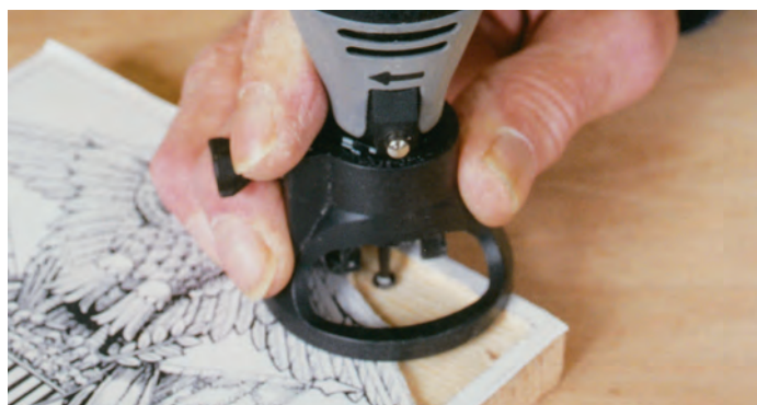
A handheld grinder like the Dremel and a routing attachment are easy to use when removing background on a relief carving.
