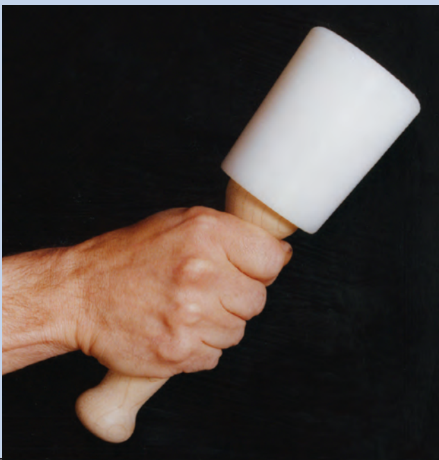
The hard head mallet, made from polyethylene, is virtually indestructible.
