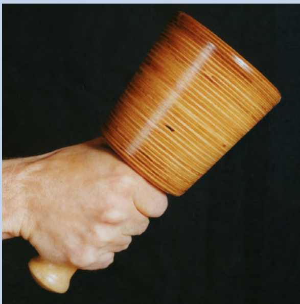
Lignostone is made from layers of beech veneer-bonded together under high pressure with a synthetic resin.
