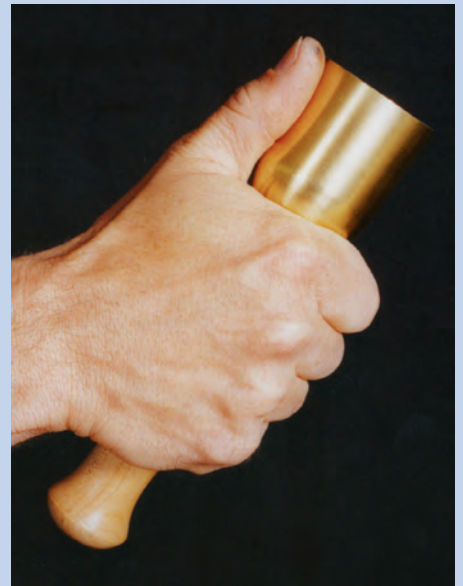
This bronze-headed mallet offers a solid blow with little rebound. The best grip is with the thumb behind the head and rest of the fingers wrapped around the head.
