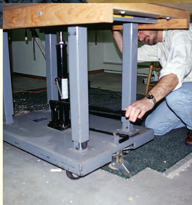
A hydraulic post lift table is used to adjust the height of Ernest's workbench.
