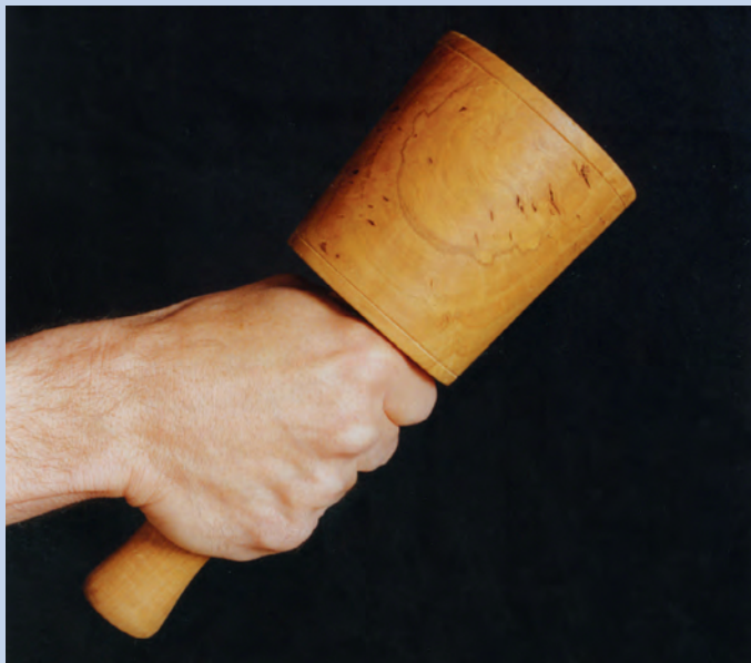
A custom-made mallet, this one has an oak burl head that is extremely hard and dense.
