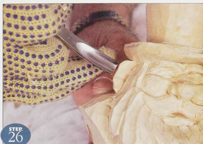
A no. 6 1/2-in or 5/8-in. gouge is an excellent tool for hollowing the ears.
