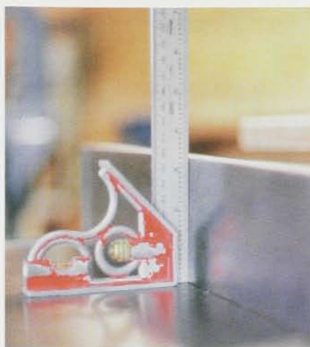
The camber method of joining panels for relief carving requires setting a jointer fence 1 or 2 degrees from its vertical position.
