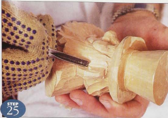
Separate the sideburns from the ears using the 60-degree V tool.
