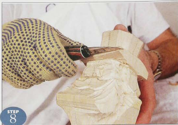
Carve away wood from the underside of the hat brim using the knife.
