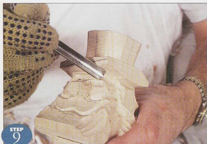
Using the number 9 8mm gouge, remove wood from the temples to accentuate the cheeks.
