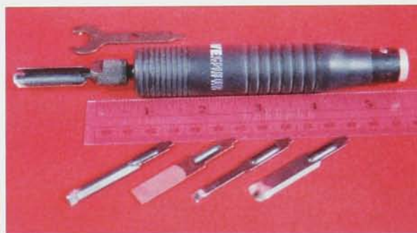
The Wecheer reciprocating handpiece accepts Warren Cutlery as well as Flexcut chisel bits.
