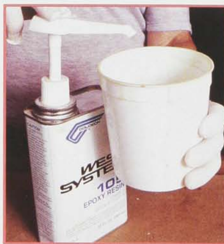
Two-part West System, a marine epoxy, is dispensed with pumps that pre-measure the amounts of resin and hardener required.
