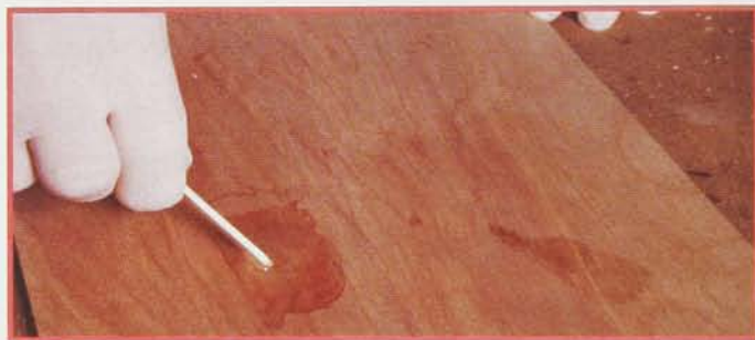
The two parts of an epoxy are vigorously mixed together. Wearing disposable or latex gloves should be mandatory when working with epoxy.
