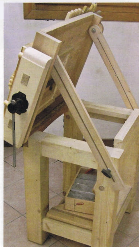
Adjust the angle of the table top and lock it in place with the adjustable knobs.
