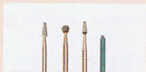
Texturing bits from left: small taper green stone, small ball green stone, small tapered stone with a rounded tip, blue ceramic rod
