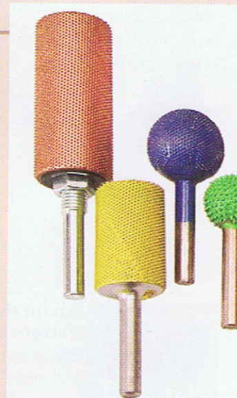
For large carvings, use large carbide-point bits, from left: fine cylinder sleeve, fine cylinder, fine ball, coarse ball
