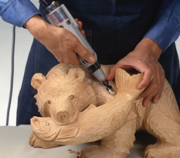
Reciprocating power carvers add hammer-like action to traditional-edged tools.
