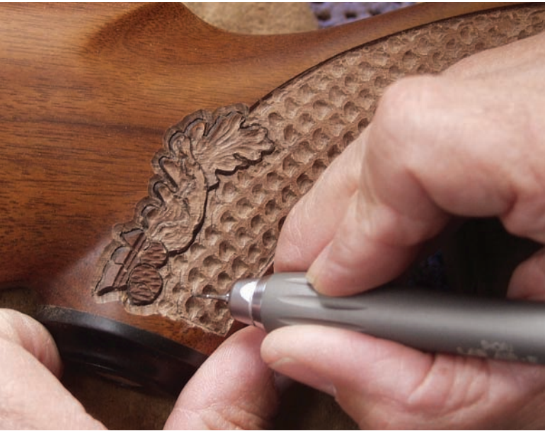
Air turbine units provide precision control for carving materials such as wood, egg shells, and glass.
