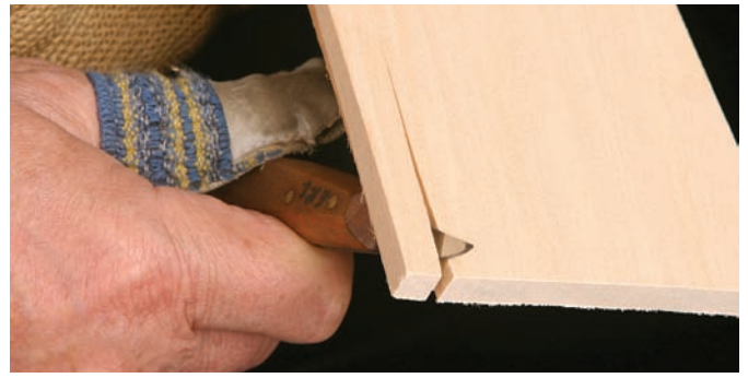
When a knife is allowed to wedge between the vessels, the vascular rays tear, and the vessels split from one another.
