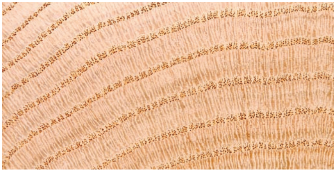
Horizontal vascular rays connect the vertical vessels together. These rays are clearly visible in this piece of oak.
