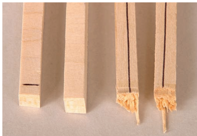
The pieces with short vessels split under very little stress. The pieces with long vessels broke under much more stress.
