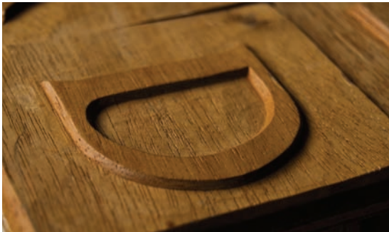
The same relief techniques are used to carve traditional letters, such as this “D.”
