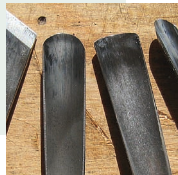
Helli rounds the corners of his gouges for maximum performance.
