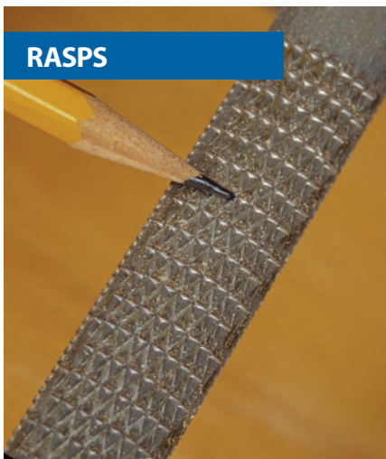
The coarse teeth of a rasp resist clogging.
