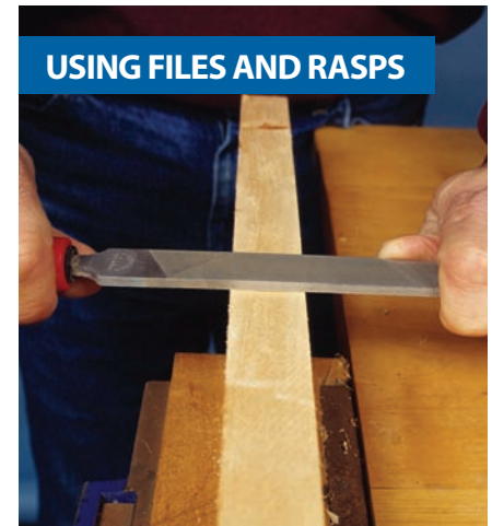
Draw filing cuts on the push stroke.
