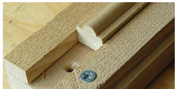
A simple, shop-made vise holds the blank in place.
