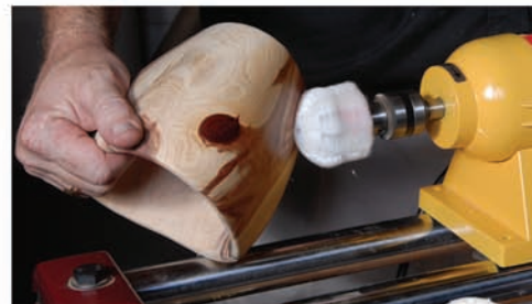
Guinevere® Inflatable Sanders conform to the shape of the material they touch.
