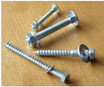
Carriage bolts and lag screws can be used to assemble a simple, yet solid, carving bench.
