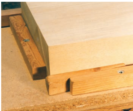
A block of wood held by fences and wedges which are easily removable.
