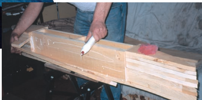
After gluing the head section, the side panels are attached to create the final width of the fish's sides. Then, the layers for the tail section are glued into position.
