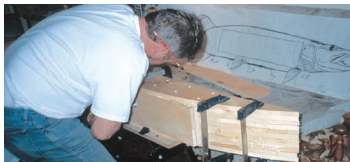
While glued layers of pine are setting, clamps are added to ensure a tight bonding.
