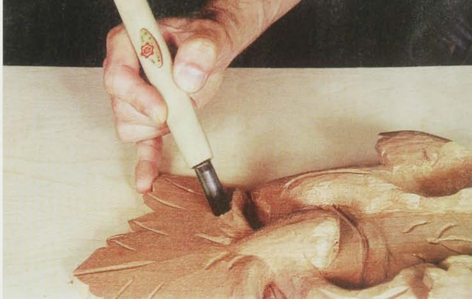
Made in Japan from laminated steel, this long-handled, short-bladed gouge offers a superb cutting edge.
