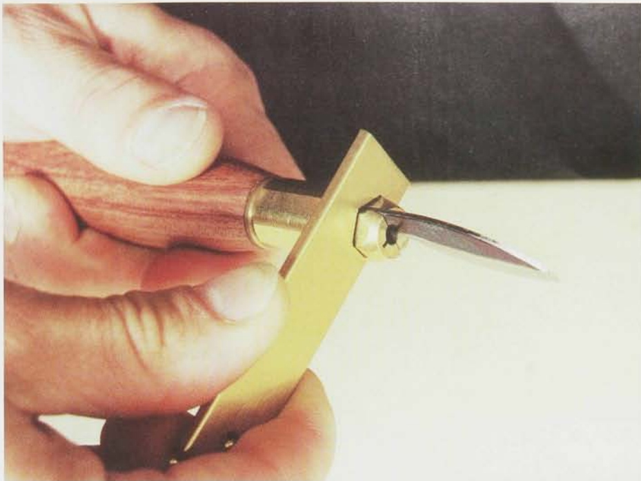
A unique feature familiar to many carvers is Warren's threaded brass lockjaw, tightened with a wrench that accepts a wide variety of interchangeable blades.
