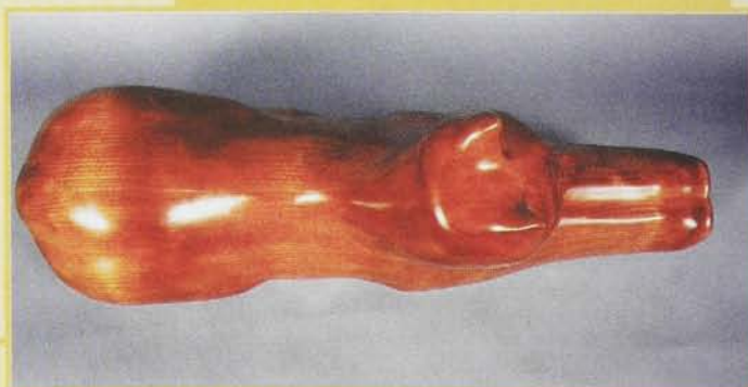
The shape of the cat emerged from the wood with the use of handtools such as macaroni tools and a drawknife.
