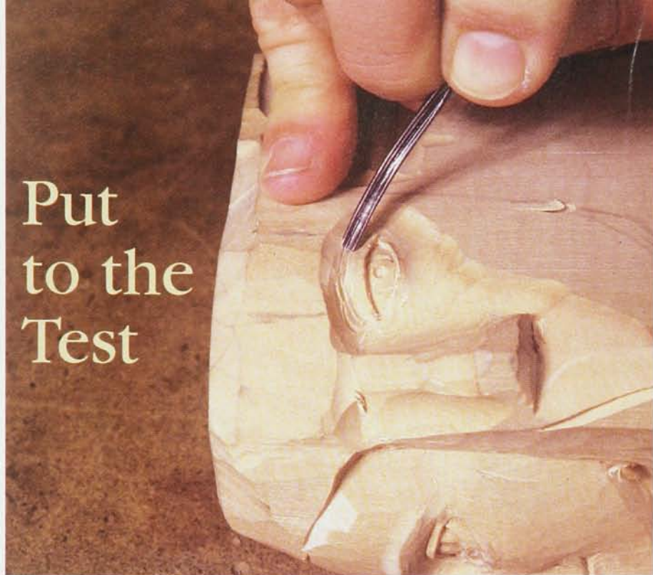
A 1.5mm short-bent V tool adds very fine age lines in the concave area above the eye of this carving.
