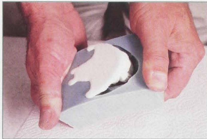
Follow the cure time recommendations before separating the mold and the cast. Remove ragged edges with a knife.
