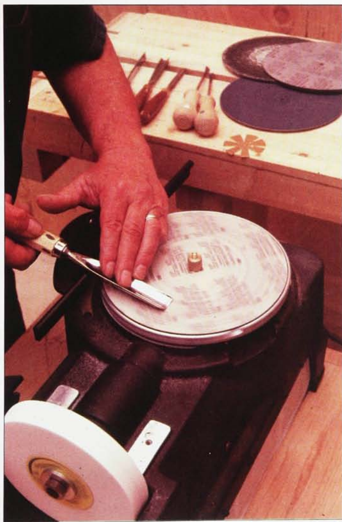
The Veritas Power Sharpening System consist of a horizontal platter to which abrasive disks are attached. Using no water, the abrasives can handle a variety of tools that include chisels, gouges and plane blades.
