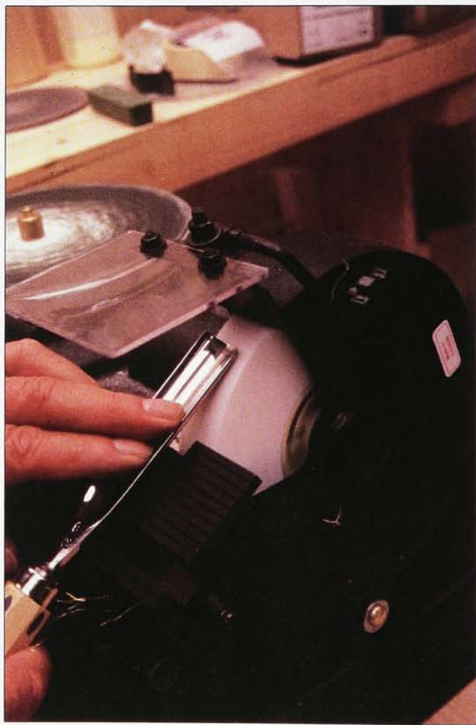
A 6-in.-diameter grinding wheel and an adjustable tool rest are excellent for both sharpening and re-shaping gouges. The soft wheel and slow speed greatly reduce the risk of overheating.
