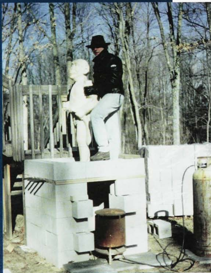
Joe Avarista's homemade kiln consisted of cinder blocks, propane tank, burner, and other materials.
