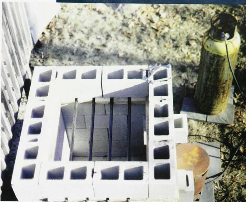
1-in.-diameter pipes supported the carving above the burner.
