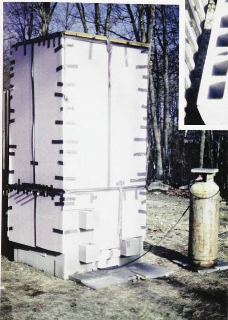
The kiln was enclosed with sheets of Styrofoam to reduce heat loss.
