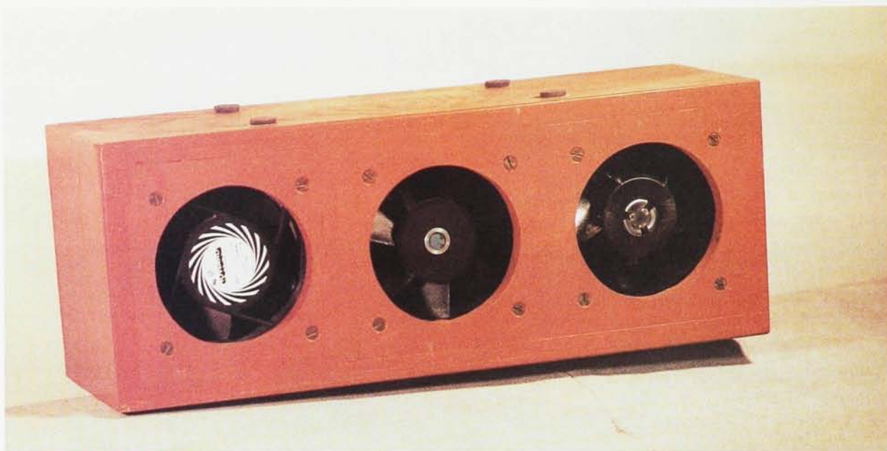
Rear of the dust collector.
