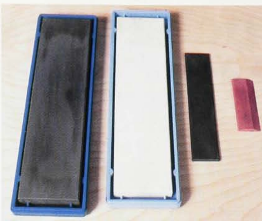
Man-made ceramic stones are extremely hard and retain their shape longer than most other stones. However, they do not come in a wide range of grits. Examples are, from left to right: medium, fine and two slip stones.
