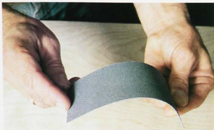
One form of diamond stone is flexible owing to its plastic backing. Pieces can be cut away with scissors and attached to wood or metal armatures for sharpening irregular shapes.
