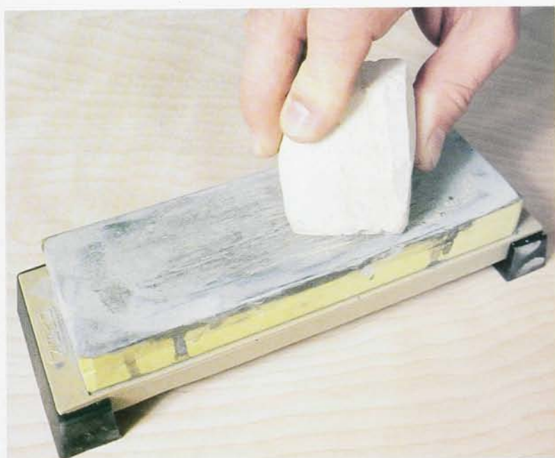
Japanese waterstones have grits that range from 100 to 8000. To create a sludge that helps with the sharpening process, a nagura stone is rubbed on a waterstone. The nagura stone creates a paste that saves sharpening time and encourages even wear on the waterstone.
