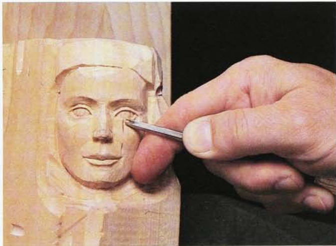
Small tools such as the no. 11 2mm veiner, useful for outlining eyes, are available from pfeil®.
