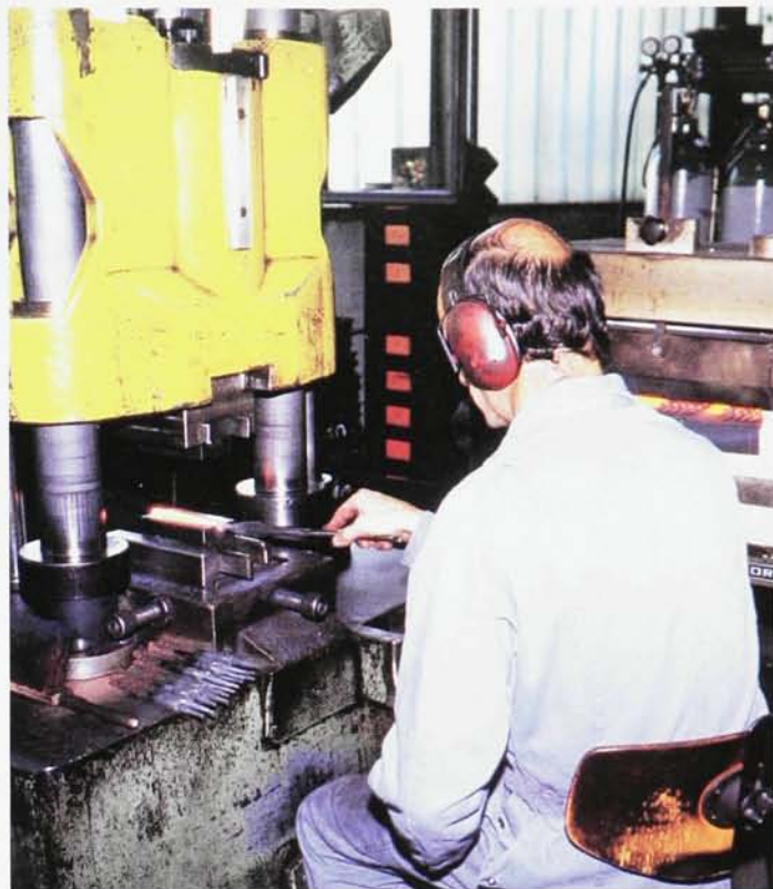
Pfeil® tools are manufactured in Switzerland where forging and shaping are done using chrome vanadium steel. Photo courtesy of Pfeil®.
