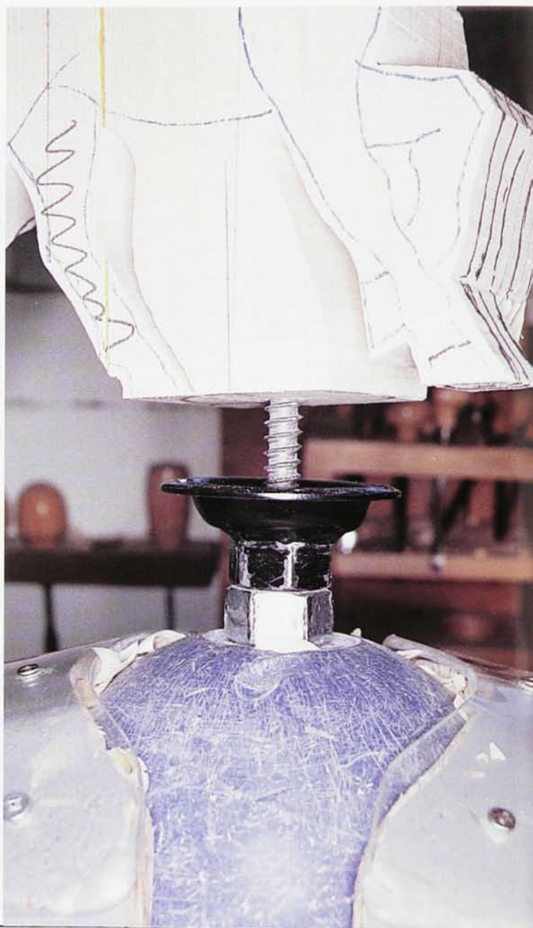
Bertsch uses a custom-made swivel vise to secure his horse carvings.
