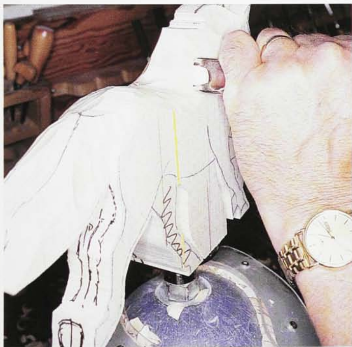
He uses a variety of gouges to rough out and finish-carve a horse, starting with a no. 9 and ending with a no. 3 gouge.
