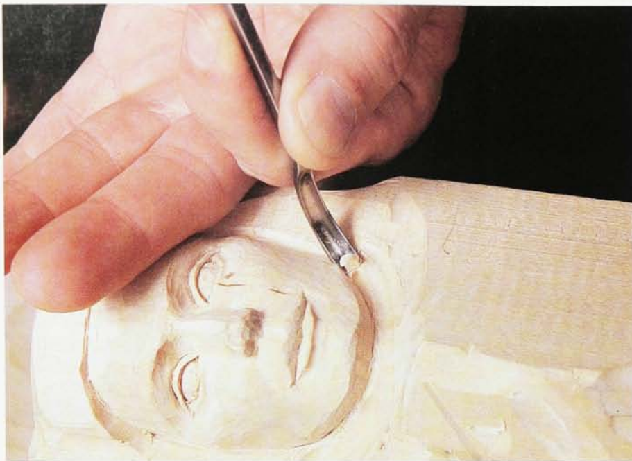
Manufactured by pfeil® are spoon-bent gouges such as the no. 9 7mm tool that I use to make concave cuts in high relief carving. They are also useful for undercutting areas not reachable with regular gouges.
