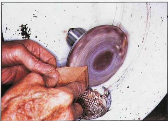
The cushioned disc effectively sands irregular shapes.
