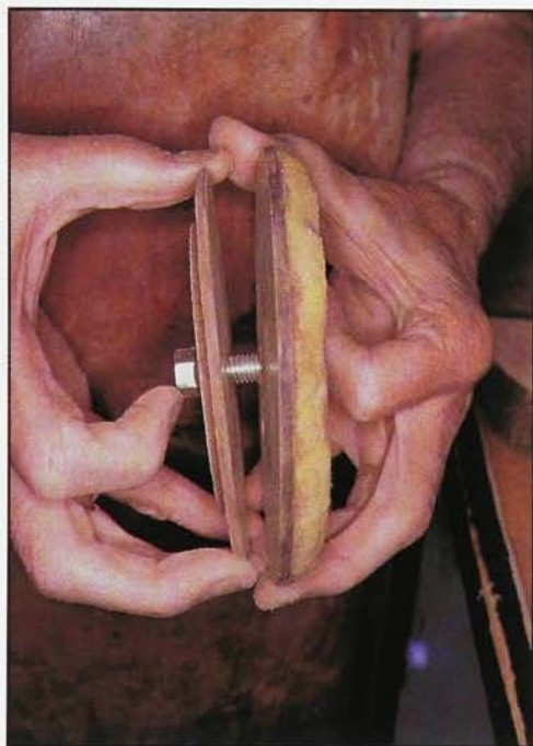
Finish-sanding is done with a custom-made sanding disc. It consists of pieces of Masonite, a piece of carpet padding, and a shaft.
