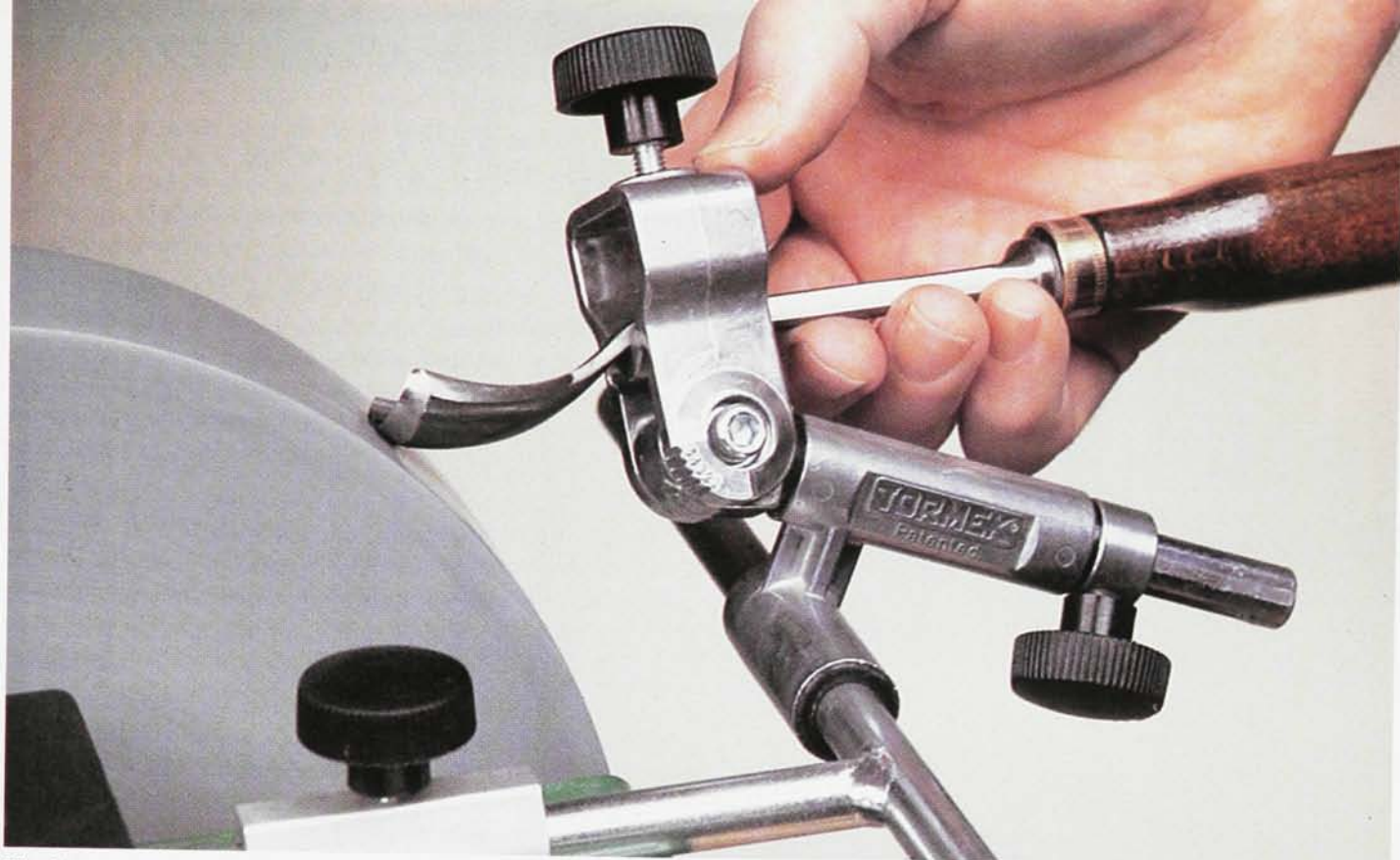
The Universal Gouge Jig SVD-180 is indispensable for sharpening gouges and V tools. The jig slides on the support bar for grinding away from the tool's edge.
