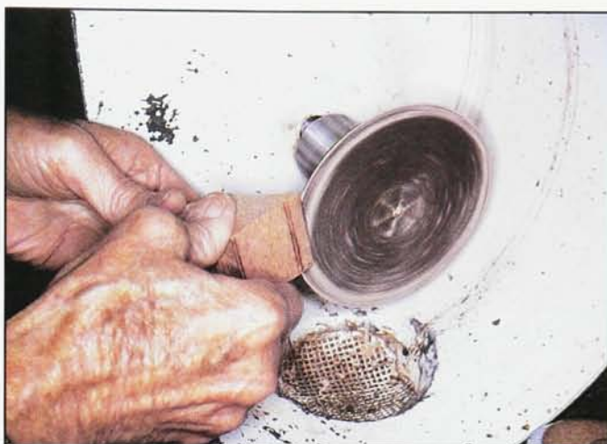
Shaping a pipe bowl is not done with grinders. Instead, Margroum uses coarse sandpaper glued to a rubber sanding disc to shape the bowl.
