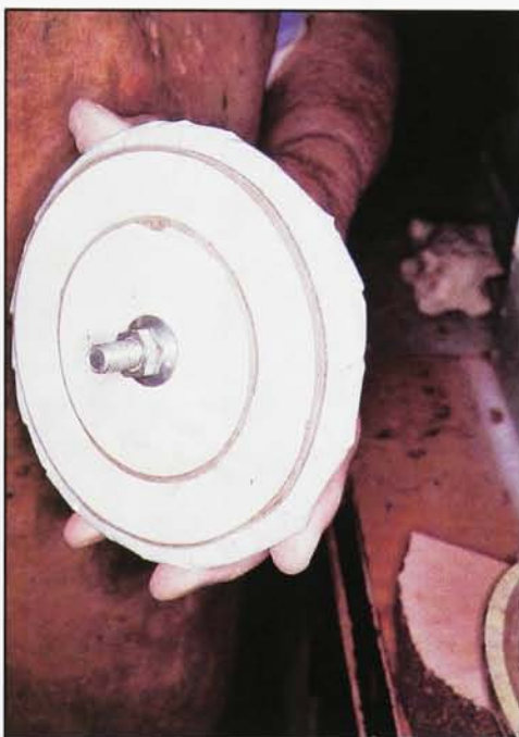
The padded sanding disc is covered with a pleated piece of sandpaper. The pleats are held in place between the Masonite plates.
