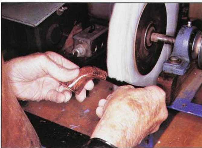
As a final step, Margroum polishes his pipes with carnauba wax applied to a homemade flannel buffing wheel.
