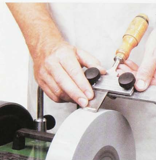
The Straight Edge Jig SVH-60 comes with the basic Tormek® system and is used for grinding and honing chisels.
