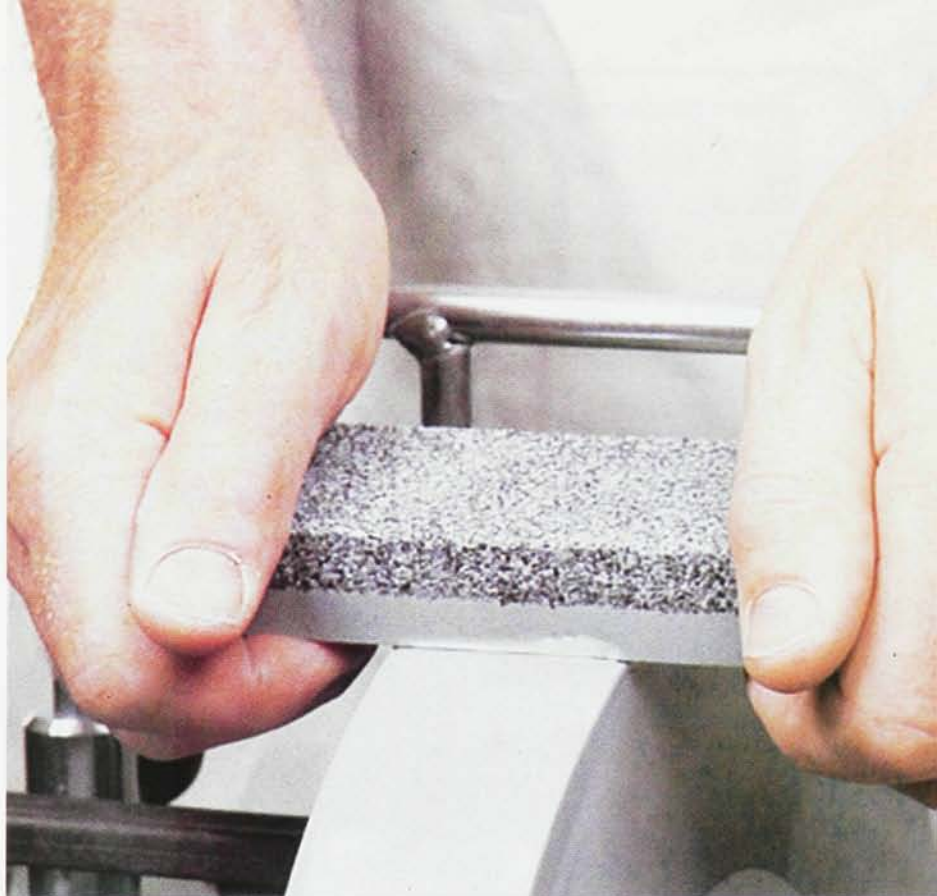
The Stone Grader SP-650 changes the grinding properties of the stone to achieve an extra-fine grind.
