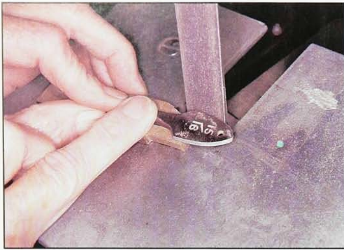
To bore out the pipe bowl, Margroum reshapes a spade bit using a belt sander.
