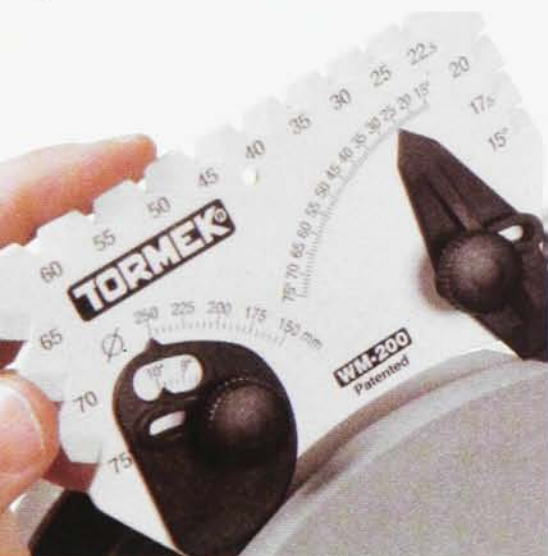
The Pro AngleMaster WM-200 helps set the edge angle on a tool.
