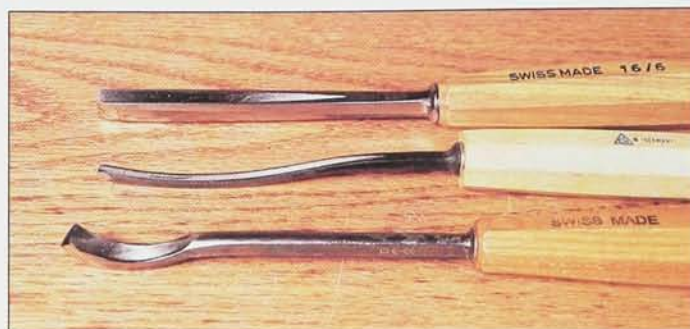
V tools come in a variety of shapes and sizes. From top to bottom: straight, long bent and short bent.
