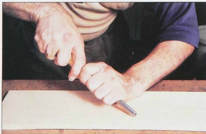
To properly hold a V tool, grip right above the ferrule and down the blade. Make sure that the heel of the gripping hand rests on the wood.
