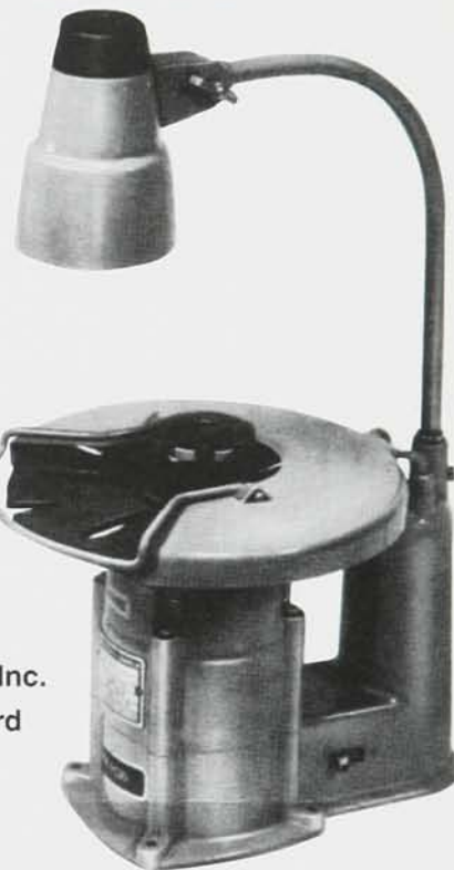
The perforated surface of the disc grinder becomes transparent with rapid rotation. The process of grinding a bevel on a tool can be clearly seen with the aid of a strong light source from above.
