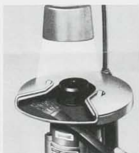
The perforated surface of the disc grinder becomes transparent with rapid rotation. The process of grinding a bevel on a tool can be clearly seen with the aid of a strong light source from above.
