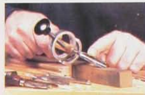
For sharpening gouges, V tools, chisels and skewers, I have developed a jig to maintain constant angles. The Oar Sharpener is shown here.
