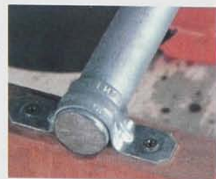
Grinder base and tool rest. Tool rest: 3/4 in. dia. mild steel rod. Base: Birch plywood, 24 x 9 x 1/4. Tool post: 5 x 3 x 1-1/4. Motor held to base with 2 1/4 x 3/8 flat-head machine screws. Locate mounting holes to match grinder base. Position the tool posts so there is 1/8-in. clearance between the grinding wheel and the tool rest.
