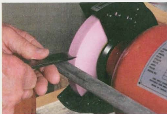
Straighten a damaged edge by grinding straight into the wheel. Press with your thumb to roll the tool on the rest.
