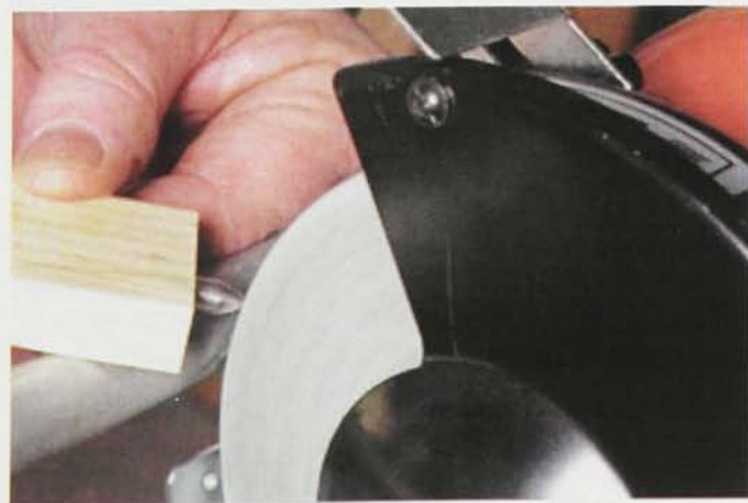
Shape a grinding wheel with a carborundum stick, (top) or with a diamond dresser (above). This dresser has been mounted in a hole drilled in the end of a wooden block.
