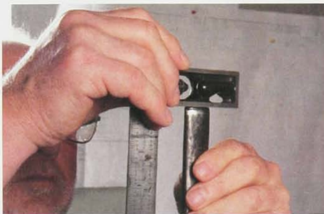
Use a square to check the edge of the gouge. It should be straight across.
