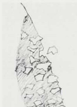
A soft bond permits the abrasive particles to break away, exposing fresh, sharp grit.
