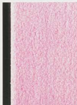
Wheel surface magnified 8 times shows the individual particles of abrasive grit.
