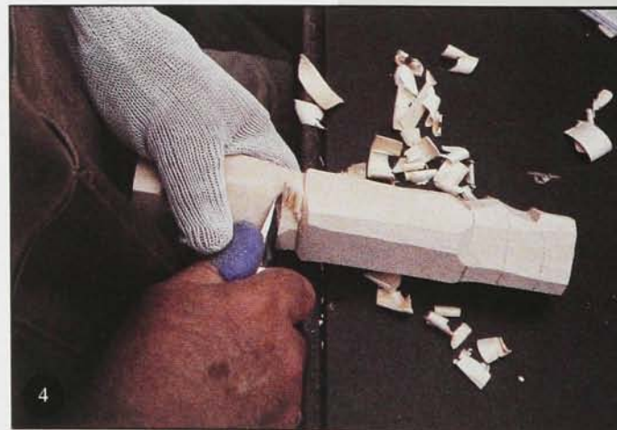
I get the body generally shaped using a leverage cut. With the knife held in one hand, I use the thumb of the opposite hand to push on the back of the blade. But I don't push the blade into the wood. Instead, I position the blade near its tip and, as I push the blade into the wood, I work it toward the base of the blade. It's what I call a skewing motion. I have both control and a mechanical advantage.
