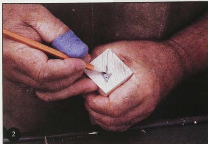
Grain direction has to be decided before carving. The arrow points to the front of the piece. With the grain running toward the front, I don't have to worry about breaking off the nose or the peak of the cap.
