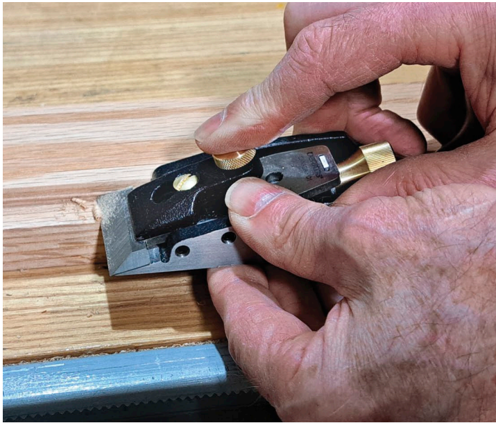
Clean Them Up – These planes can also be used to clean up a rabbet joint. Here, the Veritas Cabinetmaker's Trimming Plane is being used for that task.
