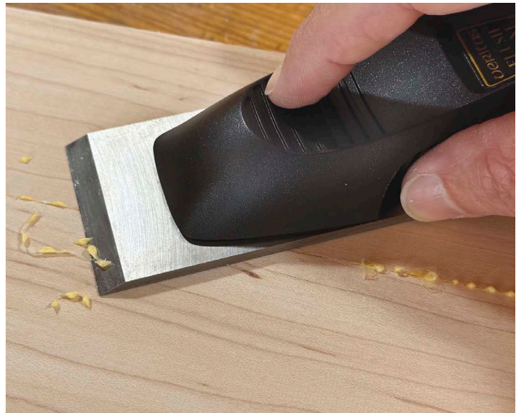
Squeeze-Out – A chisel or flush plane will do a good job removing partially or fully dried glue from a joint.
