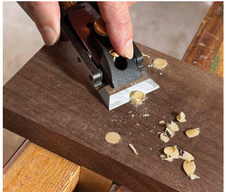
Flush Them Up – Trimming dowels or plugs is easy and accurate with a sharp chisel or flush plane. Here, the Veritas Cabinetmaker's Trimming Plane takes care of the task.
