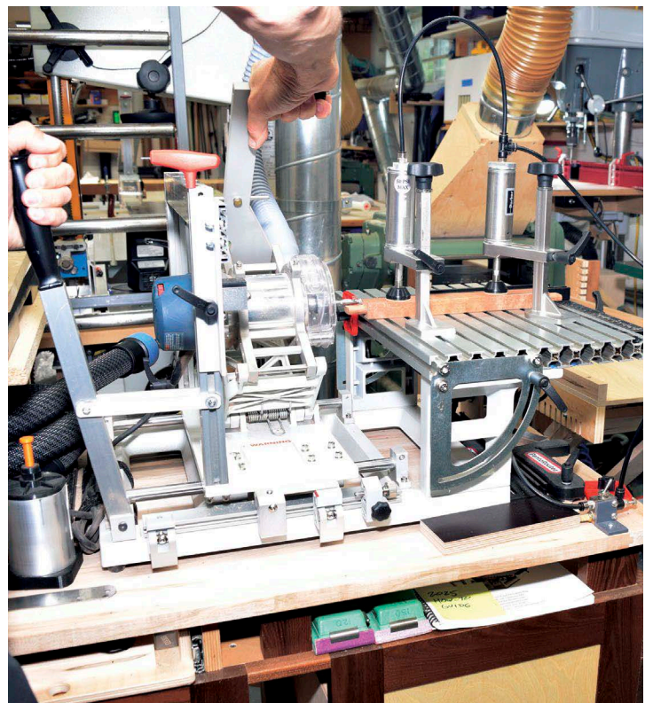
PantoRouter — A PantoRouter is a very flexible machine for making all sorts of joints. Here, David Bedrosian creates a tenon in his workshop. (Photo by David Bedrosian)
