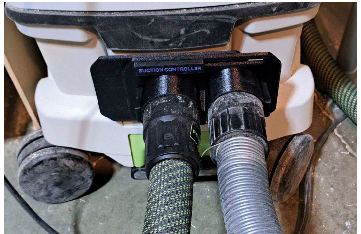
Quick Adjustment – When attached to a dust extractor, the switch between hoses, or even fine-tuning a ratio of suction between the two hoses, takes only a second or so.
