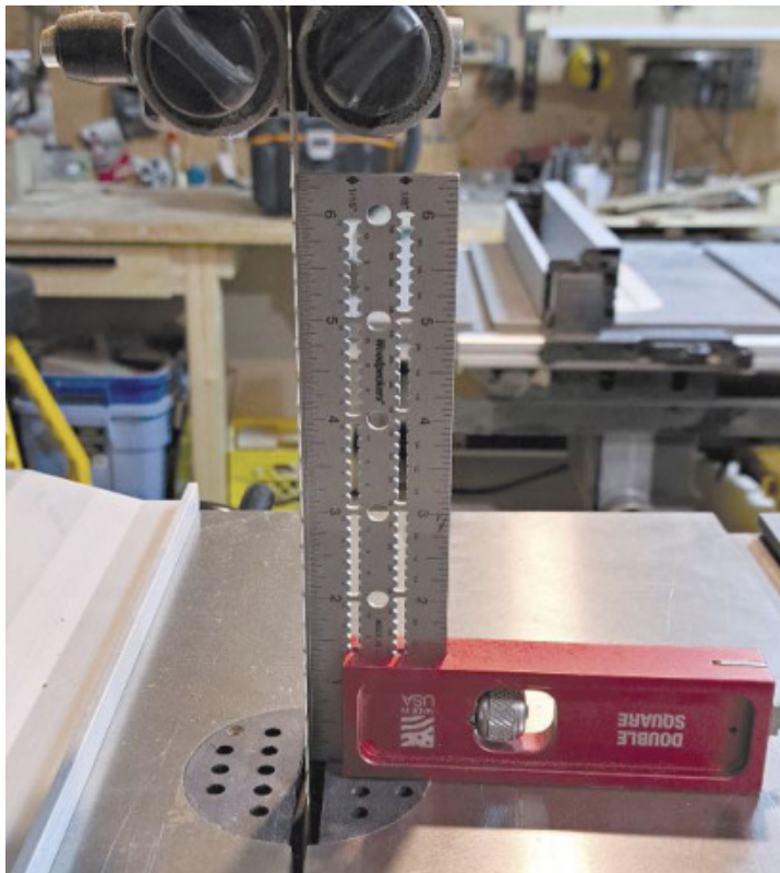
Sitting Square – Check that the blade and table are perpendicular to each other. Any adjustments can be made to the angle the table sits at.
