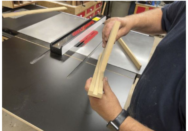
Nice Fit – Once the groove is cut in the end cap, it's ready to be attached to the main horizontal section of the jig for good.
