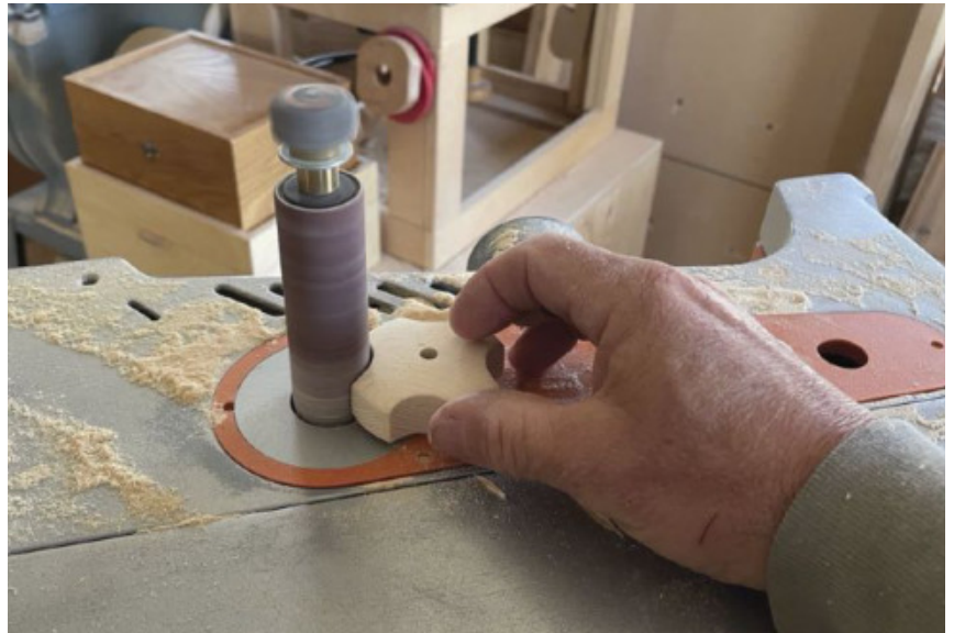
Shape the Notches – After removing most of the waste for the notches on the bandsaw, Harding uses a spindle sander to smooth the inner surfaces and create a unified look and feel.
