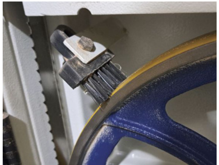
Tire Brush – A tire brush will keep sawdust and pitch from building up on the lower tire and, in turn, the blade.
