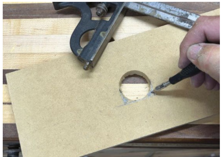
Create a Flat – Notching the hole so the clamp jaw can better seat against the flat edge works nicely.
