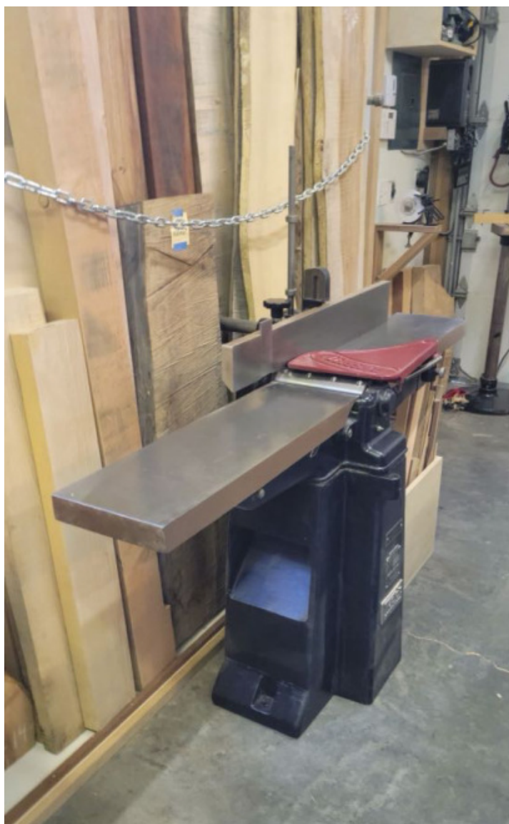
Starting Point – Selecting the right boards for a project is a critical step. Thornhill keeps his lumber standing vertically, secured with a chain. One of his jointers is nearby, ready to flatten one face and one edge of a board.
