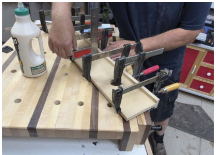
Clamp It Together – A bit of glue in the groove and clamps to bring the parts together are all that's needed.
