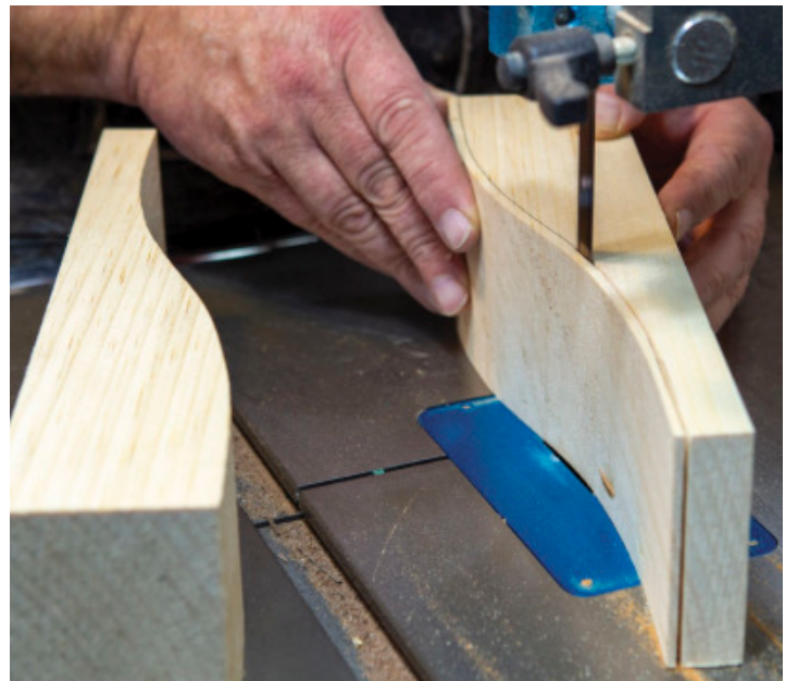
Remove Material – Once the lines are drawn on the blank, use a bandsaw to remove the same amount of waste as the laminations are thick.
