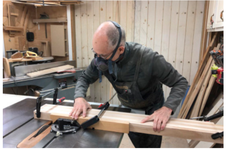
Nice Notches – With the legs ganged together, Brown cuts the notches in their rear edges to accept the plywood shelves.
