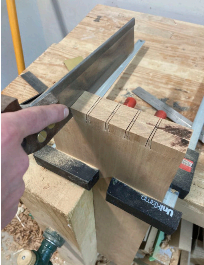
Gang Them Together – Dobson clamps two similar parts together before cutting the tails to speed up the process of creating the dovetail joints for the case.
