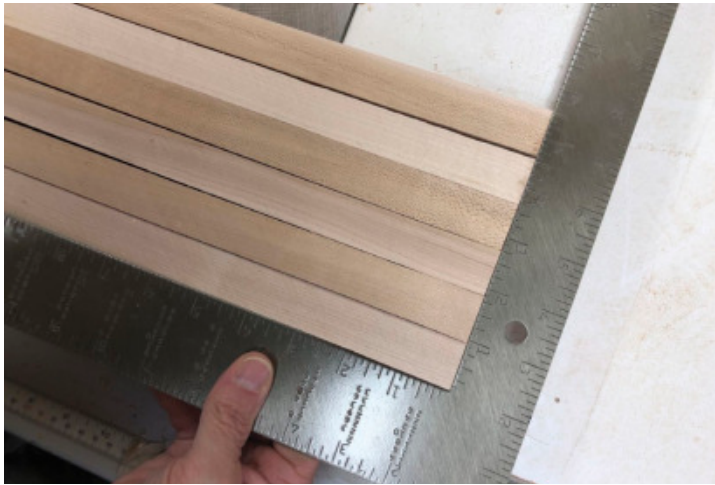
Square Up and Clamp – Brown ensures the legs are all aligned at their ends before clamping them together and machining the notches in them.
