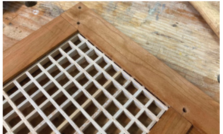
Drill for Pegs – Holes in the corner joints will accept pegs. The pegs will increase the strength of the frame, yet also play a role in aesthetics.
