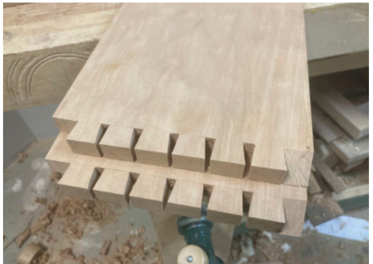
Ready for Assembly – These case parts can now be used to lay out the mating portion of the dovetail joints.
