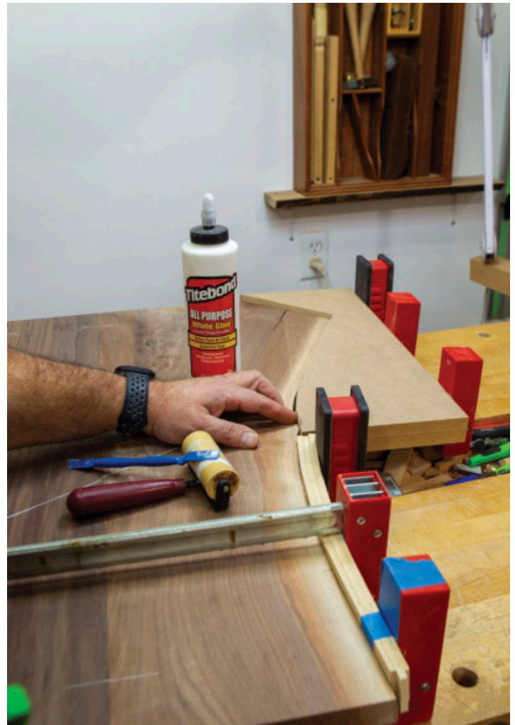
Cauls Are Critical – Cauls will spread clamping pressure over the width of the joint, but even more importantly, these cauls will help protect the live edge from being damaged by the clamps.
