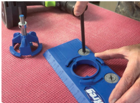
A Simple Twist – The main adjustment needed before using this jig is to set the hinge setback. With a twist of a screwdriver, it's easy to adjust the setback to between 3mm and 6mm. (Photo by Rob Brown)
