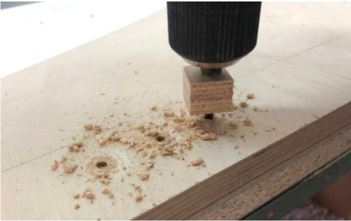
Not Too Deep – A simple wood stop over the drill bit will limit the depth of the hole so you don't drill through the other side of the workpiece. The depth of hole can be fine-tuned by adjusting the position of the bit in the drill's chuck.
