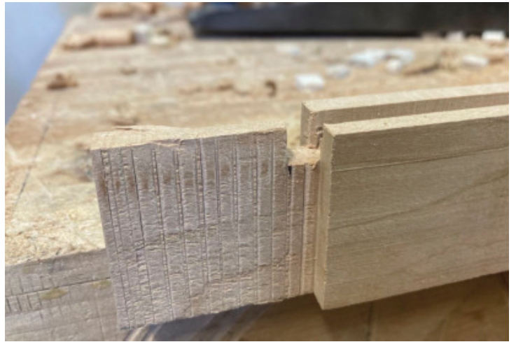
Notched Tenons – Once the tenons are machined on the table saw, a notch to accept the door panel needs to be cut into some of the tenons.
