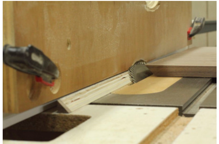
Simple Bevels – With the case pieces cut to length, Brown sets his table saw to machine the bevel joints on their ends and makes the cuts. The offcut sits in the ample gap between the fence and the blade once it's removed.
