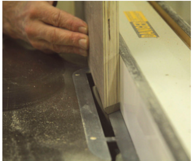
Flip the Fence – Brown moved the table saw's rip fence to the left side of the blade to make the first cut to shape the edge profile at the front of the case. If you have a left-tilt saw you can make this cut with the fence on the standard (right) side of the blade. This pass should be made first, so the flat portion of the front edge can reference off the table saw's upper surface.
