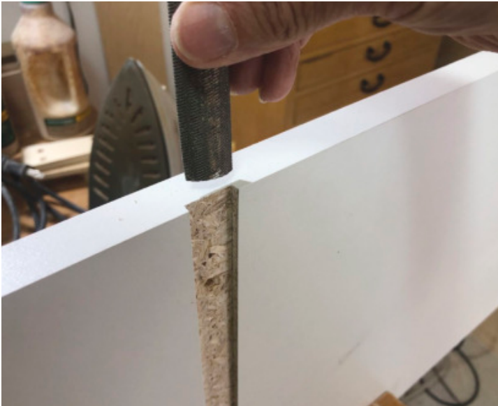
Tape, Then File – Once the iron-on tape has been applied to the exposed edges, Brown used a file to clean up the areas around the ends of the dado and rabbet joints.
