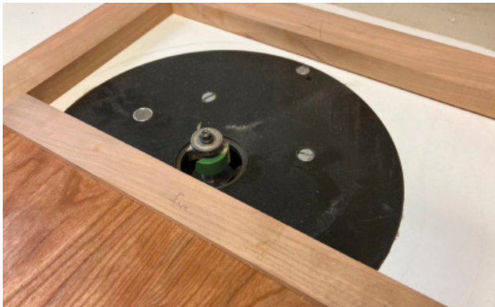
Rout a Rebate – Rout a rebate into the rear face of the door so the kumiko panel can be installed.
