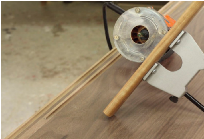
Groovin' – A trim router, edge guide and straight bit will make quick work of machining the grooves for the doors to slide in.
