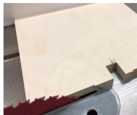
Choice Is Yours – Although it's not completely necessary, Brown chose to remove about 1/8" from most of the front edge of the template, but to leave the material near the notch. This gives the bearing on the router bit something to run on shortly before the bit starts to machine the wood.
