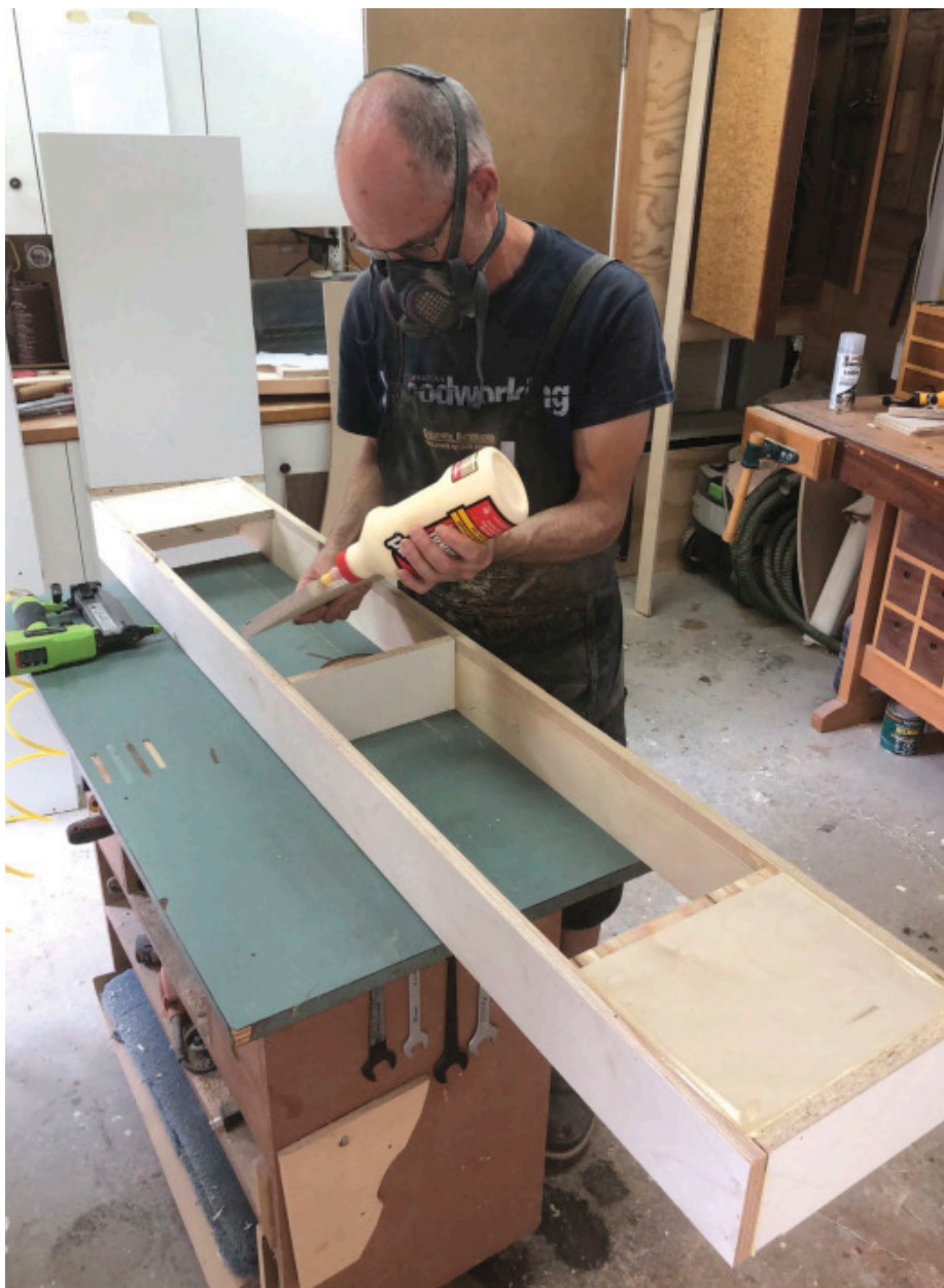
A Strong Base – A base that can be positioned in place, then shimmed to be level, will give you a solid foundation on which to build the rest of the wall unit.
