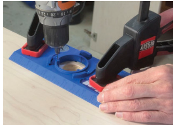
Two Easy Pilot Holes – Once the 35mm hinge hole has been bored, remove that bit and bore the two 1/16" pilot holes to attach the hinges. This helps keep the hinge plumb to the edge of the door and not split the material while installing the screws. (Photo by Rob Brown)
