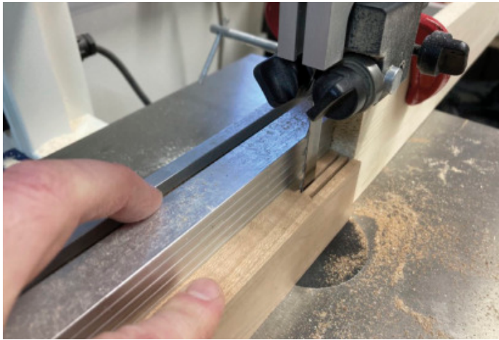
Start with the Slots – Dobson cuts the slots for the door joinery on the bandsaw.
