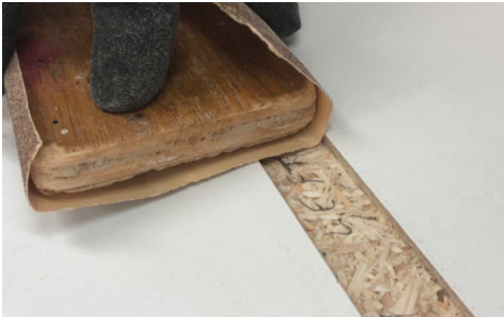
Reduce Chipping – During assembly, the edges of the dados will chip if they're not lightly eased. Doing this also reduces the risk of cutting your hands on these sharp edges. Notice the part label on the exposed particleboard, letting Brown know how the workpiece will be oriented in the final assembly.
