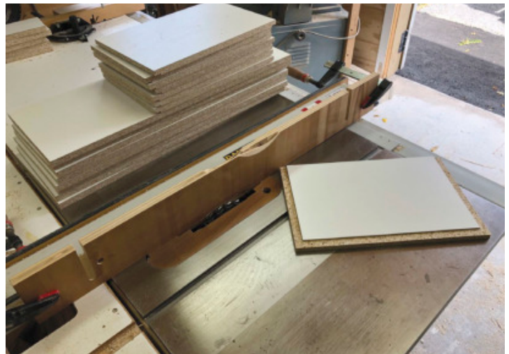
Drawer Parts – Simple rabbets and dados secure the drawer box parts together. Using the same material for the sides, fronts, backs and bottoms means only one setup is needed.
