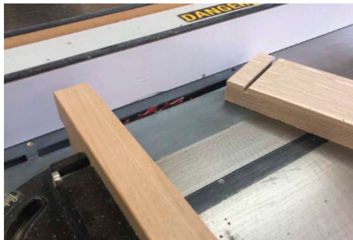
A Blade Kerf – A blade kerf is all that was needed in the horizontal support rails. Position one edge of the kerf so once the mating tenon is machined the rear faces of the two parts are flush.
