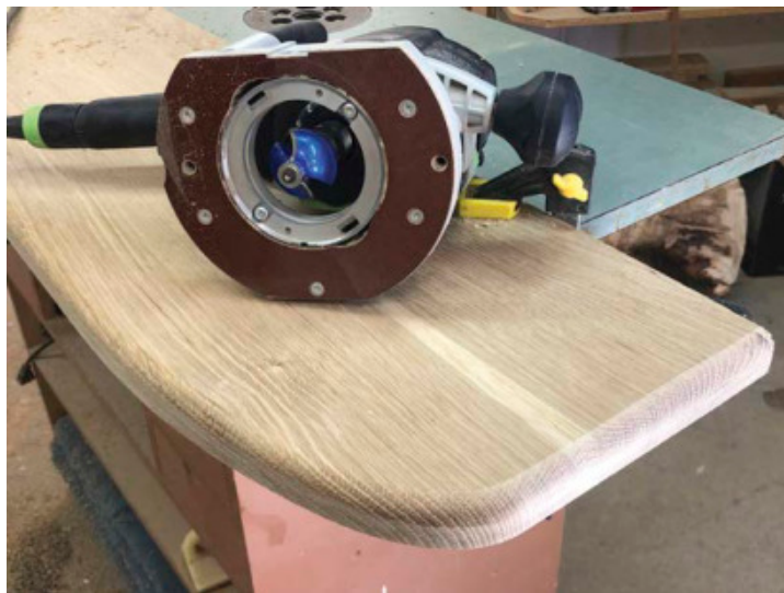
Ease the Edge – Brown routed a round over profile into the underside of the surface. He didn't rout the rear edge.
