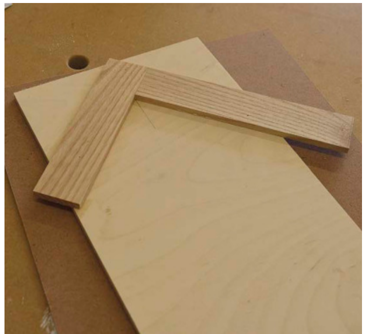
Right Angle – Ensure the first two pieces are accurately fixed to the base and at a 90° angle to each other. These two pieces will form the basis for the design.
