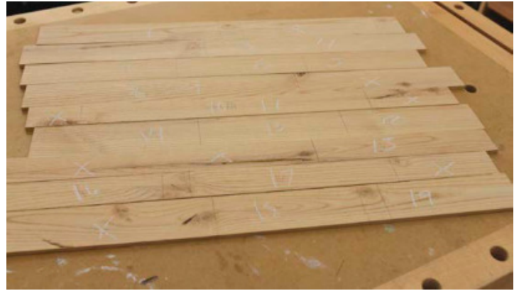
Knot Free – Nicholson marked all his solid wood strips so he could remove all the knots yet still have usable lengths of material for the sign face.
