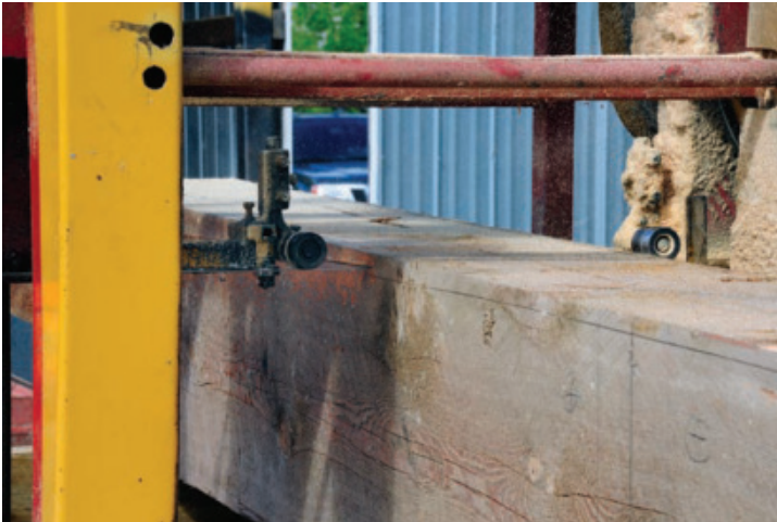
Rough Shape – The camber on the front faces of the gate rails are shaped on the Clarke bandsaw mill by sneaking up on the final shape. This is one of the first steps in making the gates
