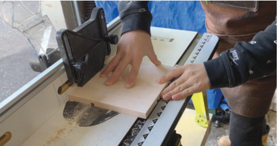
Cut the Grooves – A router table can be used to cut the epoxy grooves. You could also use a table saw. Just be extra careful when machining a small board. In that case you might want to leave the workpiece long and machine the grooves before cutting the blank to finished size.
