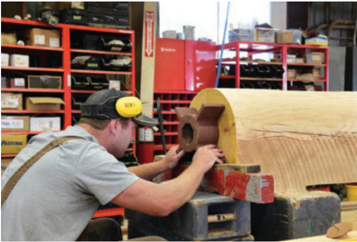
Wedges to Fine Tune Position – Wedges help the craftspeople align the gudgeon on the end of the quoin post before cutting the recessed area where it will fit into the quoin post.
