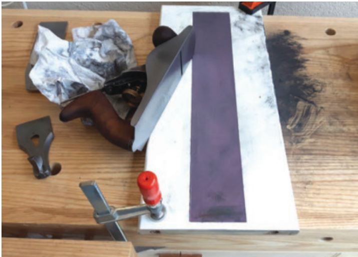
A Flat Sole – Flattening the sole, or at least at the toe, mouth and heel, is a critical part of improving an old plane’s performance.
