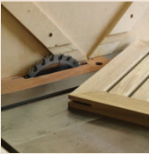
Cut the Grooves – With the workpiece sitting in the jig at a 45° angle to the surface of the table saw, the workpiece can be run across the blade to produce a groove for the solid wood key.
