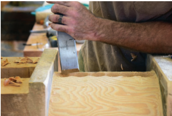
Square It Up – After removing most of the waste with a saw-toothed bit, the mortises to accept the wear bars are finished by hand with a chisel.
