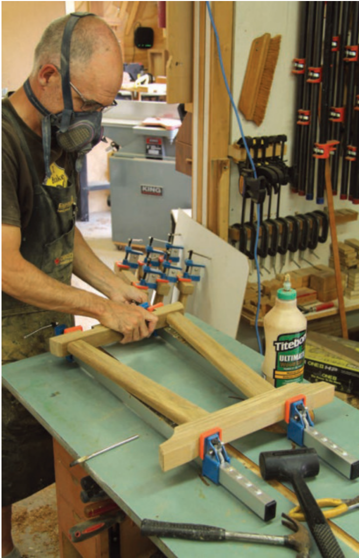
First Sub-Assembly – Bring the legs and upper / lower rails together with glue and clamps.
