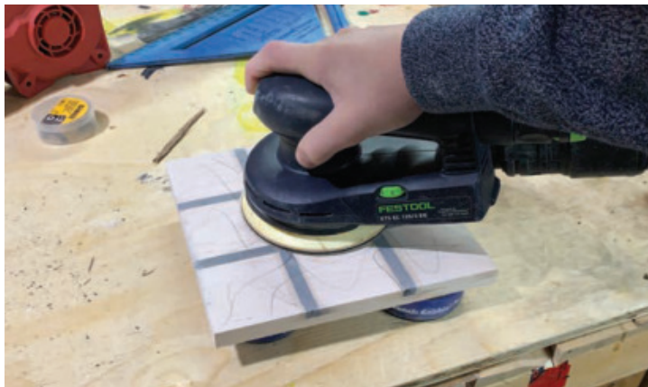
Sand It Smooth – When the epoxy has cured, sand the surface smooth.
