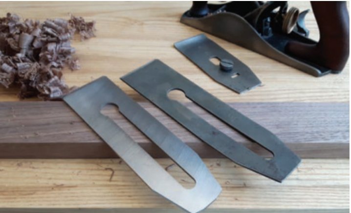
Blade Upgrade – Although you may very well be able to salvage the old blade and bring it back to life, a new blade (shown on the left) can also be purchased for just about every older hand plane out there.
