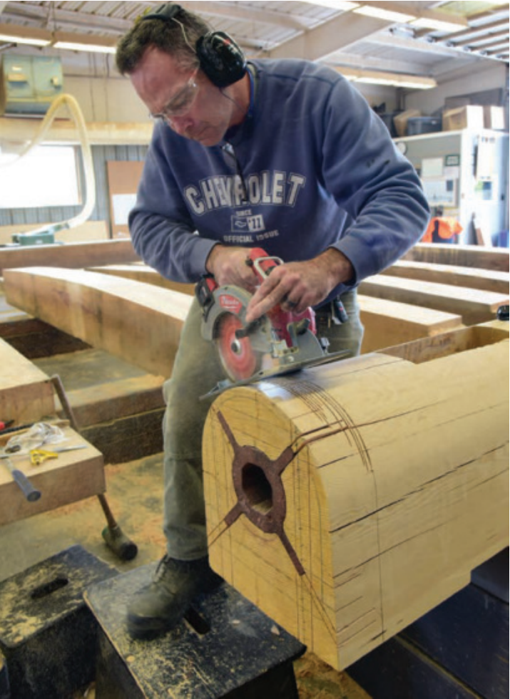
Wrapped in Steel – A circular saw is used to machine stop cuts into the end of the quoin post in preparation for placing the steel band around the perimeter of the end. This band will keep the end of the quoin post from splitting and weakening while it's in use.
