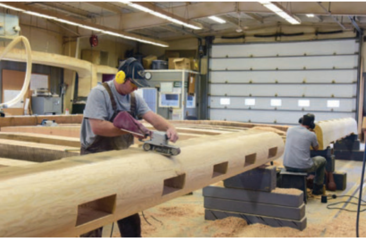
Correct Curvature – The curve on the edge of the quoin post needs to be consistent and accurate. Here, Joe Adams uses a belt sander to fine-tune the curved surface.
