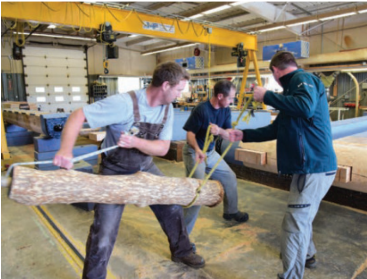
Bam-Bam – This shop-made tool – essentially a wooden battering ram – takes three men to use. It coerces all the large mortise and tenon joints to fit tight.
