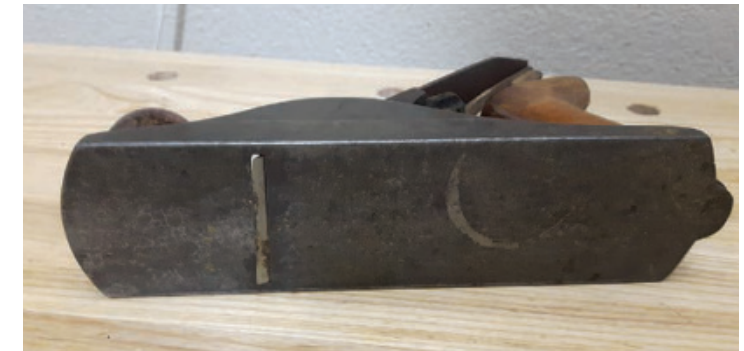
No Major Problems – A few stains aren't the end of the world. Deep pits or cracks, on the other hand, are harder to deal with. This is the underside of Duguay's plane before he set to work breathing new life into it.
