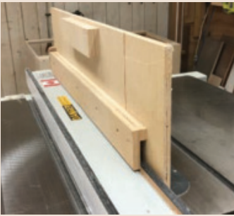
A Key Jig – A simple jig, consisting of the main plywood surface, a few pieces of material to guide the base on a table saw's rip fence and a pair of fences fixed to the base forming a 90° angle will assist in cutting the grooves to accept the keys.
