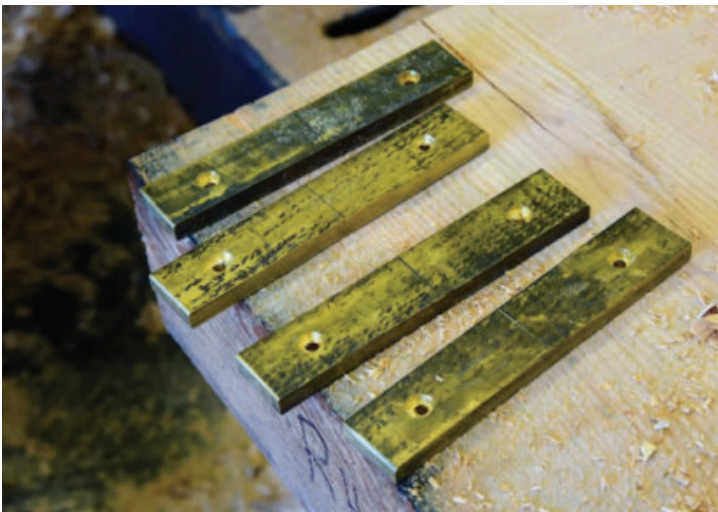
Wear Bars – Brass wear bars await insertion in the mortises cut into a quoin post.
