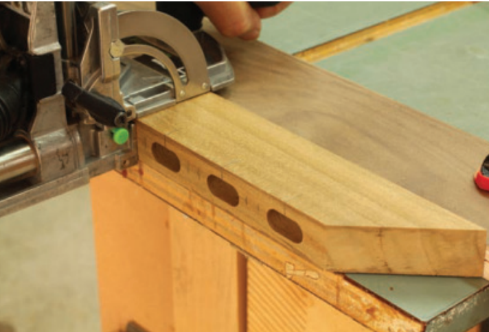
Mortises for the Slats – A Festool Domino makes quick work of the mortises, though a router can also be used. Even dowels would properly secure the slats to the mitred frame. Brown carefully marked each mortise with pencil.
