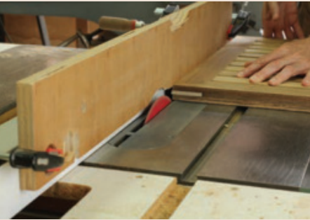
A Key Jig – A simple jig, consisting of the main plywood surface, a few pieces of material to guide the base on a table saw's rip fence and a pair of fences fixed to the base forming a 90° angle will assist in cutting the grooves to accept the keys.
