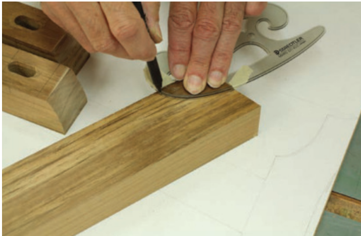
Notch the Top Rails – Notches in the upper surface of the top rails will accept the stringers.
