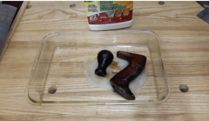
Remove the Old Finish – Paint and varnish remover will get rid of the old, cracked finish and leave you with a smooth surface on which to apply a new finish. This not only looks great, but it also provides you with a smooth, comfortable grip on your tools during use.
