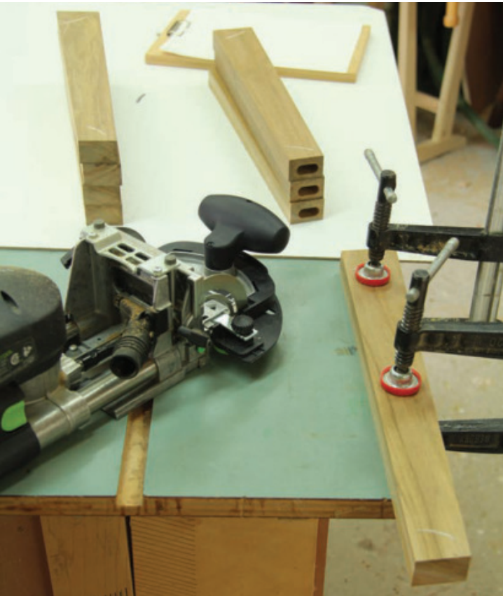
Time for Joints – Brown used his Festool Domino XL to machine the mortises in the legs and upper / lower rails, but there are many other ways to machine this joint.
