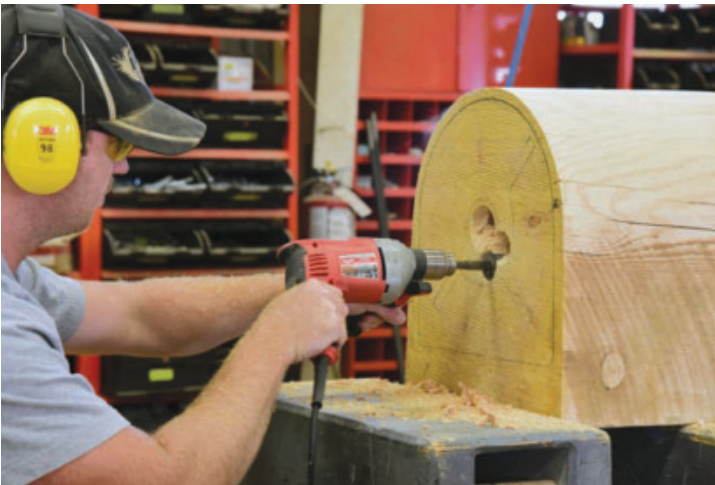
Drill Out Some Waste – Joe Adams begins clearing the waste to form the gudgeon mortise on one of the quoin posts with a saw-toothed drill bit.
