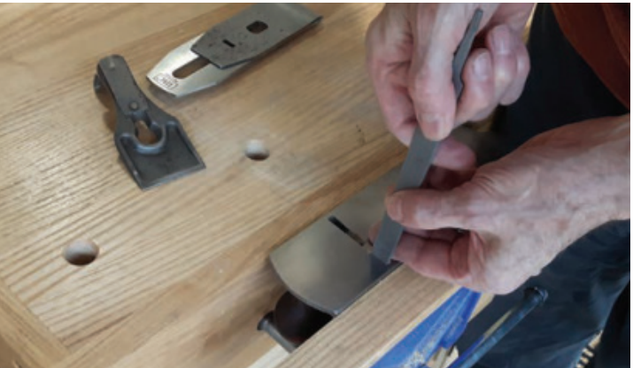
Widen the Mouth – Widening the mouth might be needed in order to allow the right amount of a gap between the blade and the sole of the plane.
