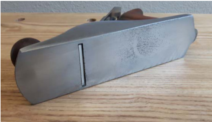
Refurbished Sole – Although the sole isn’t perfect, it doesn’t need to be. The odd stain or imperfection can be overlooked. Note Duguay spent some time on the sides of the plane to allow the plane to be used with a shooting board.
