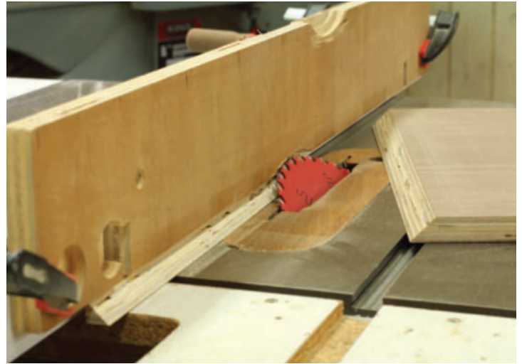
Cutting Bevels – There are a number of ways to cut bevel joints in case parts. Brown's approach allowed all the bevel joints to be cut after one setup. See "Online Info" at the end of this article for where to find information on this setup.
