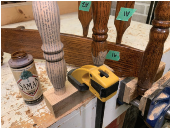
Simple Finishing Jig – A simple jig to hold the parts while finishing is easy to make.
