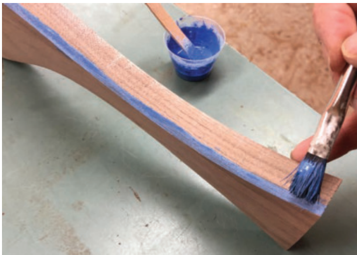
Paint the Visible Edge – The portion of the curved edge that will be visible once the curved sections are glued back together gets painted now. If you add paint to the entire edge, the glue will not adhere properly and the parts will likely come apart down the road.
