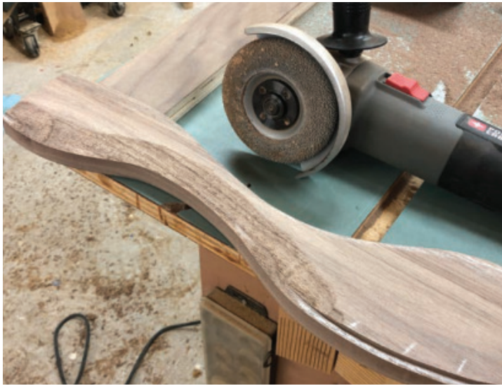
Smooth the Transition – Brown power carved the curved sections to slope down to the routed rabbet, but hand tools and sanders would also work.
