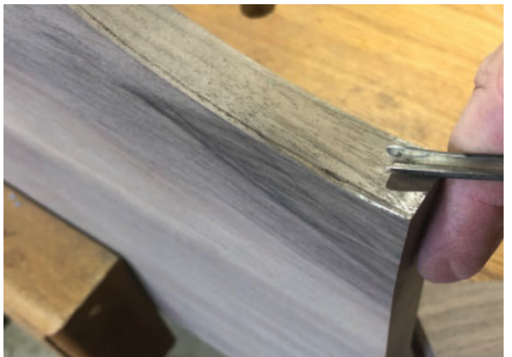
Small V-Groove – This edge will get glued to another edge that has had its outer 1/4" painted. To stop the glue from squeezing out, Brown added a small V-groove on its edge, close to the face of the doors, to capture any glue before it made a mess on the visible surface of the doors.
