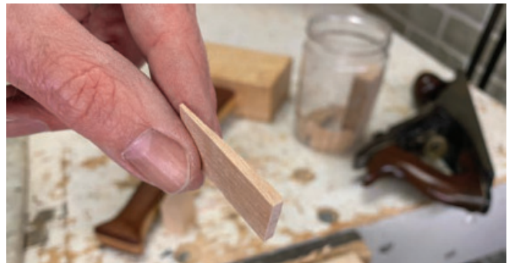
Make Some Wedges – A wedge helps secure the through tenons on the end of the posts. It's driven into the end grain of the posts once they're seated properly in the mortises.
