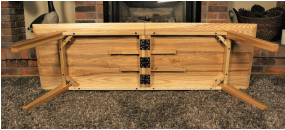
The Inner Workings – Once the hinges have been installed and the wedges have been pressed into place, the table can be flipped upright and used.
