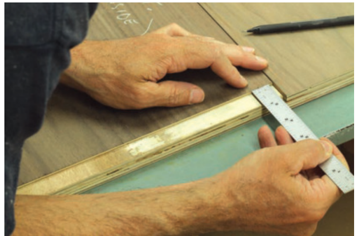
Dealing With the Scribe – With the bevel joints cut, Brown turns his attention to the rabbit joints that secure the rest of the case. Here, he has the case bottom and top aligned with each other and is marking the location of the edge of the rabbit joint in the top, as extra material needs to be left on the top to form the scribe.
