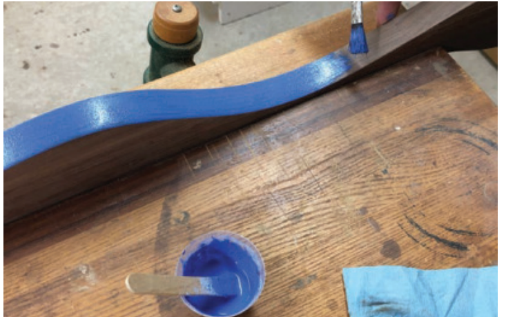
Add Some Paint – Here, the door edges in the gap are painted.
