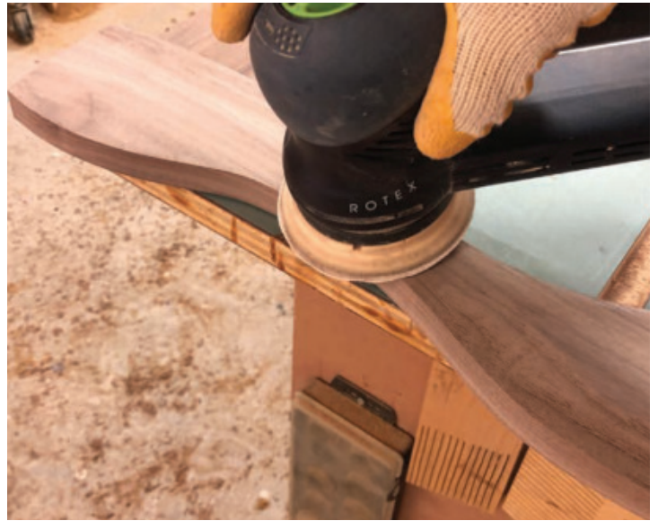
Sand the Curved Surfaces – A power sander will make quick work of the sloped surfaces. They need to be sanded so they're ready for a finish before the curved sections are glued back together.
