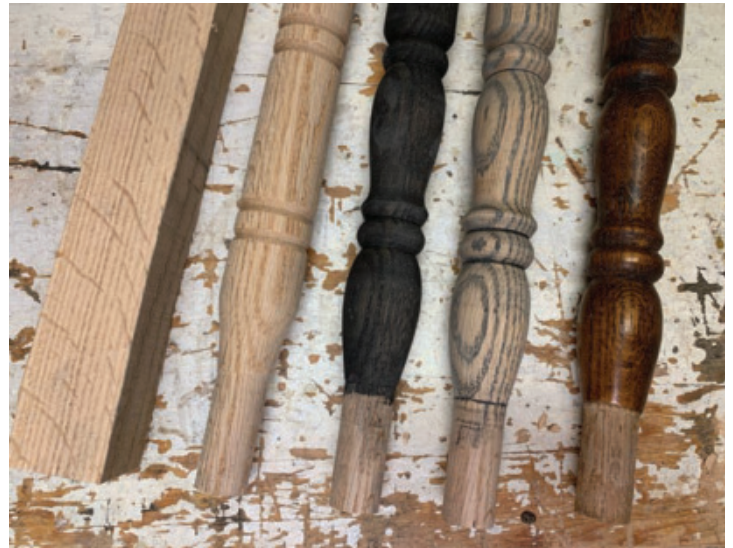
Different Stages – Here are the different stages of the posts as they get completed, from left to right: a rough blank; a partially turned post; the turned post with black paint; the paint mostly sanded off; and the post ready for final assembly.
