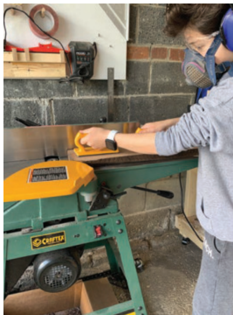
Mill It Flat – A jointer is a great way to flatten one face of a piece of rough lumber before planing it to thickness and machining further joinery.
