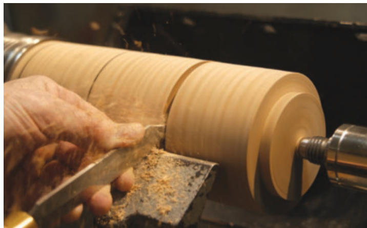
Cut the Top Off – Here, Cusworth parts off the lidded section and sets it aside while he focuses on the main cup and base sections.
