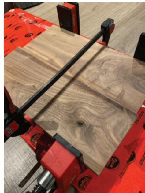
Glue Up the Top – With the boards that make up the top milled to rough size, glue and clamp the edges together and let the assembly dry overnight.
