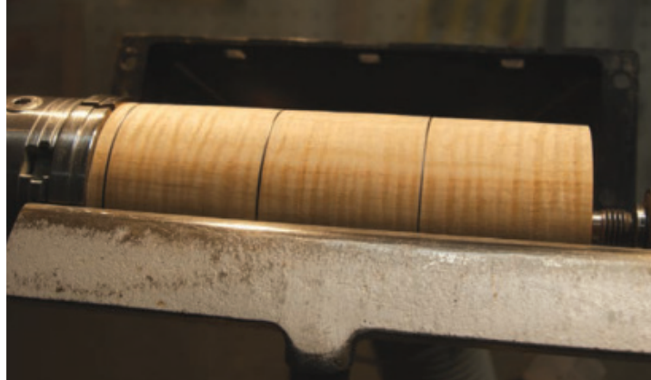
Divide It Up – With the stock turned round, Cusworth marked where the three main segments would be located.
