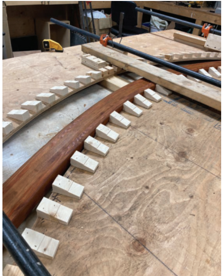
Pre-Bend the Strips – In order to make the bending process go more smoothly, the laminations are clamped up in the form long enough to "pre-curve" them slightly. This stops the laminations from fighting against you when the epoxy is applied to the strips.
