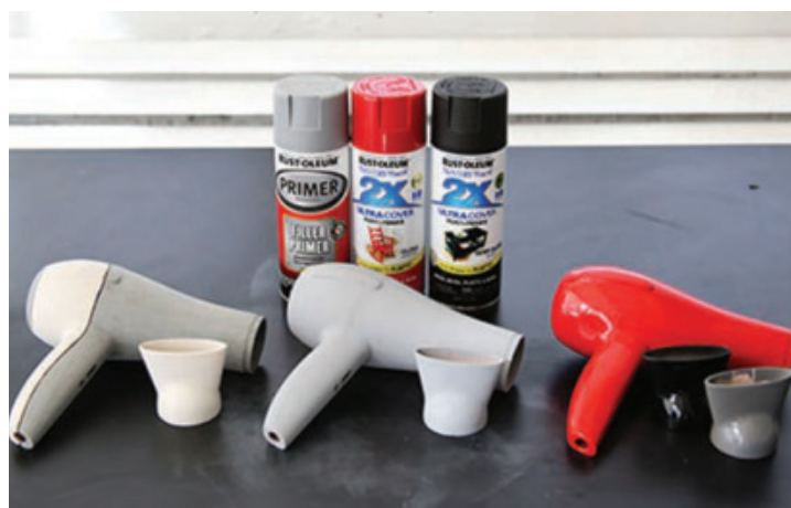
Post Print Finishing – A completed 3D print can be left as is or can be sanded, primed and painted to improve surface quality. (Photo by Makerbot).
