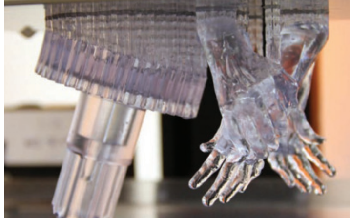
A Resin Printer in Action – A resin printer prints objects upside down, and they appear to “emerge” from the resin. (Photo care of Envisiontec)
