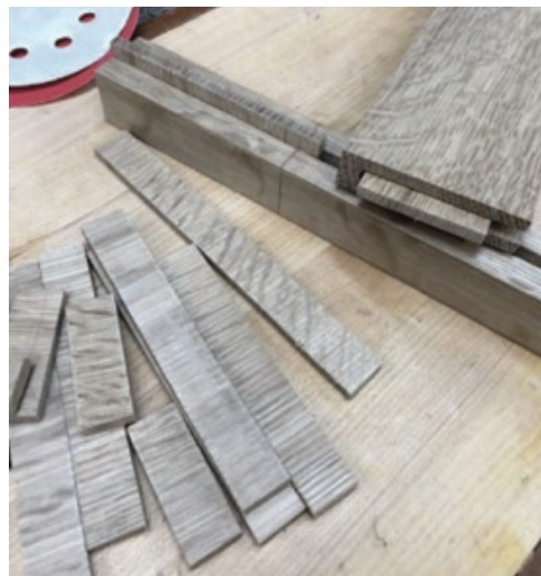
Floating Tenons – When making floating tenons it's critical the grain is oriented correctly or the joints will be very weak. Notice how the grain of the tenon that's inserted in the rail is running parallel with the grain of the rail.
