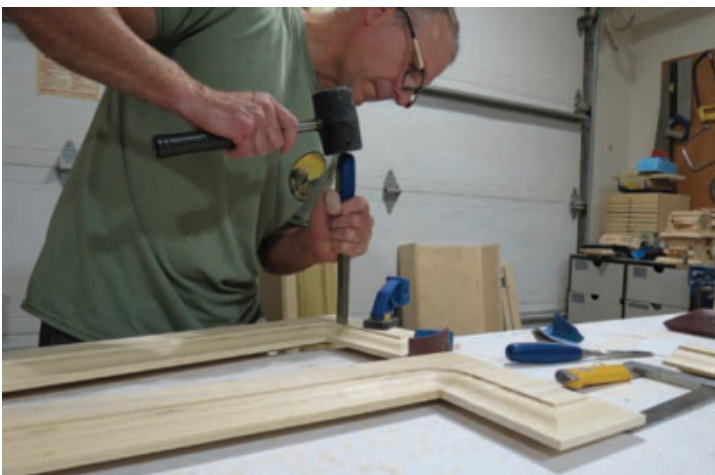
More Light Taps – A sharp chisel is mandatory for this step. After that, more light taps always trump fewer heavy taps with your mallet.
