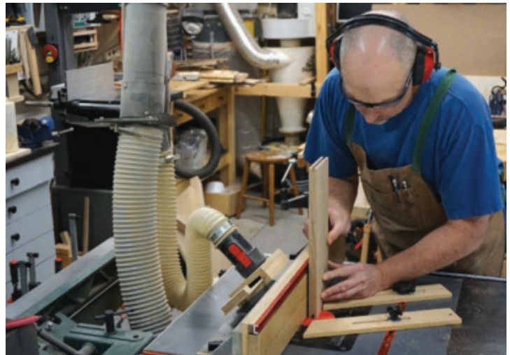
Lots of Grooves – Because Gillard used floating tenons to join many of the workpieces, grooves must be machined in the edges and ends of the stiles and rails.
