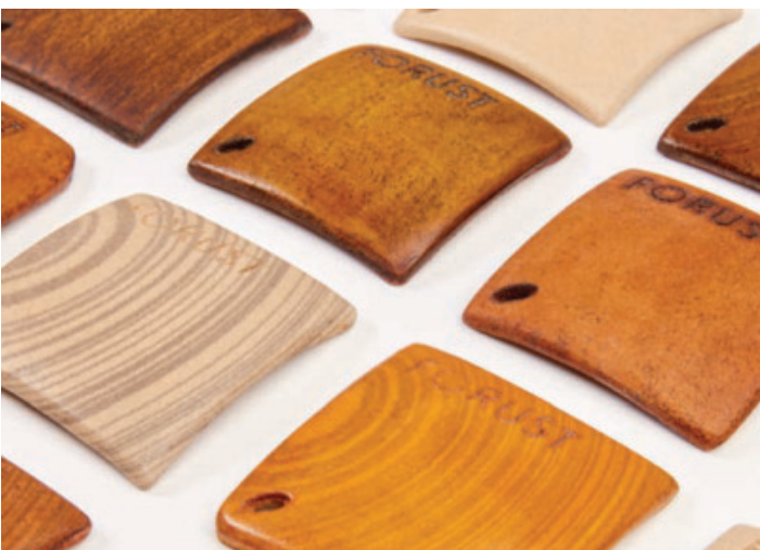
New 3D Printing Wood Technologies – 3D printing technology has advanced to include the ability to print wood products and reproduce wood grain. (Photo from Forust/Desktop Metal)
