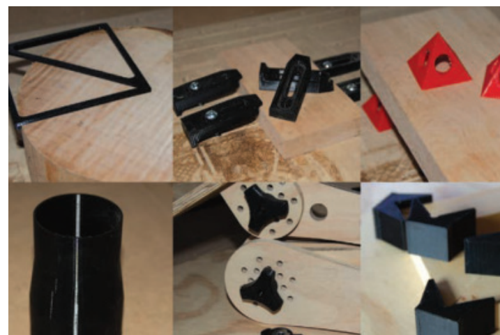
3D Printed Parts – Clockwise from top left: center finding jig; hold down clamps; finishing standoffs; corner clamp brackets; 1/4" -20 knobs; and vacuum adapter for a dust port.
