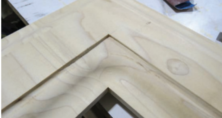
Squared Off – The finished inside joint, ready to be sanded and assembled.
