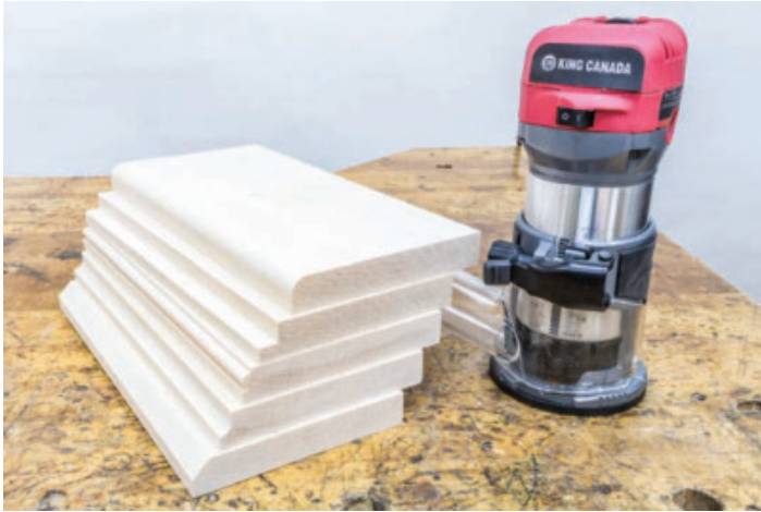
A Plethora of Profiles – From roundovers to rabbets and coves to chamfers, this King trim router has what it takes to rout all sorts of edge profiles.
