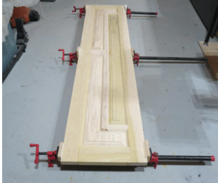
Final Assembly – After a dry fitting and sanding, it's time for some glue and clamps. Ensure the assembly is sitting flat while it dries.
