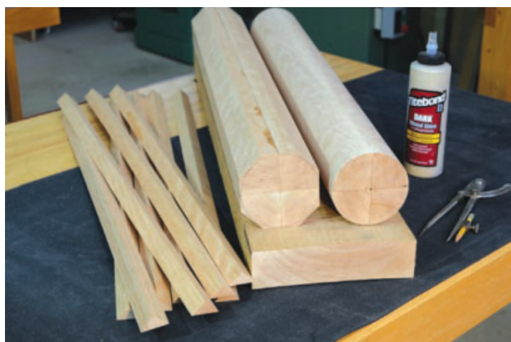
Waste Not, Want Not – Before the blank can be turned, rip each corner off and save the offcut. The offcuts can be used down the road to strengthen the leg-to-gable joint.
