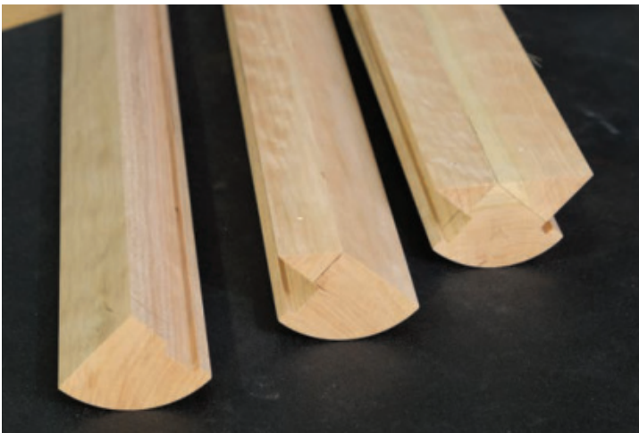
Different Legs – At left, a front leg with a freshly machined groove to accept the gable. Center, a front leg with the 45° ripping attached to it. Far right shows a rear leg with two 45° rippings glued to it.
