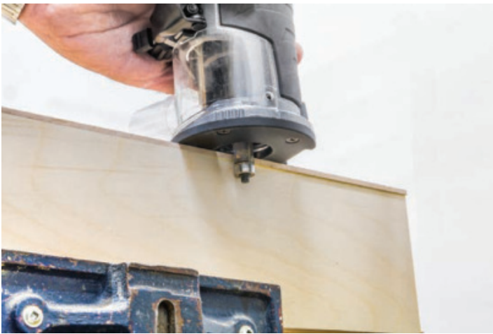
Flush It Up – On edge, the King trim router and fixed base make quick work of flushing up solid wood edging.
