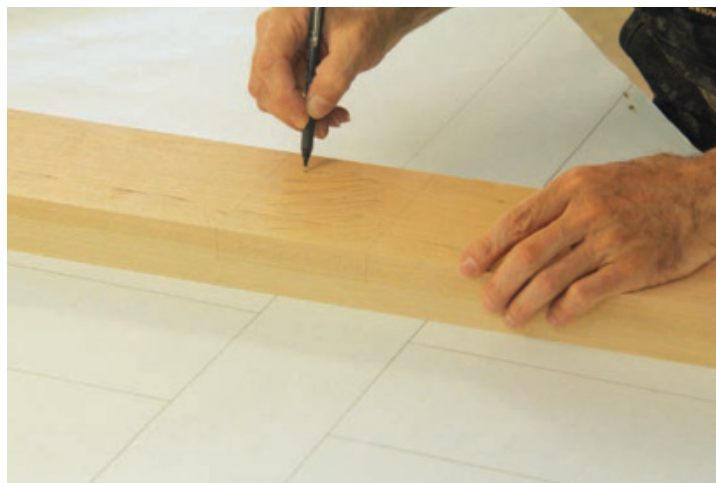
Full-Sized Drawing – When dealing with angles it's easier to have a full-size drawing to work toward. Here, Brown marks the half lap locations on one of the cross pieces and clearly marks the waste portion of the joint.
