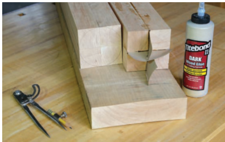
A Few Pieces of Paper – Salusbury machined the four corner legs square, then glued them in a blank for turning with craft paper between their seams. This keeps them together while on the lathe, but makes them easy to get apart afterwards.
