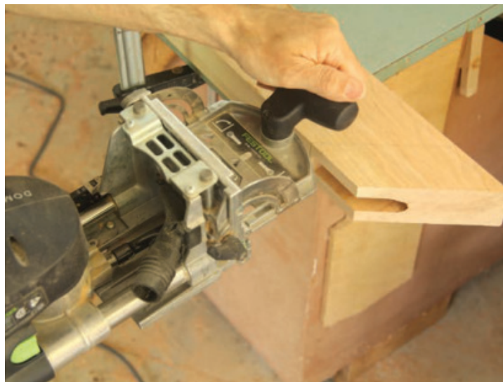
Dominos to the Rescue – There are many ways to cut this joint, but a Domino machine is one of the quickest. The remaining waste on the upper end of the cross pieces will be removed with a hand saw and chisel.
