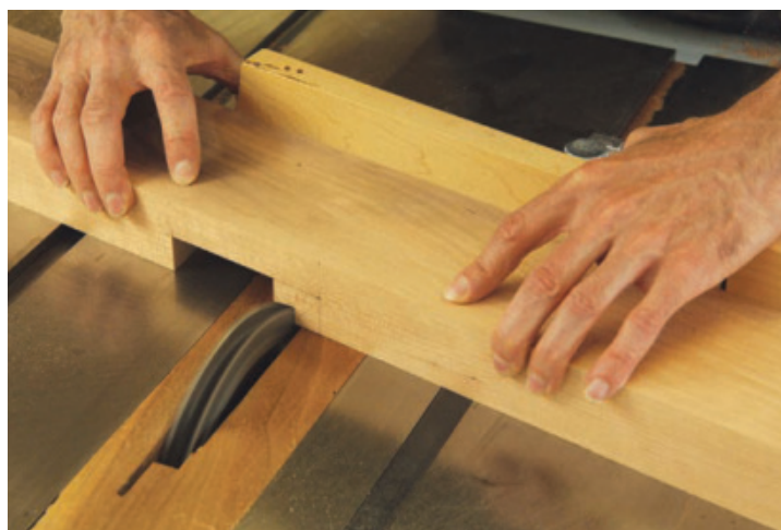
Remove the Waste – A dado blade removes wood quickly, but a standard width blade will also get the job done. Just be sure not to remove too much material or the resulting half lap joint will have gaps.
