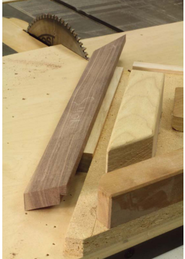
At an Angle – A strip of wood needs to be cut to the right size and attached to your miter sled securely in order to support the workpieces at a 20° angle while they're being mitered. Brown sized the strip to fit into the rabbet in each piece.
