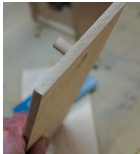
Flush on the Backside – When the locking knob assembly is pulled forward the larger portion of the shaft fits into the recess bored into the back of the sliding door. This allows the door to slide past the front edge of the top.
