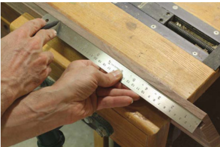
Mark the Length – The frame parts will have to be marked carefully, then cut to length. Keep in mind the size of the artwork the frame will house, and the fact that the artwork will fit into the rabbets surrounding the inner edge of the frame.
