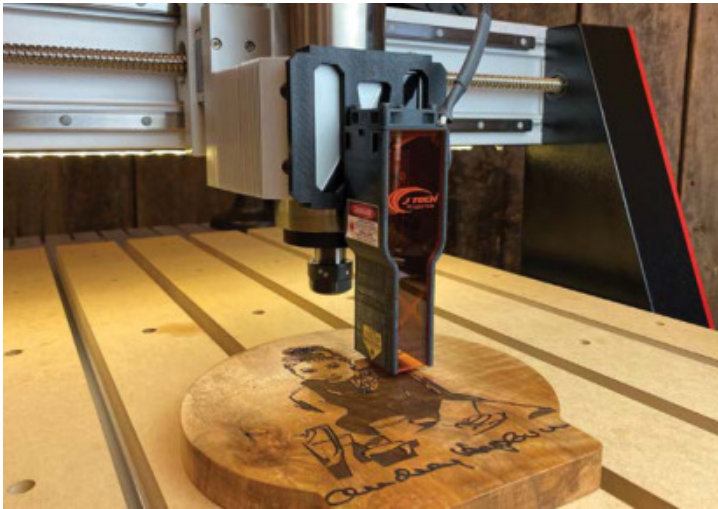
DIY Laser Add-On Package for a CNC Machine – Lasers can also be purchased as DIY kits from a variety of online retailers, then added to a CNC machine. (Photo by AxiomPrecision.ca)
