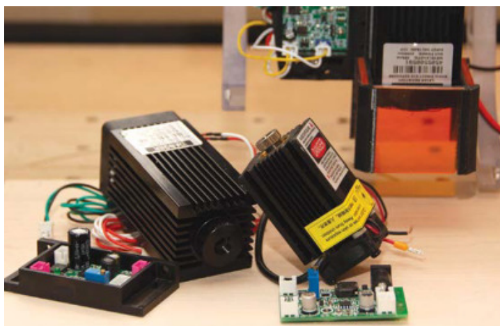
Common CNC Accessories – Lasers are a common accessory purchased for CNC machines. Shown here is the Jtech laser accessory for Axiom CNC machines. (Photo by AxiomPrecision.ca)
