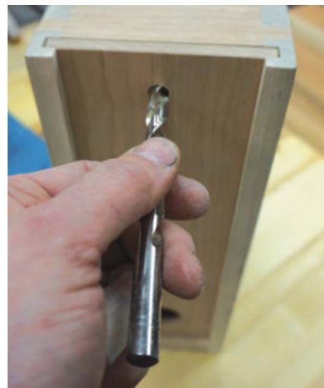
Brad Point Bit to the Rescue – A Brad point bit will allow you to mark the location of the 1/2" diameter hole in the locking knob strip. With the sliding door closed, press the bit through the hole and press the tip to mark the hole.
