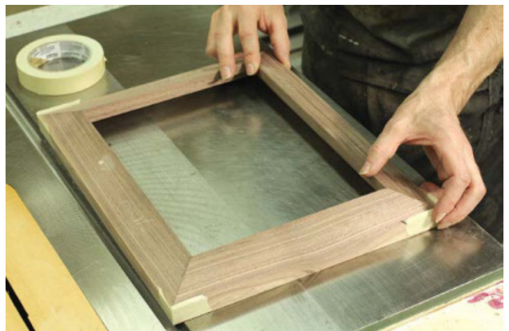
Test It Out – After using masking tape to hold the first three corners tight, Brown wraps the four frame pieces together and tapes the final corner. If any gaps are showing, trimming one or more of the parts is necessary.
