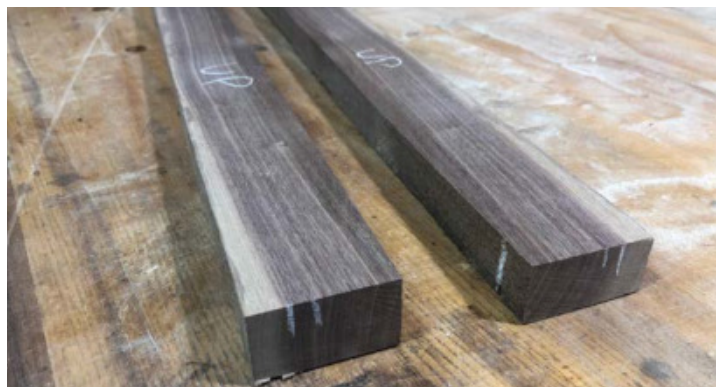
Continuous Grain – These two pieces were cut from a single piece of lumber, then had their inner faces both dressed lightly. Next, Brown removed material from their undersides to bring them to 3/4" thick. Brown also marked their ends and faces so he knew how their grain related to each other
