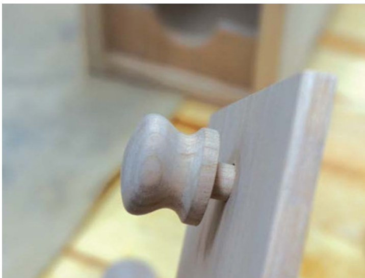
Lock Up That Wine! – Once the upper knob assembly is assembled it can be pulled forward to unlock the sliding door or pushed in to lock the sliding door in place.
