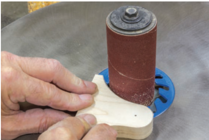
Smooth Curves – A spindle sander makes quick work of smoothing the curves on many of these curved parts.
