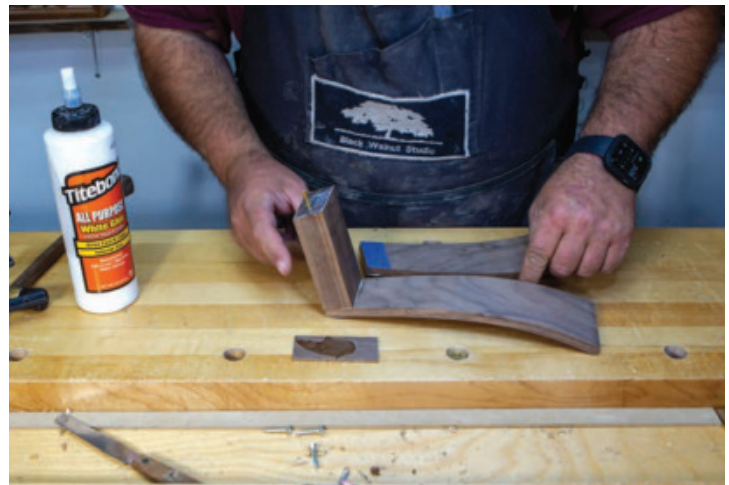
Two Adhesives – White glue works well on wood, but it won't hold the brass pins well. Der-Garabedian mixes up some two-part epoxy to secure the pins once the joint is together.
