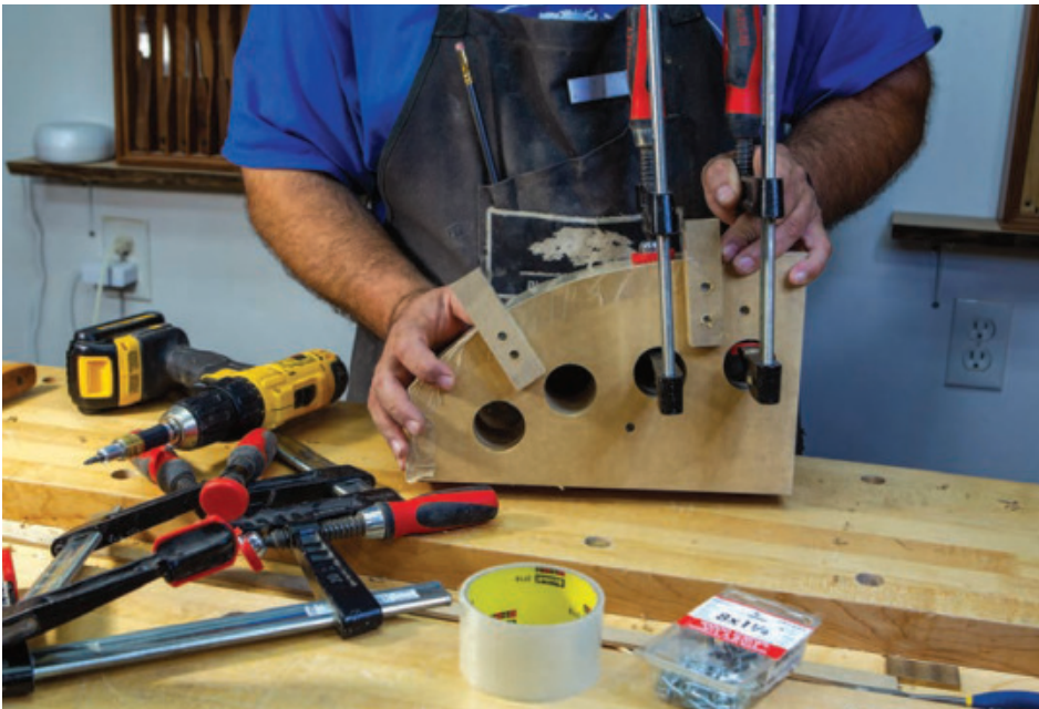
Clamp Holes – Holes to accept the clamp jaws can be added to the form. This allows the user to add clamping pressure perpendicular to the joint over the entire curve.
