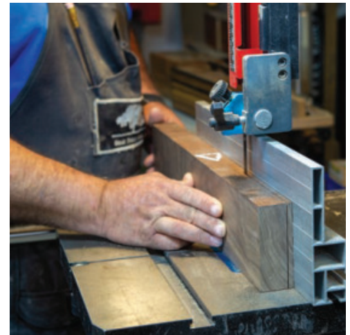
Thin Layers – Der-Garabedian resaws thicker stock to obtain six laminations 1/8" thick. Notice the cabinetmaker's triangle on the upper edge of the stock so he can glue the layers up how they were cut from the board, ensuring even grain and colour.
