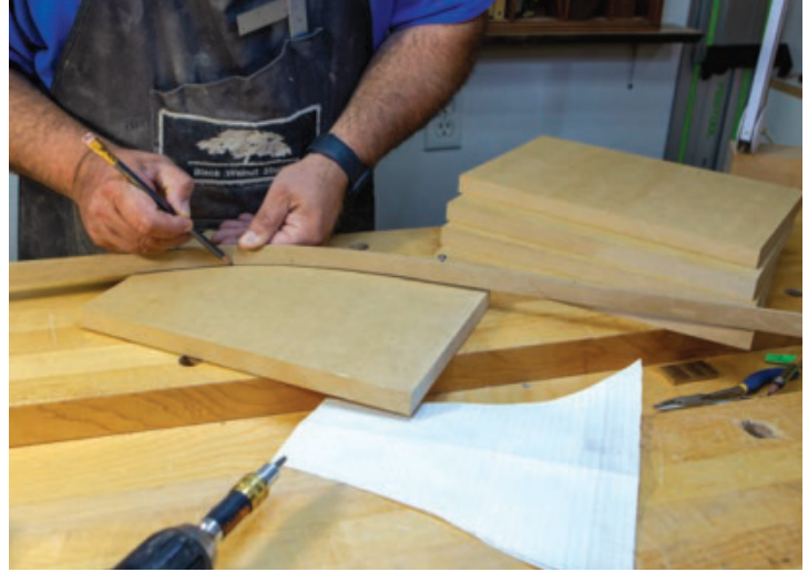
A Curved Form – The exact radius for the form isn't important, so Der-Garabedian uses a thin piece of material to give him an even curve to trace.
