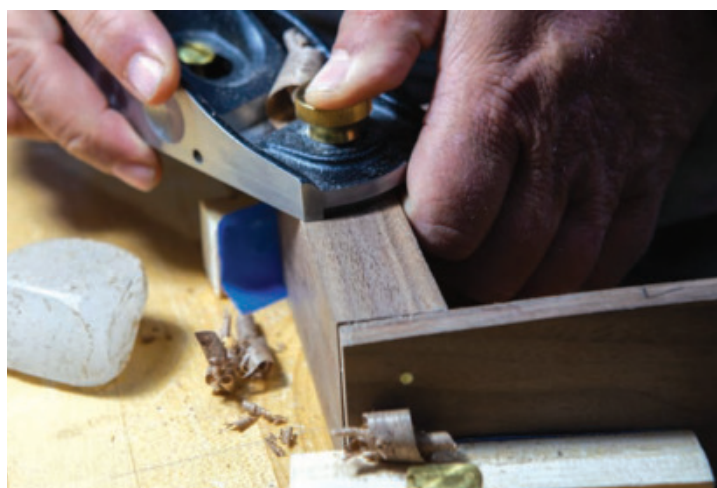
Block Plane to the Rescue – A block plane will smooth out any unevenness in the joints and allow the top and bottom panels to sit flush on the sides.
