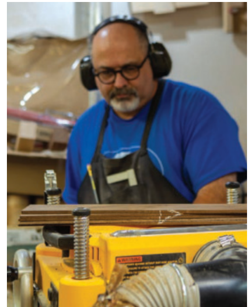
Cabinetmaker's Triangle – Used to keep track of multiple parts, a cabinetmaker's triangle is helpful in many situations. These parts are cut from one piece of wood and will be glued up as they were cut from the board.
