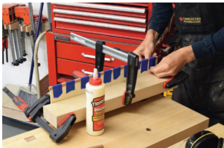
Solid Wood Edging - The sides of the panel are edged with solid wood before the face veneer is applied. The edging is oversize in thickness and in width to make it easier to work with. Blue tape provides plenty of clamping pressure and a wooden caul clamped to the panel ensures it's flat. Once the glue dries, level the edging so it's flush with the plywood.
