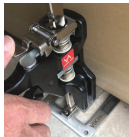
Two Lowering Options – When under load, there are two options for lowering the upper jaw. The thumb lever on the left offers very controlled lowering by any distance up to about 3/16" per press, while the lever on the right releases the upper jaw's grasp on the shaft entirely. (Photos by Rob Brown)
