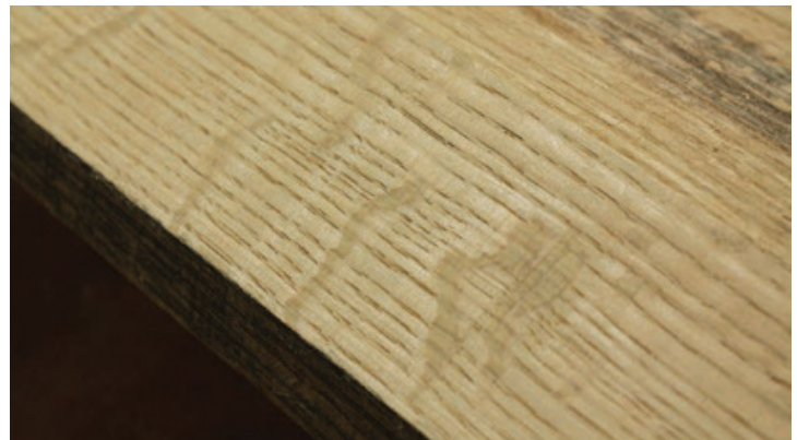
Medullary Rays – While they have a different function for a growing tree, medullary rays provide a striking focal point when lumber is quarter cut. Red oak is one of the species that has very pronounced rays.
