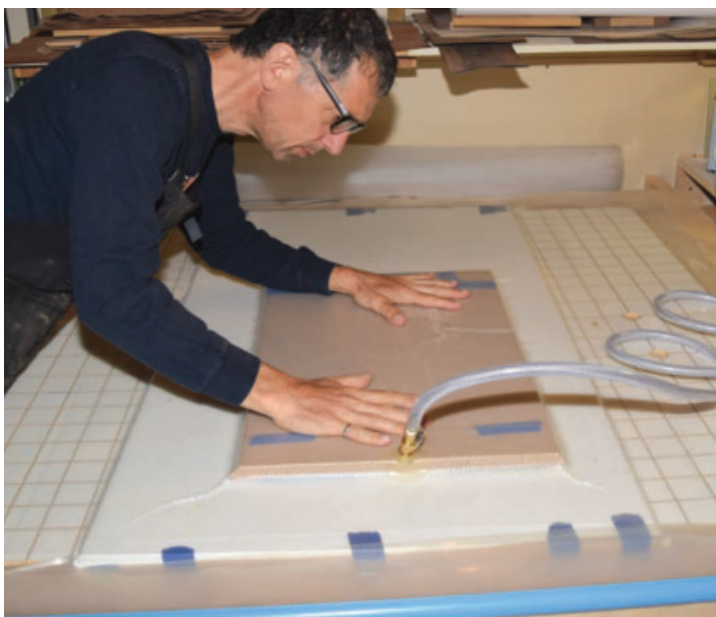
Remove the Air - The three-layer sandwich is clamped in his vacuum bag veneer press. The sheet of veneer between the plywood is needed so the grain direction of each layer is perpendicular to the next. The alternating grain direction will continue when the face veneer is applied.
