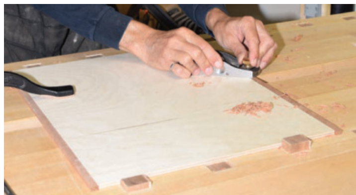
Stable Core - Bedrosian uses Titebond original on the inside faces of the 3mm Baltic birch plywood panels; he applies glue to the core, not the veneer.
