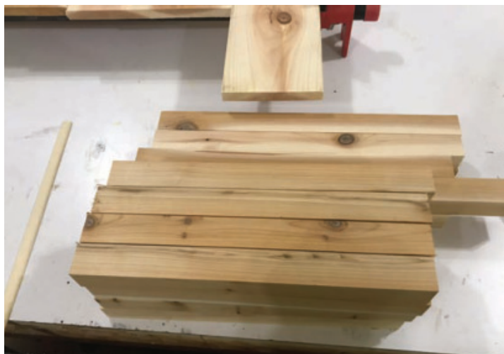
Rails and Stiles – The rails and stiles are cut from 2×4s, then dressed to final dimensions.
