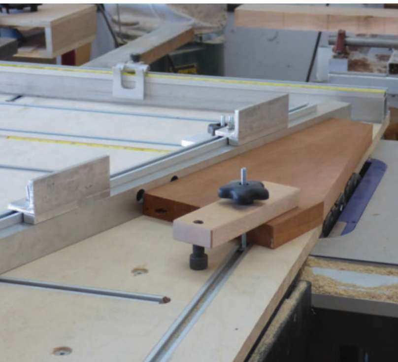
Clamp It Down – Shop-made hold-down clamps are very useful to have around. Make at least three, and you'll be happy you did.
