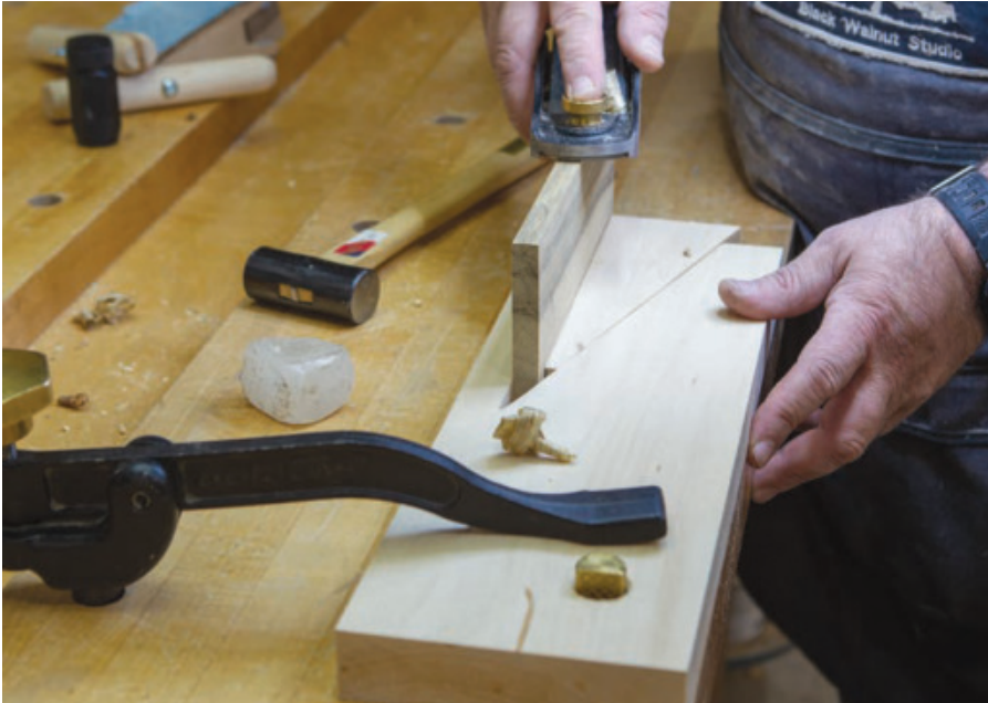
A Strong Bite – The slightly rough band sawn edges of the wedge and main section of the jig provide a lot of friction and hold a workpiece stationary when in use.
