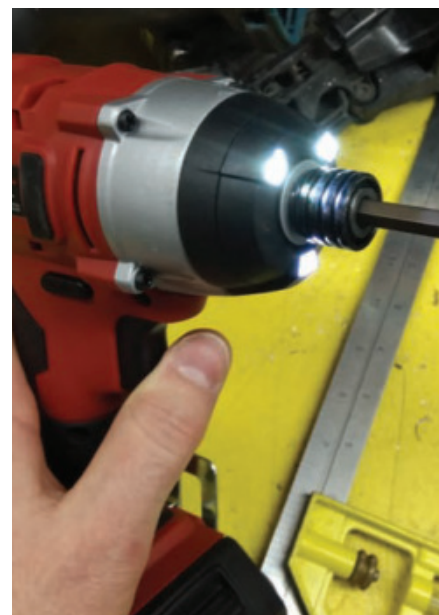
Shed Some Light – Three LED lights come on when the trigger is pulled, shining excellent task lighting on the immediate area where you're working. (Photo by Rich Keller)
