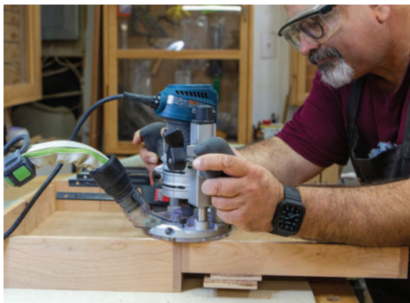
Hinged – Der-Garabedian mortises for the toolbox hinges after supporting the thinner half and clamping the pair together.
