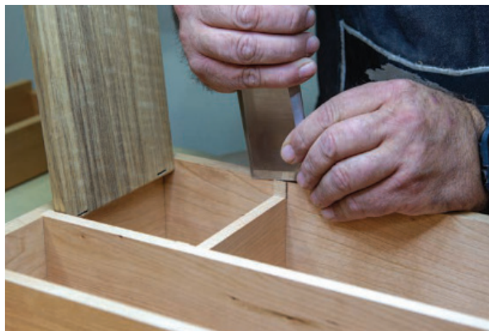
Close Shave – Final trimming of the door compartment divider is completed in place with a sharp chisel.
