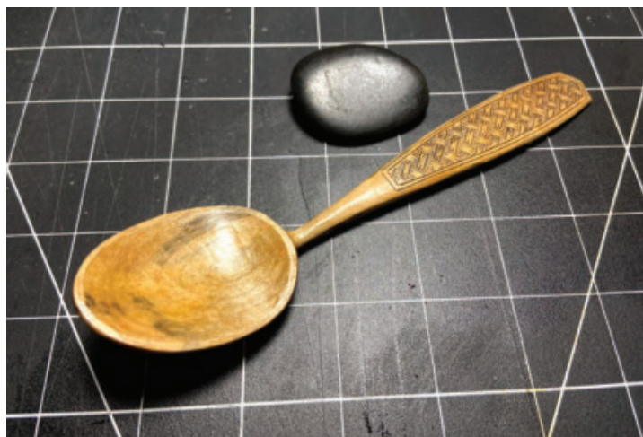
Burnish the Design – After another light application of oil over the design, use a smooth stone or another smooth, hard object to burnish the kolrosed surface. This helps to close the gaps in the wood fibres, and locks the coffee pigment into place.
