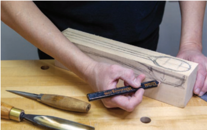
Sketch it Out – With your spoon blank cut roughly to size, draw the top view of the spoon onto it. The side view can also be drawn on, even though it will get cut off shortly. It’s sometimes easier to align the top and front view while the blank is in one piece, and the offcut with the side view on it can be used to help lay out those cuts down the road.
