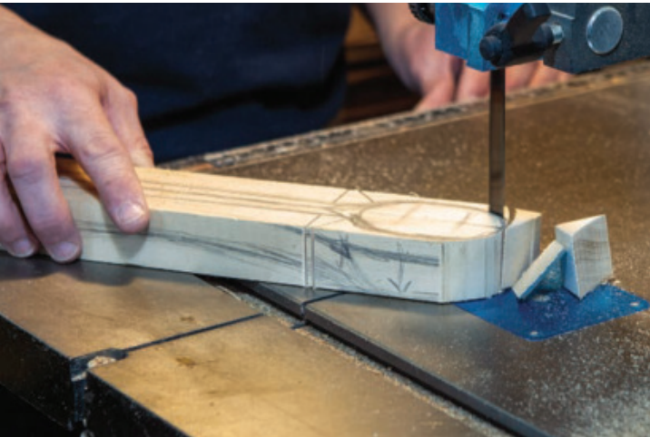
Shape with a Band Saw – A band saw will make quick work of most of the waste, quickly roughing out the spoon.
