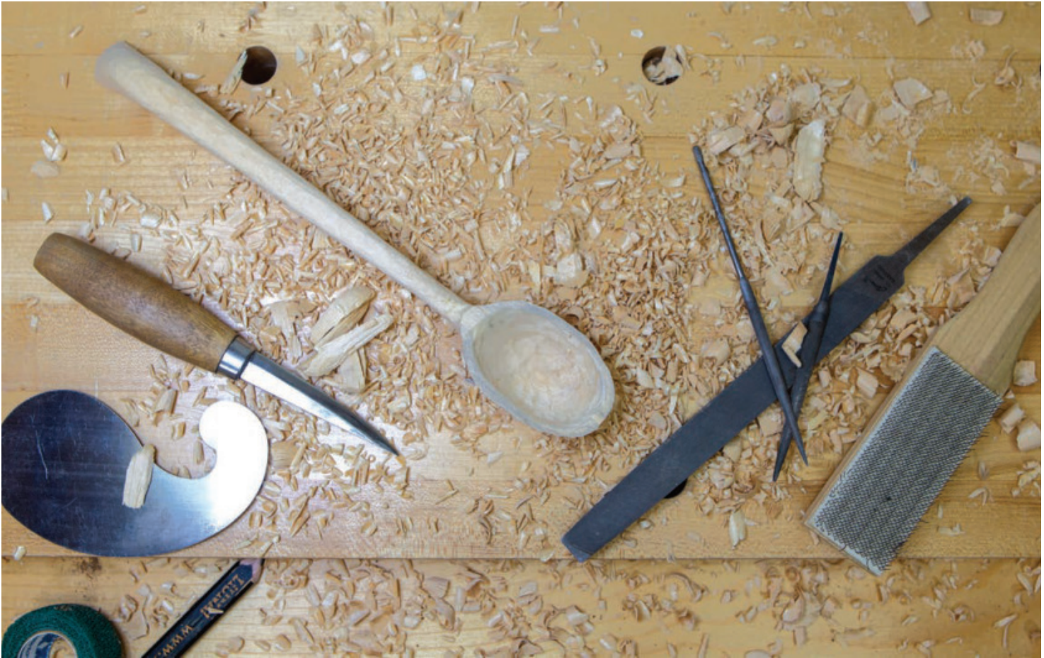
Basic Tools – A medium-sized selection of tools, most of which woodworkers already have, is all that’s needed for this spoon design.
