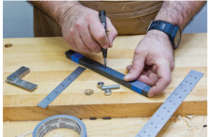
Cross Pieces – The magic parts that makes this vise work properly are the cross pieces that keep the jaws parallel during use. Start off by taping them together and drilling a hole in the center of the pair.
