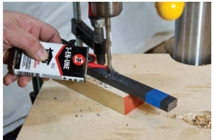
Oil Helps – Drilling metal is similar to drilling wood, but with a few main differences. Oil will help lubricate the bit. Also note the clamp that will act as a stop if the metal parts grab the drill bit and cause the metal to spin out of control.
