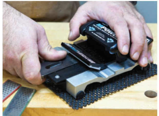
Thumb Pressure – While moving the carriage back and forth, thumb pressure keeps the blade in place so it can be sharpened.
