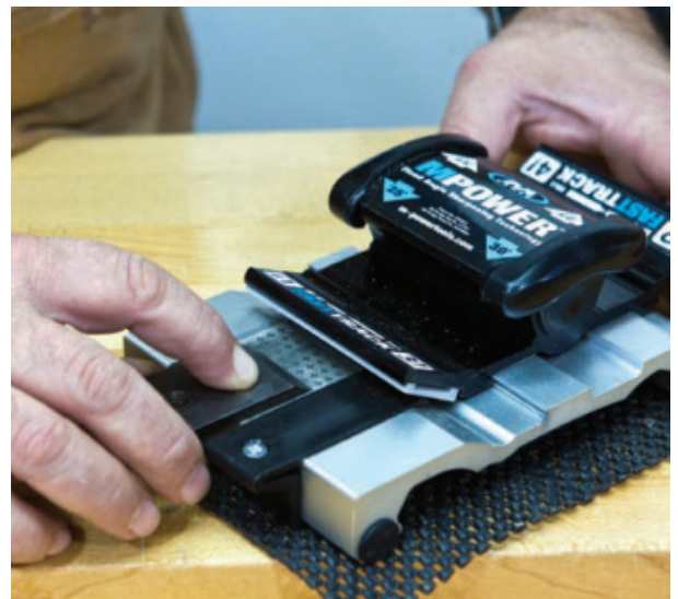
De-Burring Plate – After each grit has been used on the blade, it's necessary to pass the blade over the de-burring plate a few times to remove the burr. It's a quick and easy part of the process.
