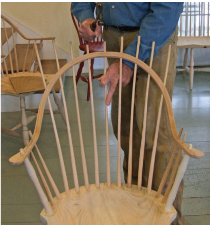
Driving Spindles Home – Glue is applied to the mortises, the spindles are aligned with them and they are driven "home" with a hammer.
