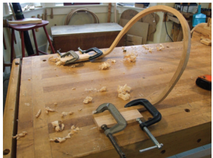
Gluing up Hand Blocks – Blocks are added and clamped to the outer edges of the arm rest that will be shaped into the hand rest.
