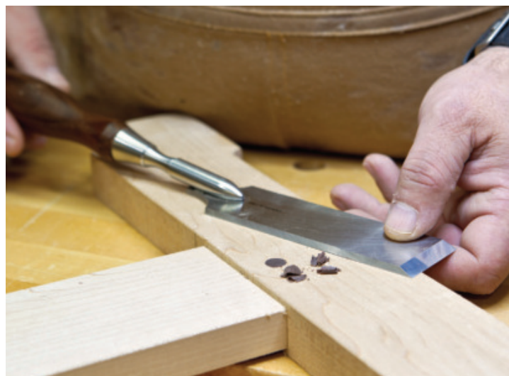
Flush it Up – Der-Garabedian enjoyed using the chisels for tasks like flushing up the pin that helps hold a mortise and tenon joint together.
