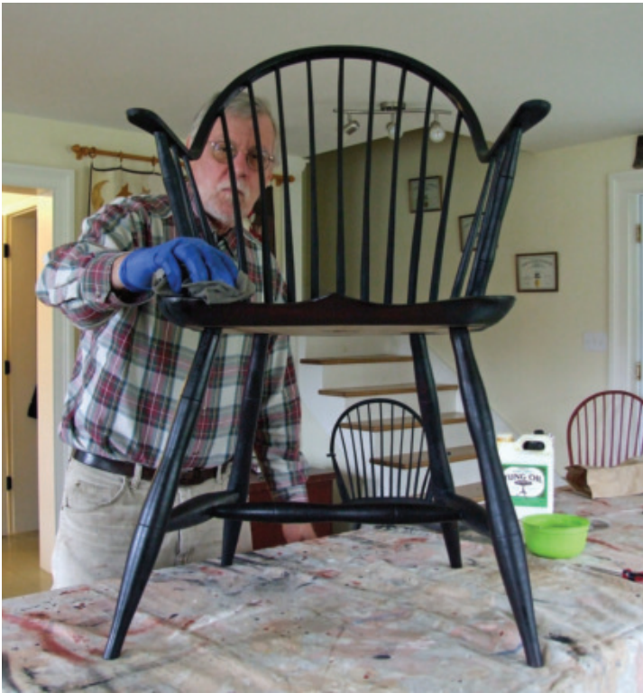
Tung Oil Applied to Chair – With the black paint lightly distressed, and the entire surface then sanded smooth, tung oil is hand rubbed into the chair legs
