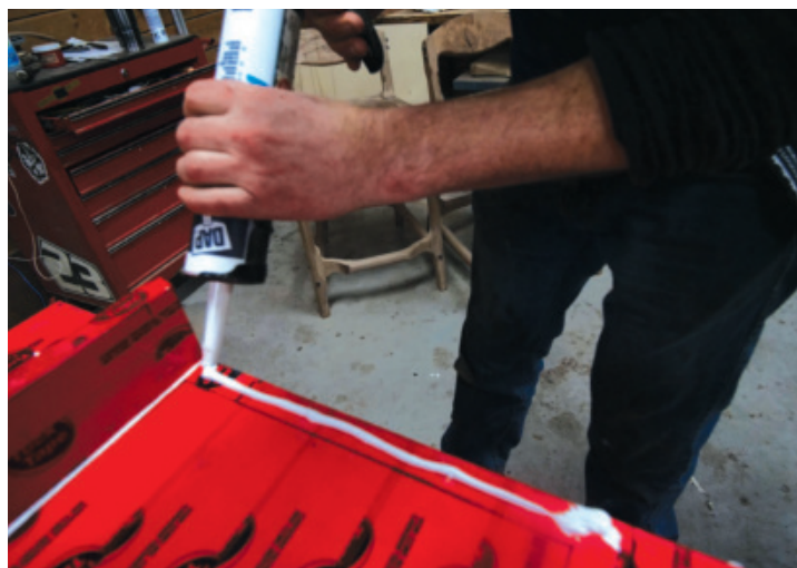
Seal the Joints – Because the joints all need to contain liquid epoxy, they need to be watertight. A healthy bead of caulking will help with this.
