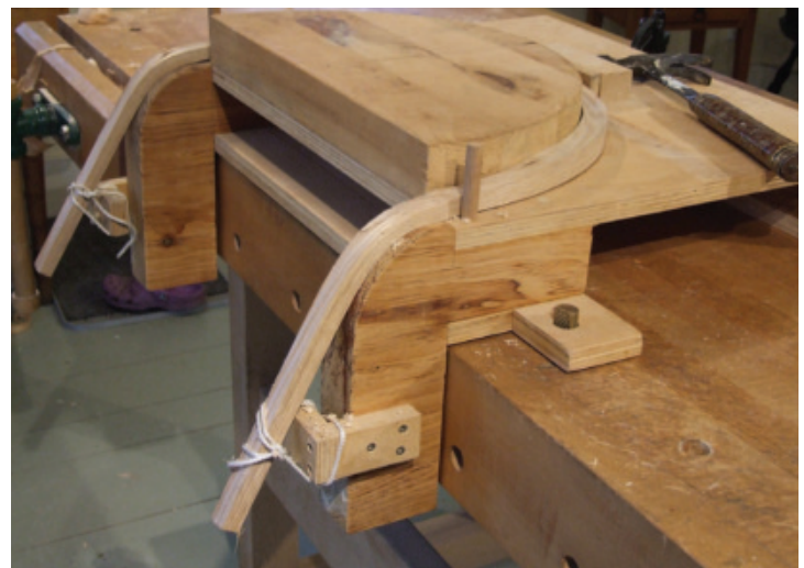
Bending the Arm – The steamed arm is bent, tied off on the form and left to dry on the form for two days.
