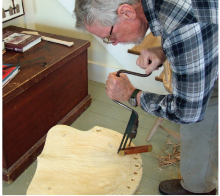
Drilling Spindle Mortises – Spindle mortises are drilled with a brace, a #9 spoon bit and a bevel square set at the appropriate angle on the spindle platform.
