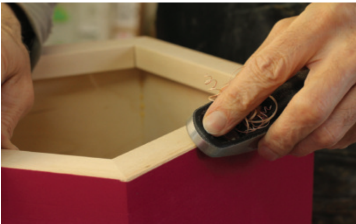
Chamfer the Edges – To create a smooth, clean transition between the painted surface and the header's raw wood, Brown takes a few passes with his block plane. Any overspray was removed at this point.
