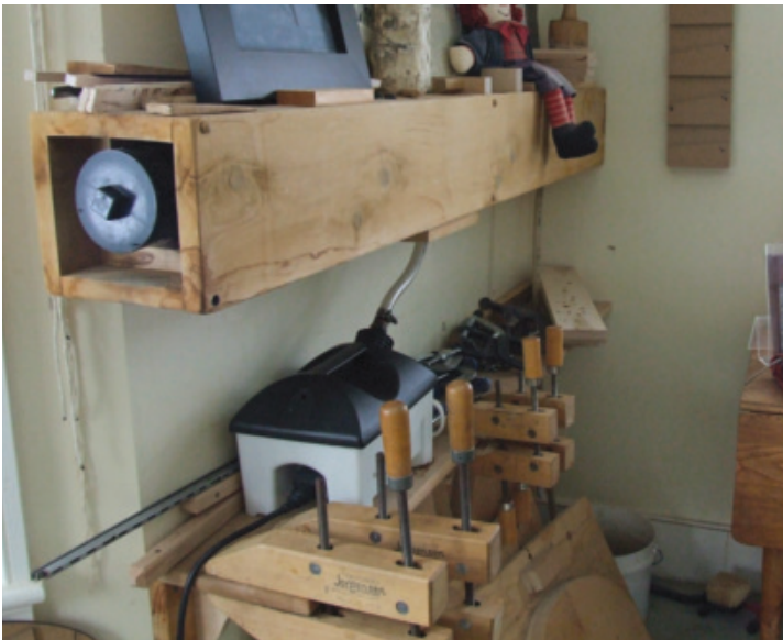
The "Steam Box" – A wallpaper steamer and ABS piping are used to construct a "steam box" for bending.
