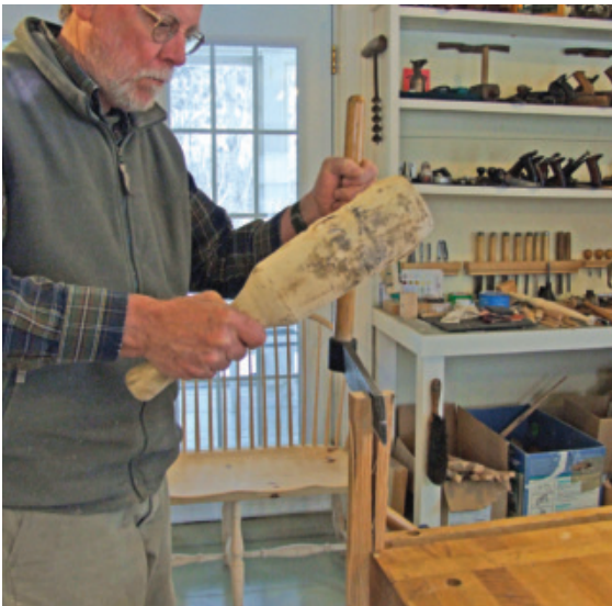
Splitting Spindle Blanks – Oak is rived to form spindle blanks using a froe.
