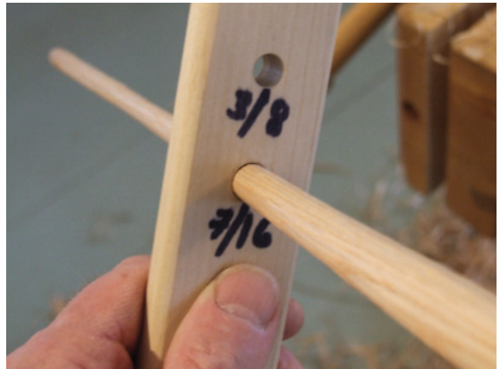
Using a Go Gauge – A "go gauge" is used to measure the spindle diameter.
