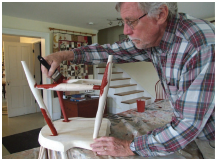
Painting Legs – The chair is turned upside down on the corner of the bench and the legs are given a first coat of paint.
