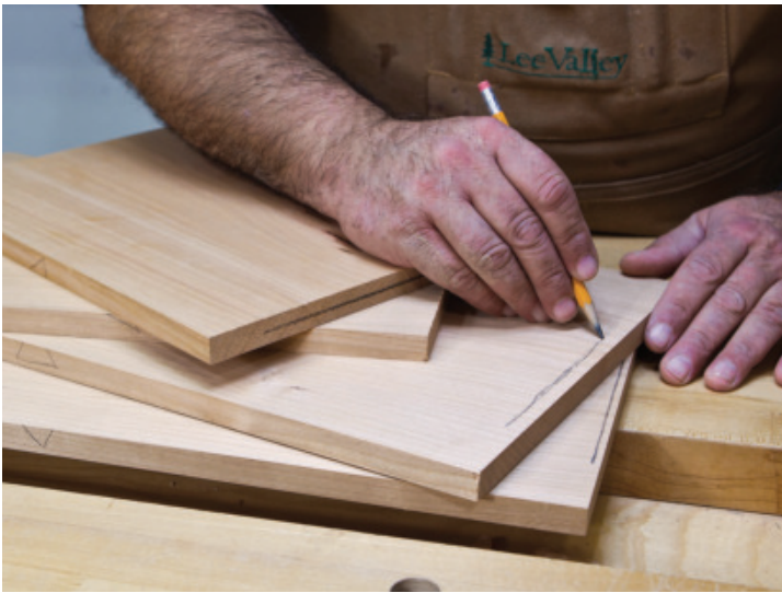
Draw it On – Adding pencil marks where joinery needs to be machined is a great approach to keeping all of the parts straight in your mind.
