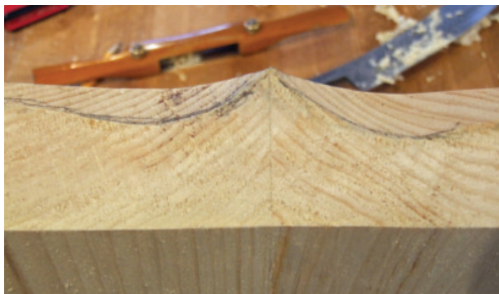
Pommel Defined – A pencil line is drawn to help define the seat pommel. The material above the pencil line will eventually be removed when the seat is dished out with an adze, scorp or other tools.
