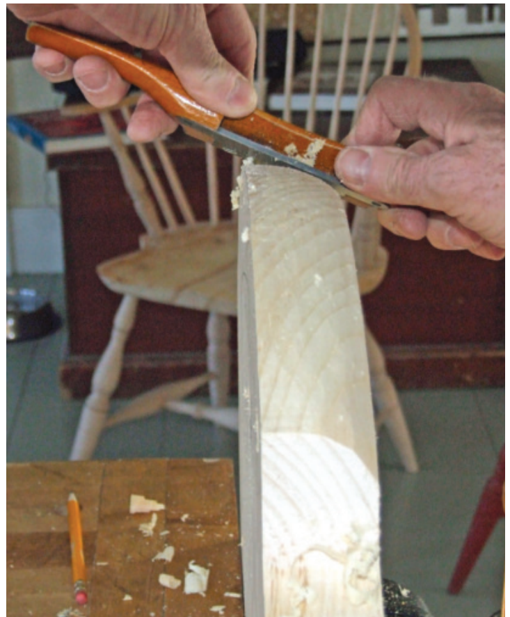
Smoothing Seat Back – The back of the seat is smoothed using a low angle spoke shave.
