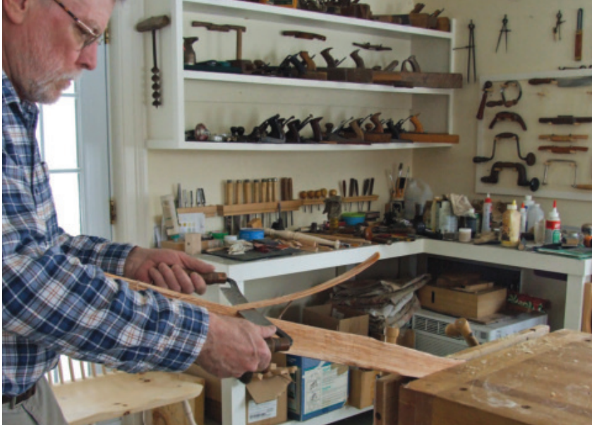
Roughing Out the Arm Blank – A draw knife is used to rough out the arm blank to approximately 1" square.
