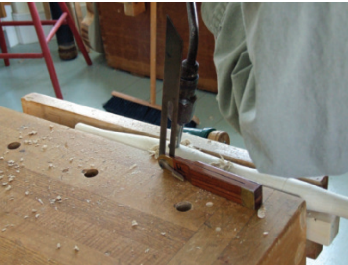
Drilling Leg Mortises – Mortises to accept the side stretchers are drilled in the legs at the appropriate angle using a brace and #10 spoon bit.
