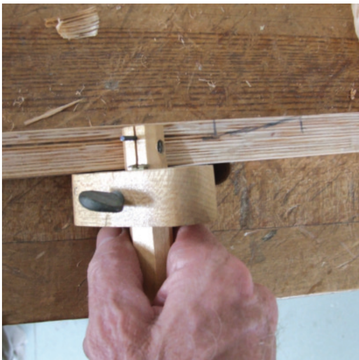
Marking the Thickness – A scribe is used to mark the target dimensions of the arm rest.
