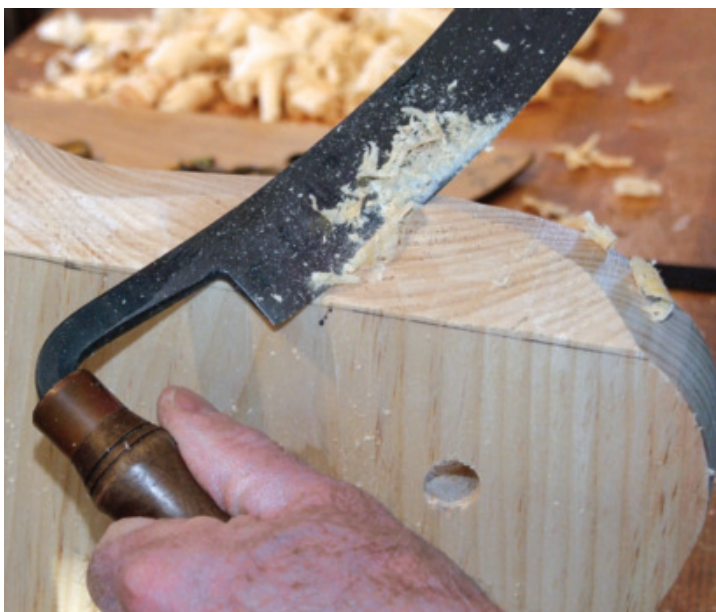
Seat Front – The seat front is carved flat using a drawknife.
