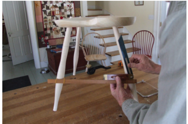
Leg Mortise Angles – A winding stick is held with a string or elastic at the leg mortise marks on the front and back legs. A bevel square is then used to determine the angle of the front and back mortises.
