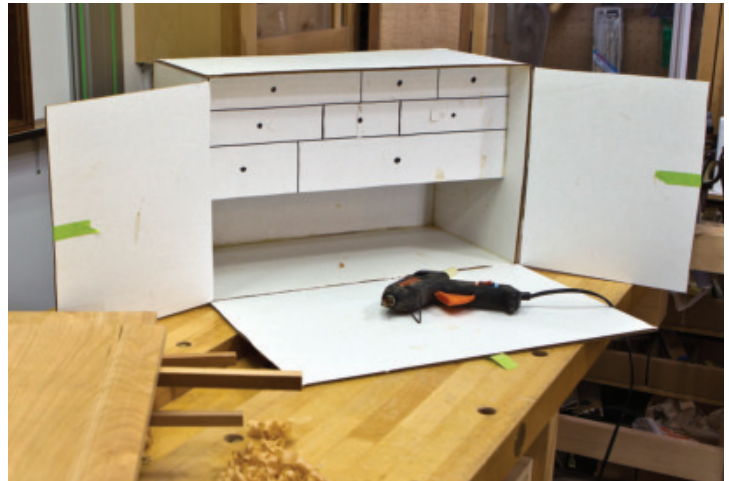
Mock It Up – A simple approach of cardboard and hot melt glue will allow you to quickly and cheaply mock up the chest for size and looks.
