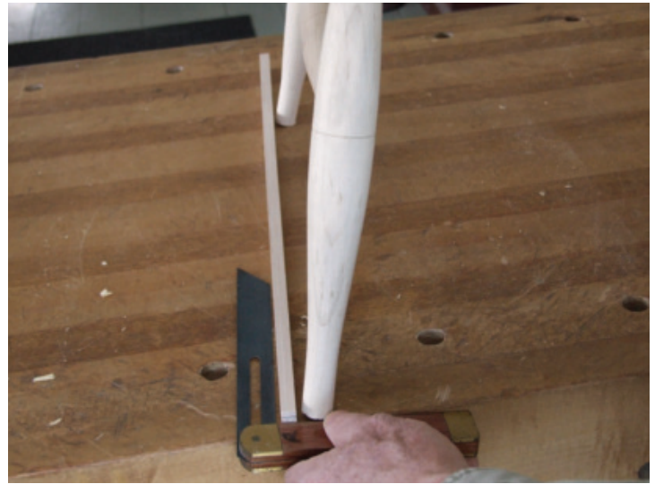
Determining Center Stretcher Angle – The front legs are placed against the front of the bench and a winding stick between the front and back legs. The angle formed between the winding stick and the front of the bench is the angle that the mortises are drilled in the side stretchers to accept the center stretcher.
