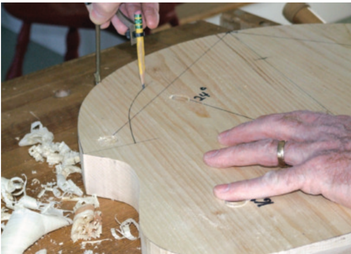
Scribing Saddle Platform – A compass is used to scribe a reference line for the spindle platform.
