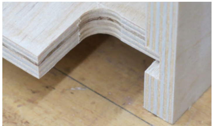
Careful Notches – Salusbury bored a hole in the inside corner of the notch in the bottom, then used a band saw to make the straight cuts. This notch will fit around each leg.
