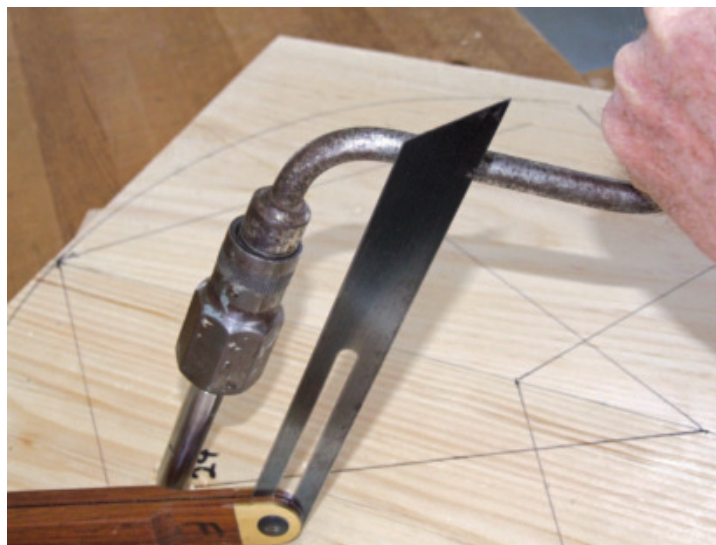
Drilling Through – The mortises are drilled through the seat blank using a spoon bit and brace.
