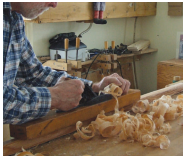
Planing the Arm Blank – A jack plane is used to smooth and square up the arm blank.
