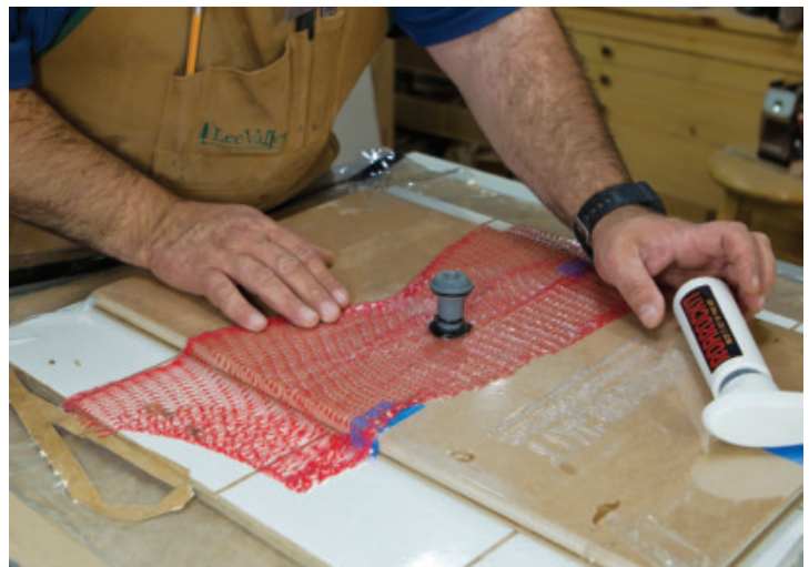
Lots of Options – Der-Garabedian chose a Roarokit vacuum kit to press his back panel, some cauls, a pair of platens and a bunch of clamps would have also worked nicely.
