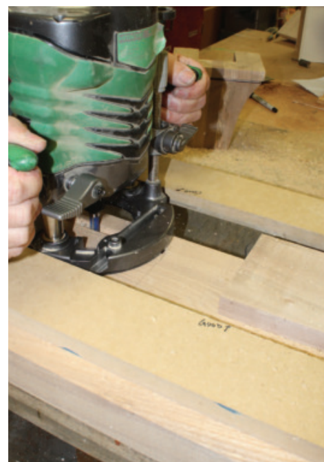
Simple Router Jig – Coleman used two long, straight pieces of MDF on either side of the router's base, and two short pieces towards either end of the long pieces to make a jig to guide his router. The two long fences trapped his router, and ensured it wouldn't stray from the intended path while routing the grooves with multiple passes.
