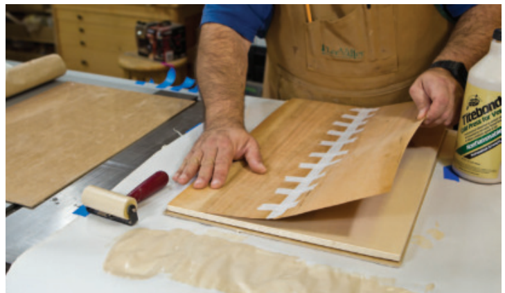
Veneer is an Option – Although you could just use plain plywood, adding veneer to both surfaces of the back panel is a nice look for this very refined chest.
