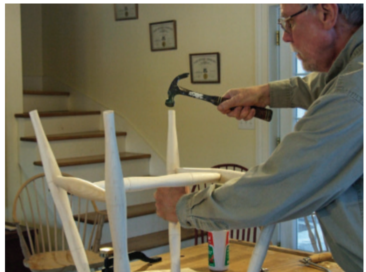
Determining Center Stretcher Angle – The front legs are placed against the front of the bench and a winding stick between the front and back legs. The angle formed between the winding stick and the front of the bench is the angle that the mortises are drilled in the side stretchers to accept the center stretcher.
