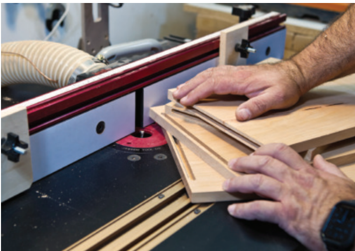
Case Grooves – A 1/4" diameter bit, chucked into the router table, will make quick work of the grooves that will hold the main carcass together.
