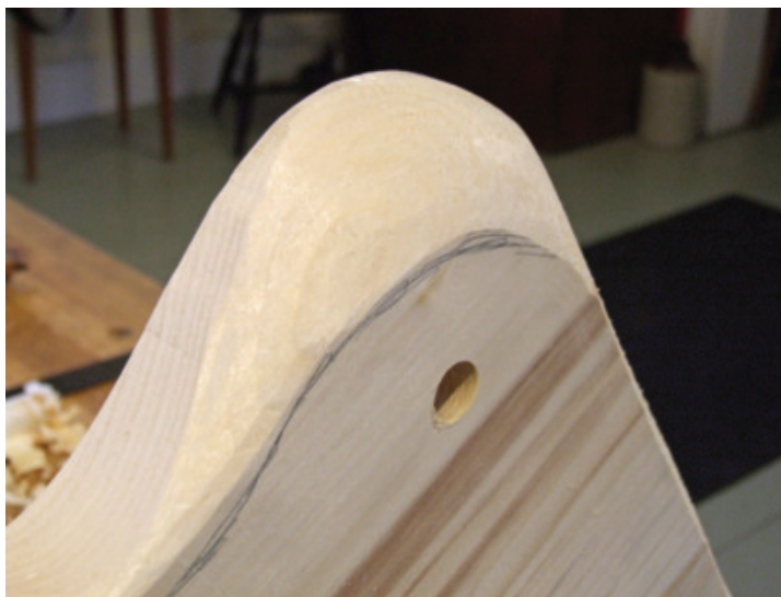
Completed Seat Transition – The finished transition from the back to the front face of the seat.
