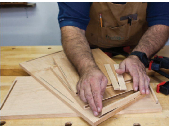
Splines for Strength – Solid wood splines will locate the joint during assembly, and add needed strength to the case.
