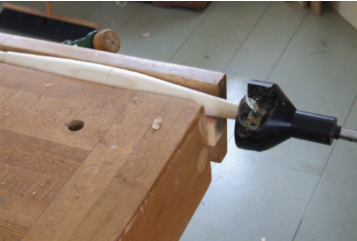
Cutting the Tenon – A tenon cutter is used to make tenons on each end of the stretchers, which are held in a vise during the process.
