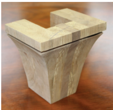
Machined and Sanded – The curves on this base aren't so tight they're hard to sand. You might want to keep this in mind when laying out your curves.
