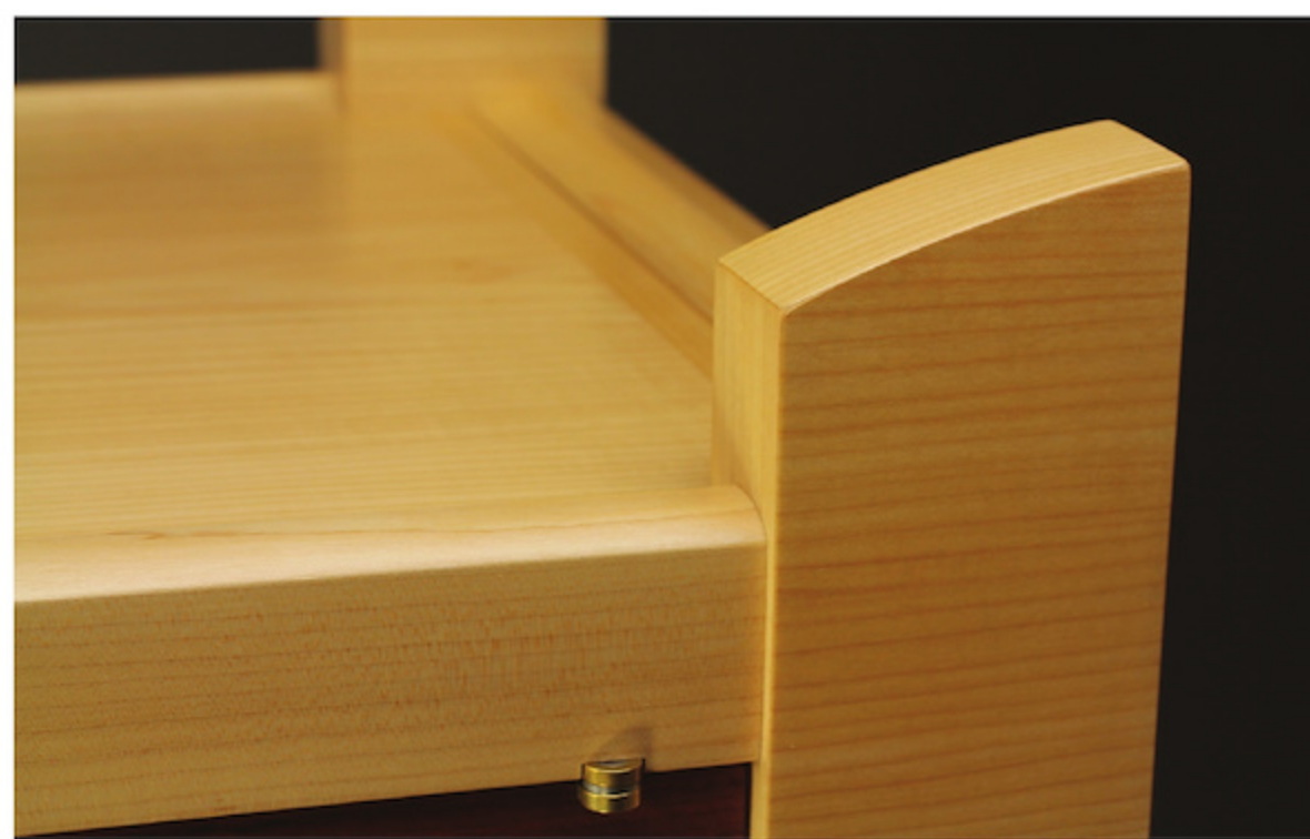
A Clearer Finish – Oil-based finishes add a darker, richer look to most woods, and that involves imparting a yellowish tinge to the wood. Water-based finishes don't add nearly as much yellow to the overall colour of the finished wood. This is especially important for people finishing a light-coloured wood, like the maple frame in this cabinet.
