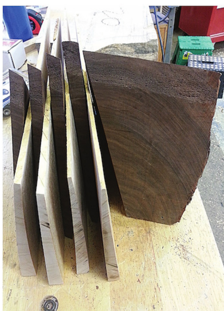
Making Wedges – Rude cut maple wedges on his bandsaw, though a plane sled would also make very uniform wedges. A simpler option is to use flat dressed pieces of wood as contrast.
