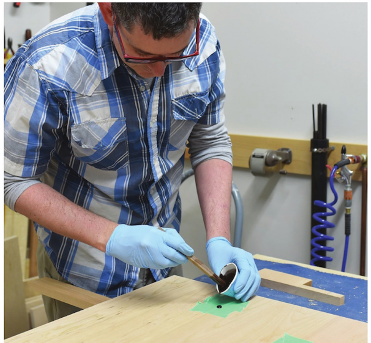
Fill any Gaps – Small imperfections can be filled with coloured epoxy, then sanded flush.
