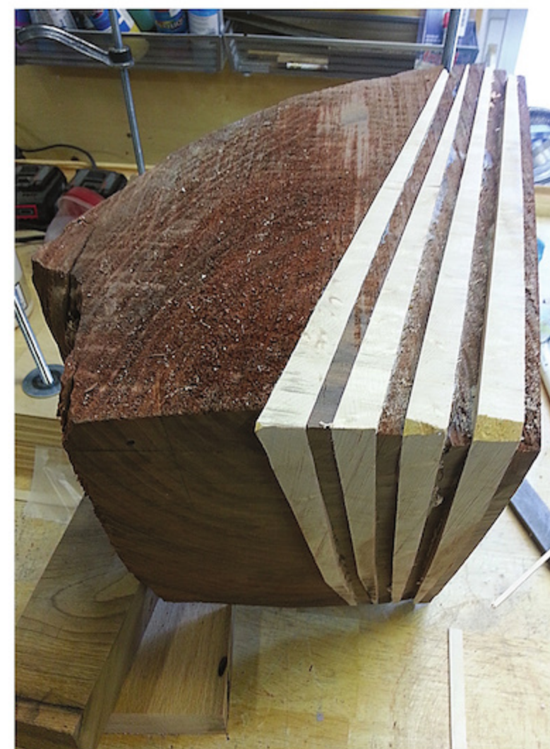
All Glued Up – Once the layers of maple and walnut were cut, Rude glued them together. Gluing these layers a few at a time might be the safest approach.
