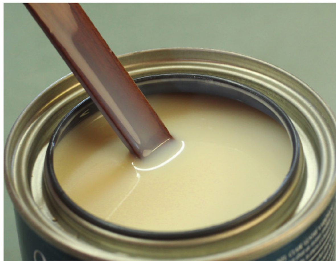
Starts White – Water-based polyurethane is white in the can but turns clear once it's on the wood's surface.
