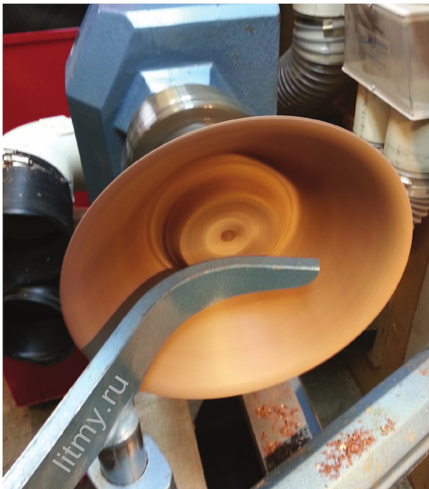
Further Wood Removal – Rude removed the center of the bowl and the tailstock, then finished turning the inside of the bowl before sanding it.
