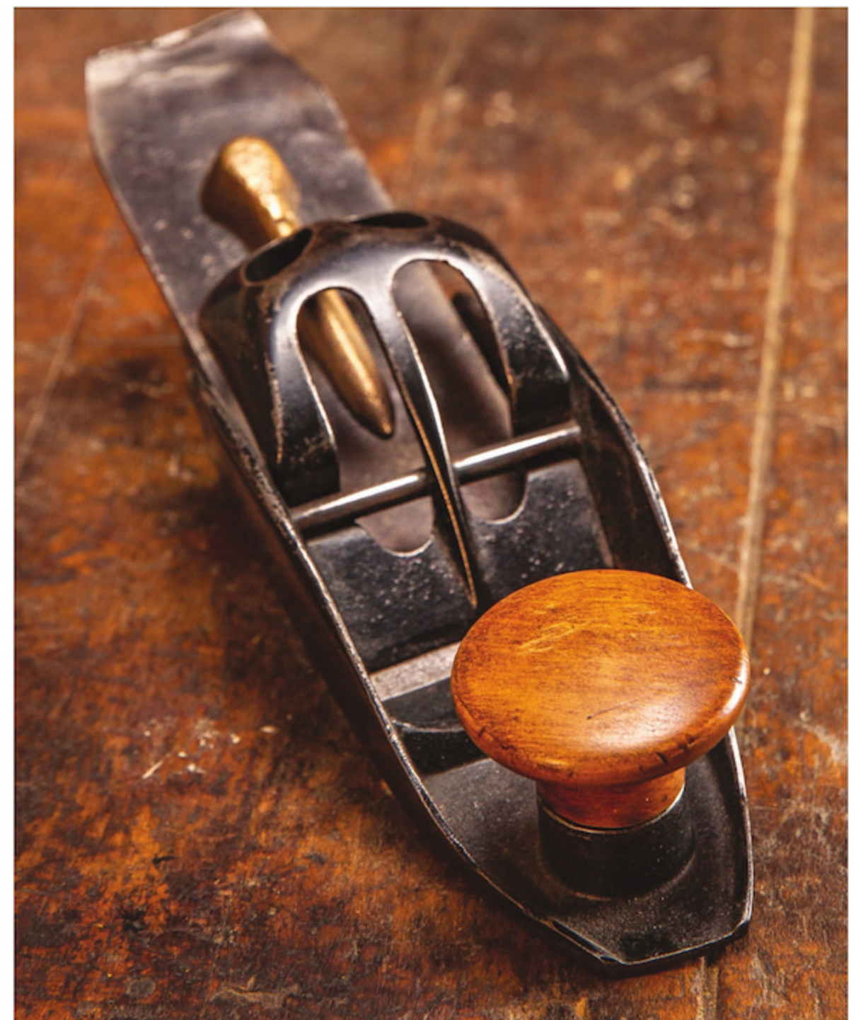
Birdsill Holly – This is the earliest known North American cast metal block plane. It's non-adjustable and dates back to the 1850's.
