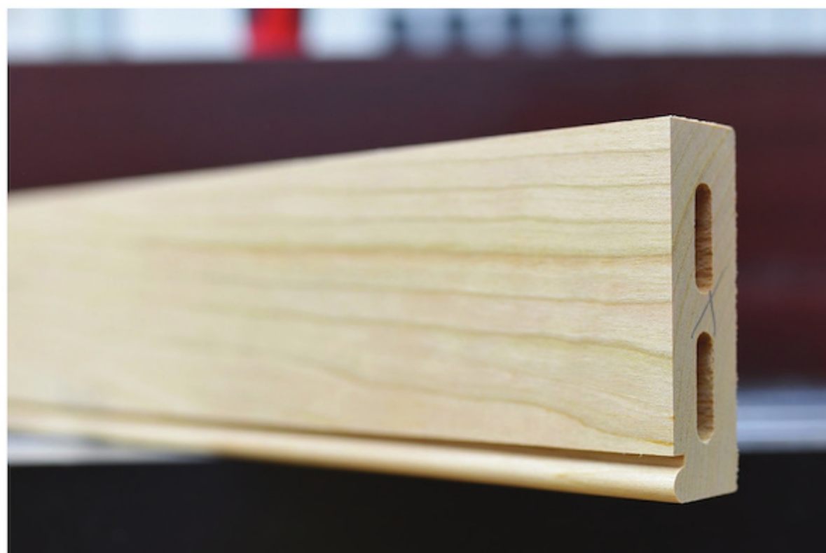
An Even Bead – Having the fence and bit aligned will go a long way to ensuring you end up with an even bead.
