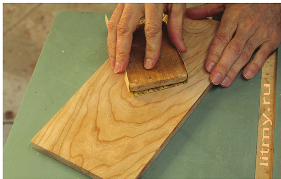
Smooth the Surface – Water-based finishes raise the grain of wood, mainly after the first coat has been applied. Sanding between each coat will smooth the surface for the next coat to go on smoother.
