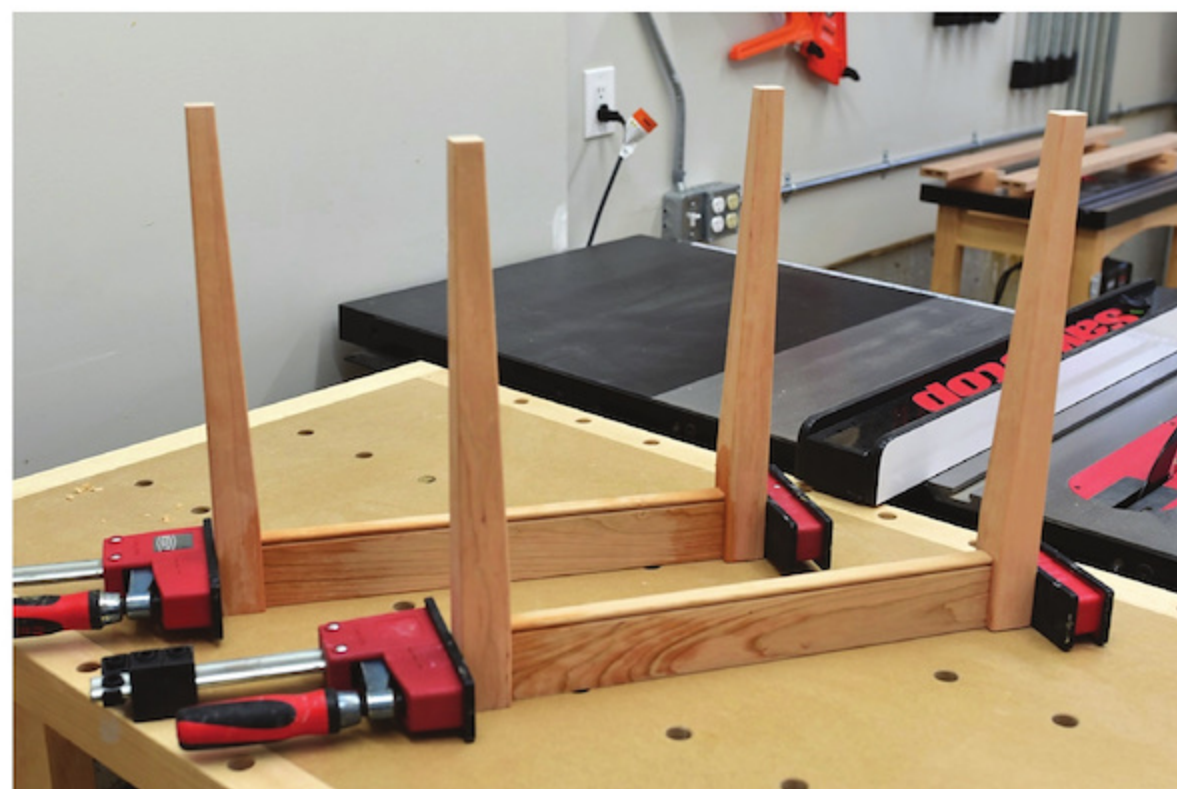
One Step at a Time – Gluing up the base in two stages reduces assembly stress.
