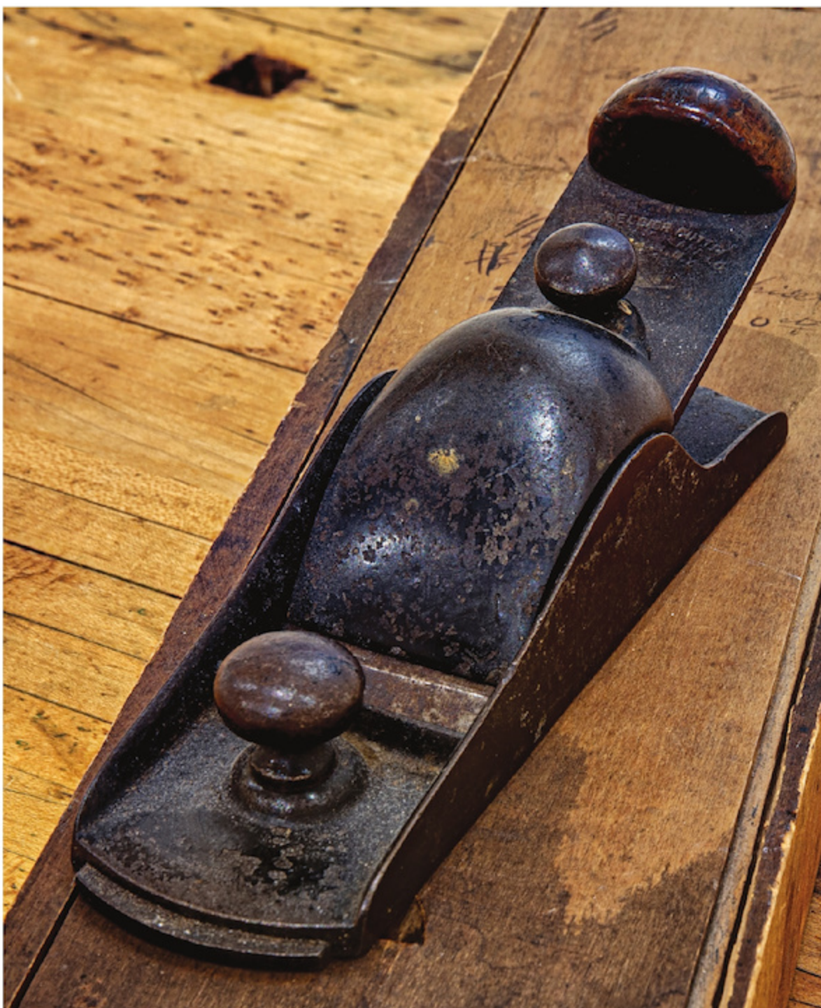
Adjustable Block Plane – A rare Metallic Plane Company No. 8 adjustable block plane, circa 1870's.
