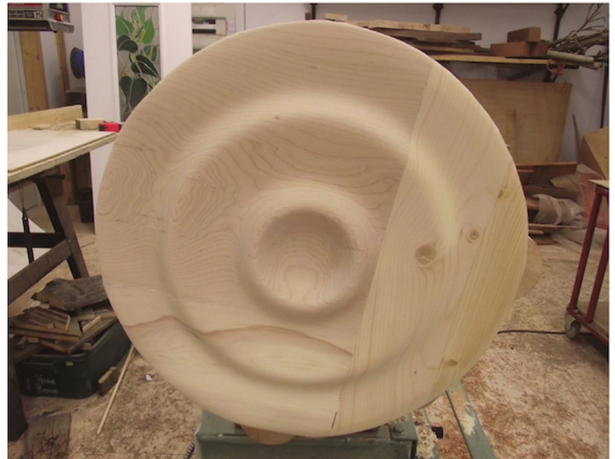
Turned Platter – With the center recess carefully formed, the waves shaped, and the surfaces sanded, you can remove the platter from the lathe.
