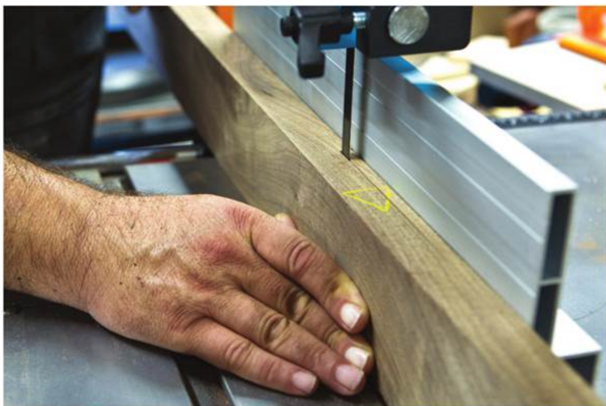
Slice It Up – A well-tuned bandsaw makes quick work of resawing the laminations from a single board. A cabinetmaker's triangle ensures the laminations get glued back together in the order they were cut, to ensure grain and colour match.
