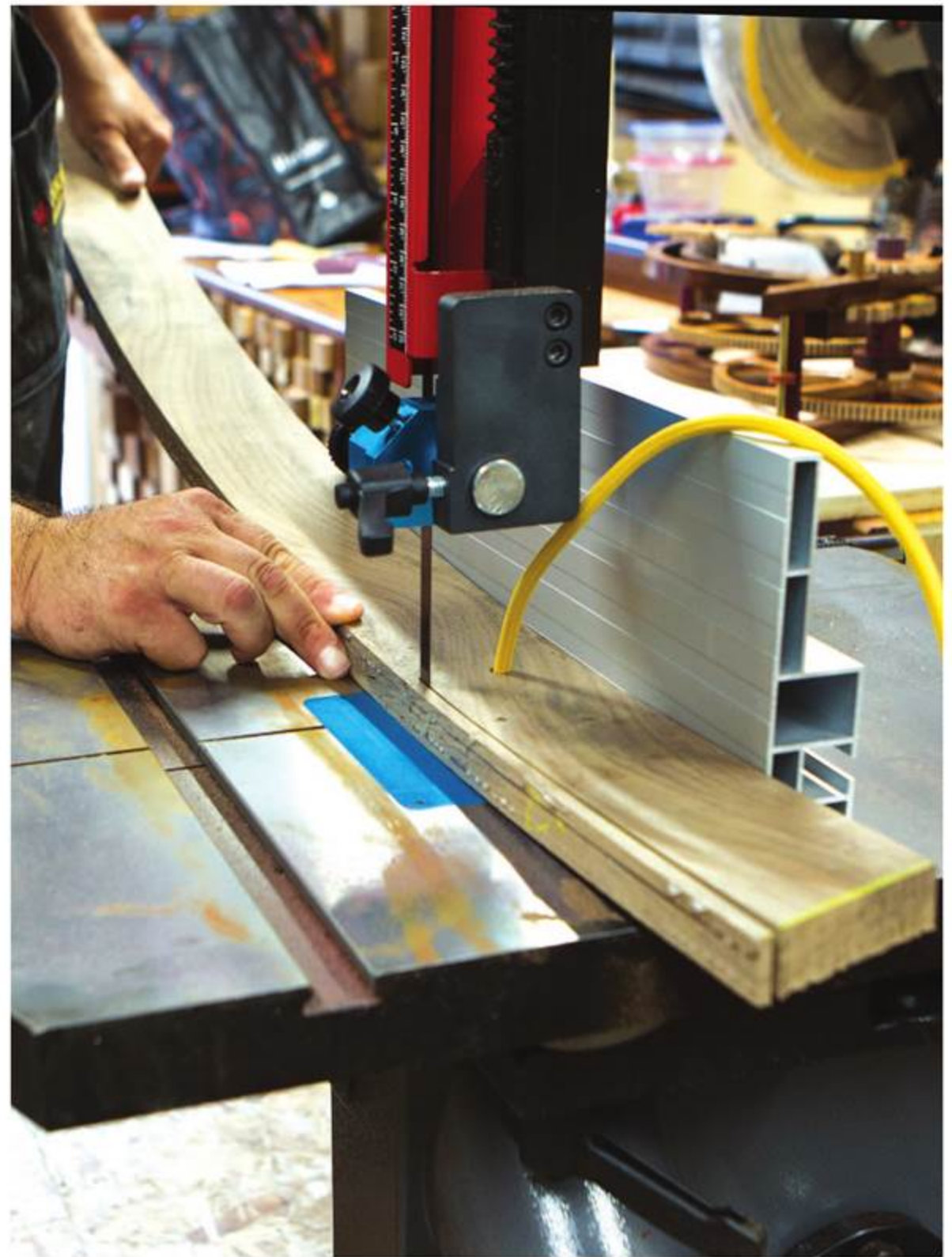
Trim the Opposite Edge – With the bandsaw fence set about 1/16" wider than where Der-Garabedian wants the lamination to finish, he rips the length to rough width, then finishes the edge on a jointer.
