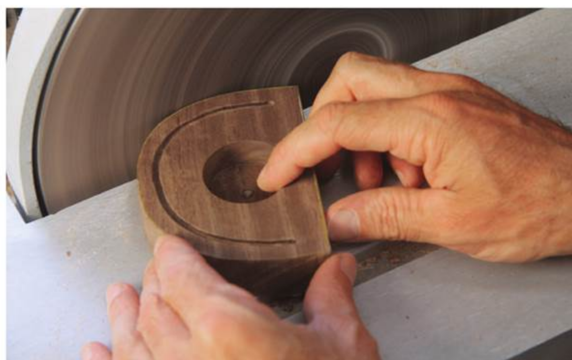
Smooth the Edges – After a bandsaw cuts each tea light holder from the blank, Brown sands the edges on a disk sander.
