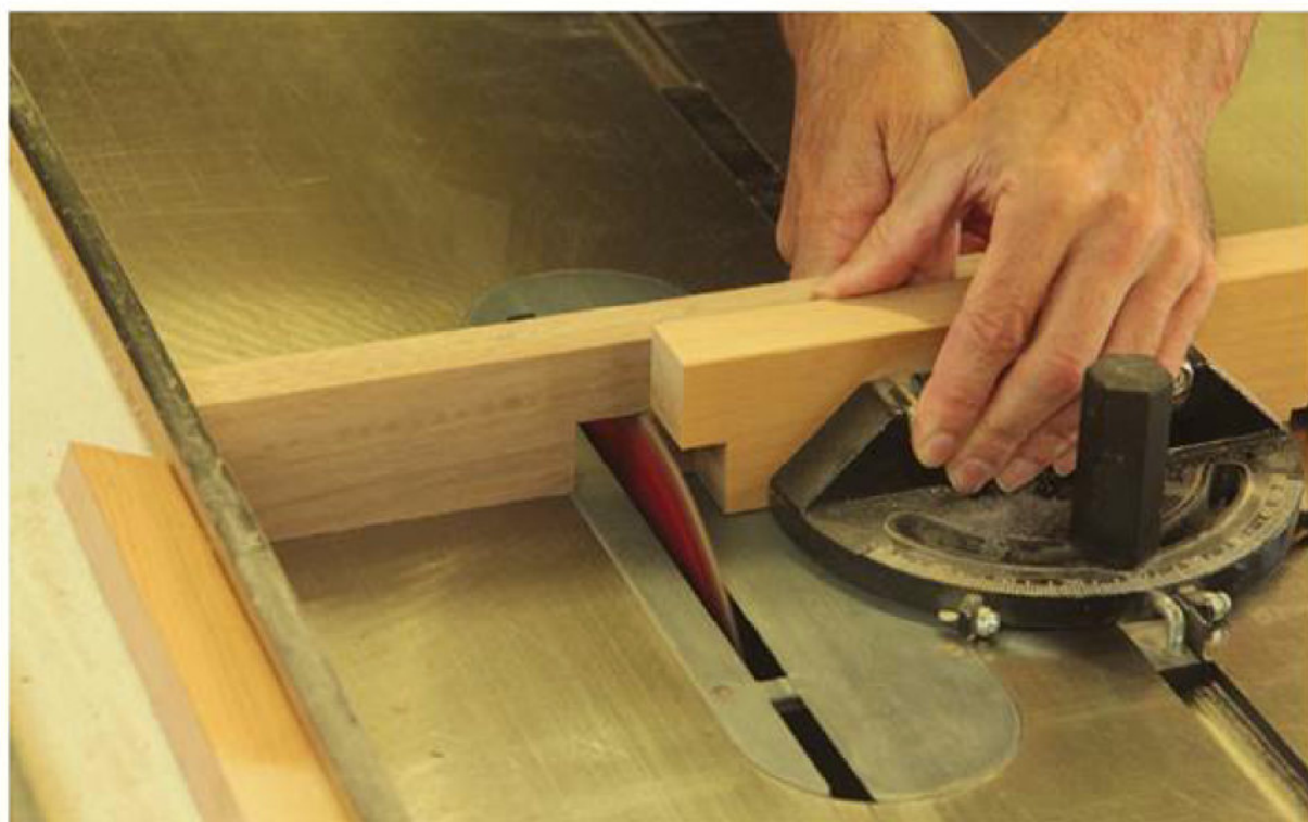
Half Lap – Brown uses his rip fence as a stop to determine the width of the half lap joints in the cross rails.
