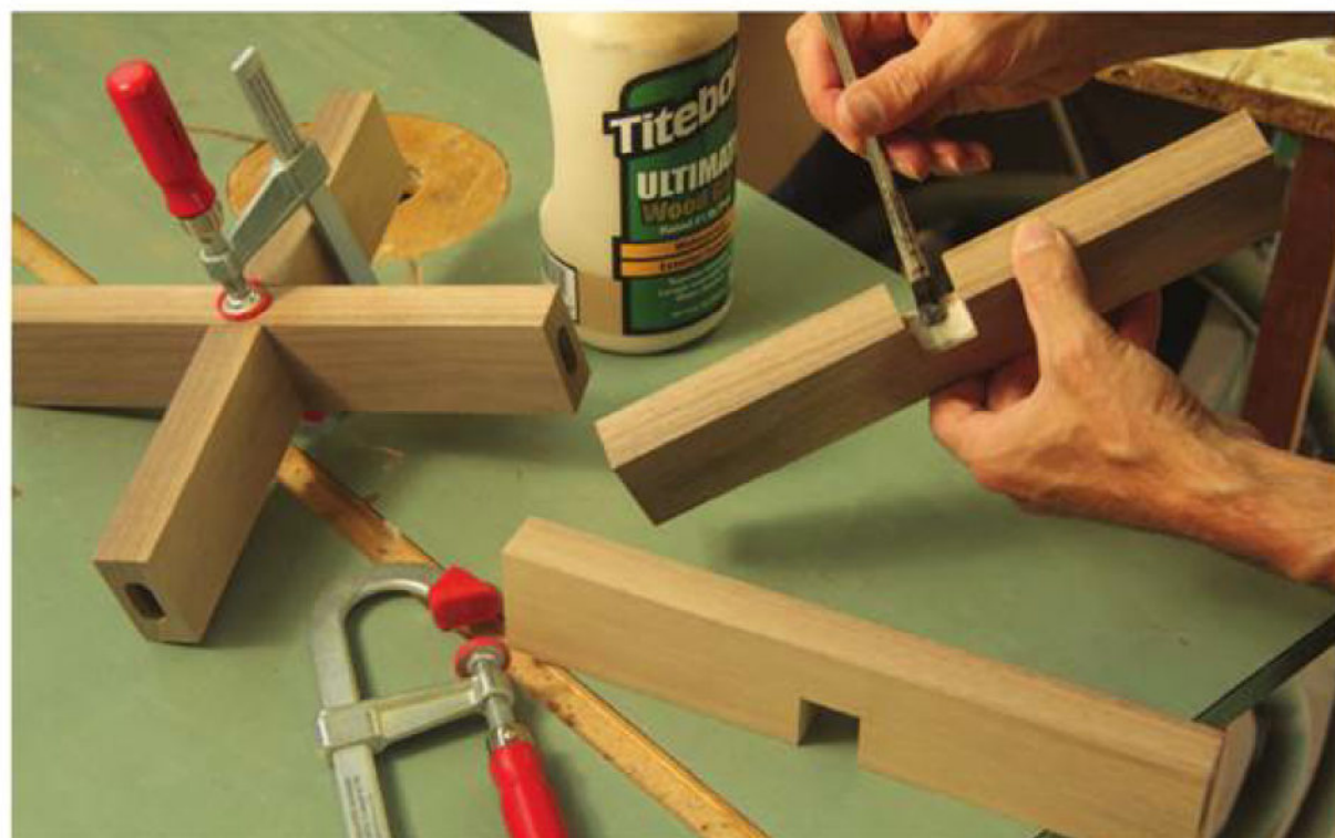
Cross Rail Assemblies – Once the cross rails are sanded, apply glue to the face grain in the joint and bring the mating parts together with a clamp.
