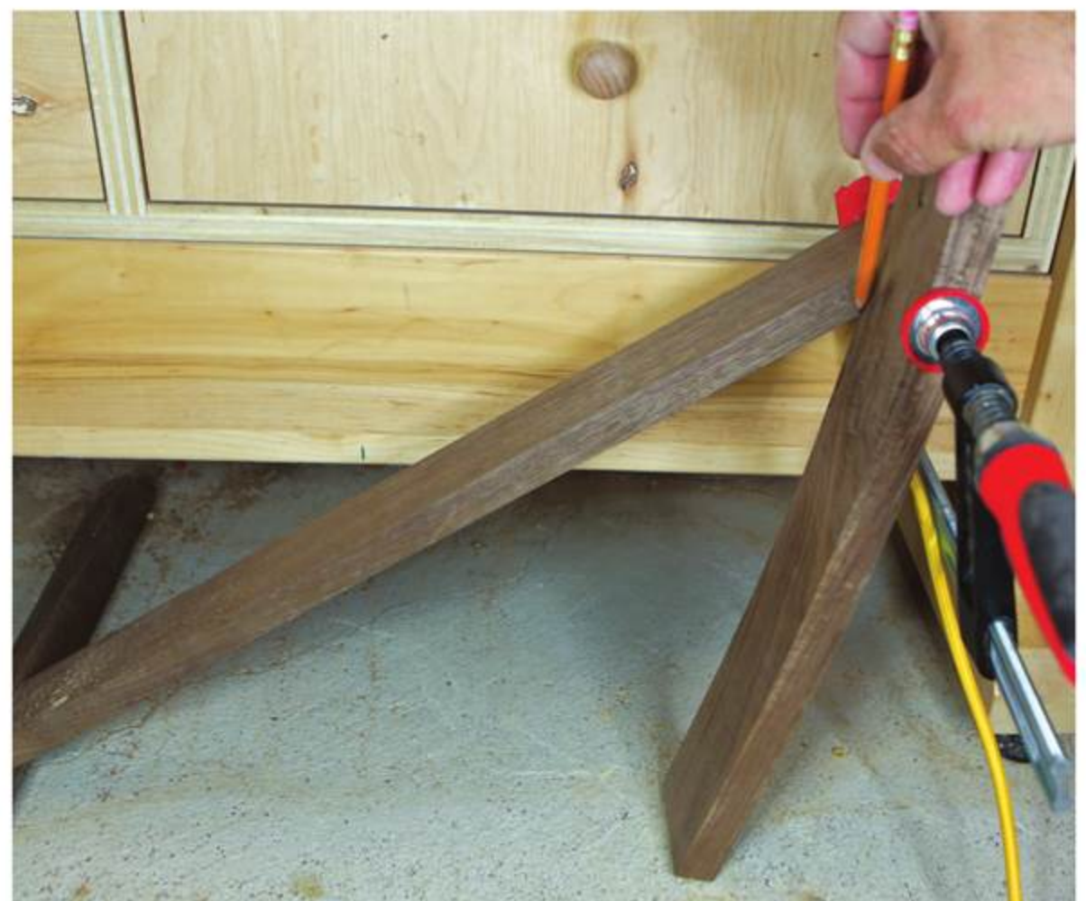
Dealing with Angles – Der-Garabedian rested the end of the bent lamination on the floor and clamped the middle of the lamination to his workbench, at a pleasing angle. He then positioned the leg-to-foot assembly next to the bent lamination at an appropriate angle, clamped it in place, and marked the angle on the leg.
