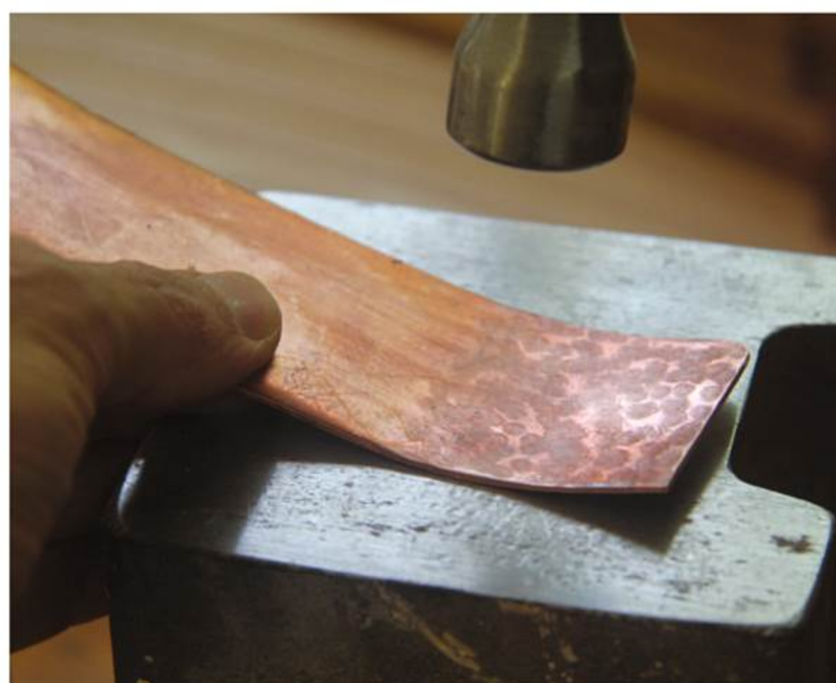
Time to Planish – A ball peen hammer and a hard surface allow small divots to be hammered into the front surface of the copper Brown is shaping. The copper reflector will have to be fine-tuned by hand to fit into the routed groove in the holder.
