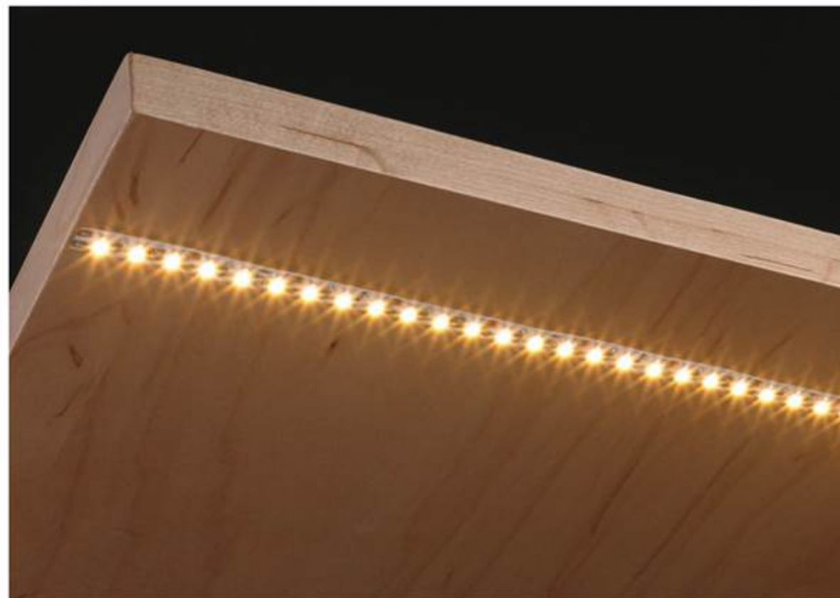
Strip LED Lights – Strip lights are very compact in size, and are flexible. Available in various wattages and densities – the number of LED lights per meter of tape varies from about 20 to 120.
