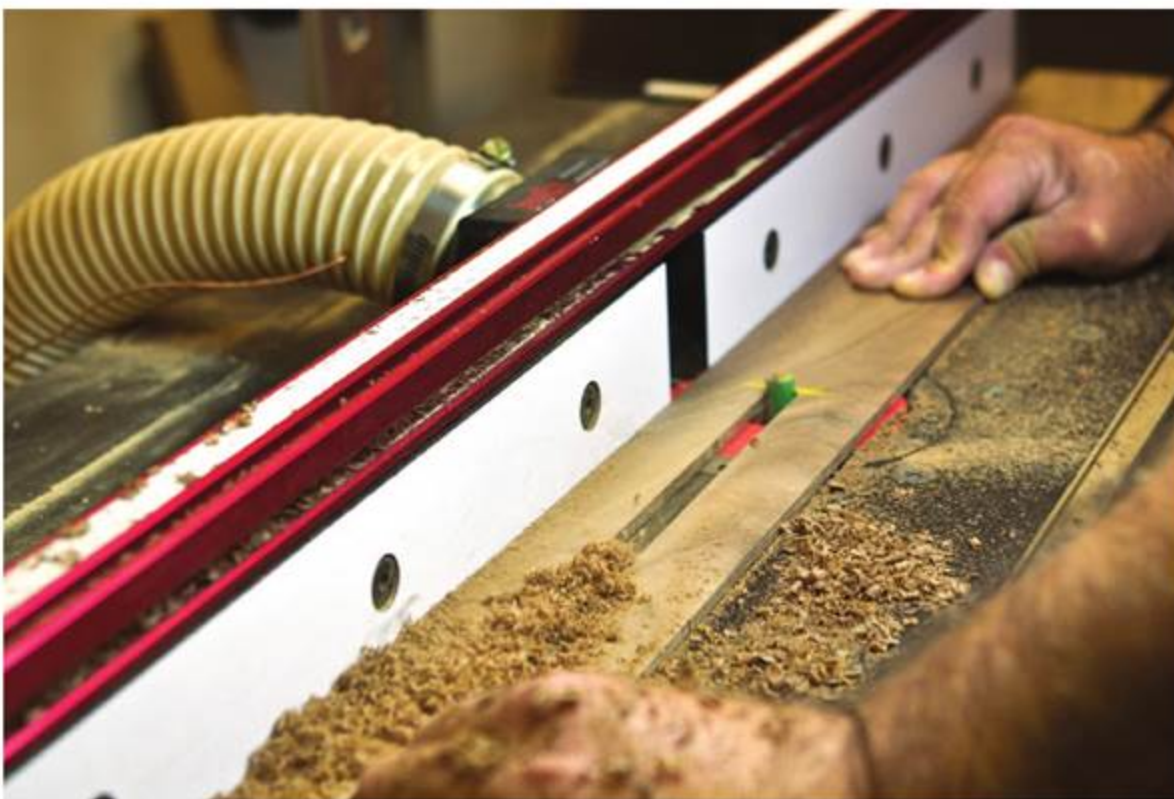
Rout Two Grooves – A router table makes quick work of creating a groove in the middle two laminations. The cord will run in this cavity.
