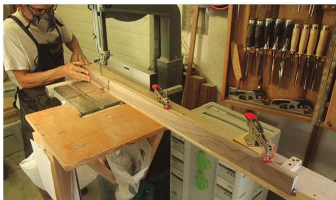
A Small Trim – Each leg is clamped to the jig on a slight angle, so when the jig runs against the bandsaw's rip fence, a taper is cut into the face of each leg.
