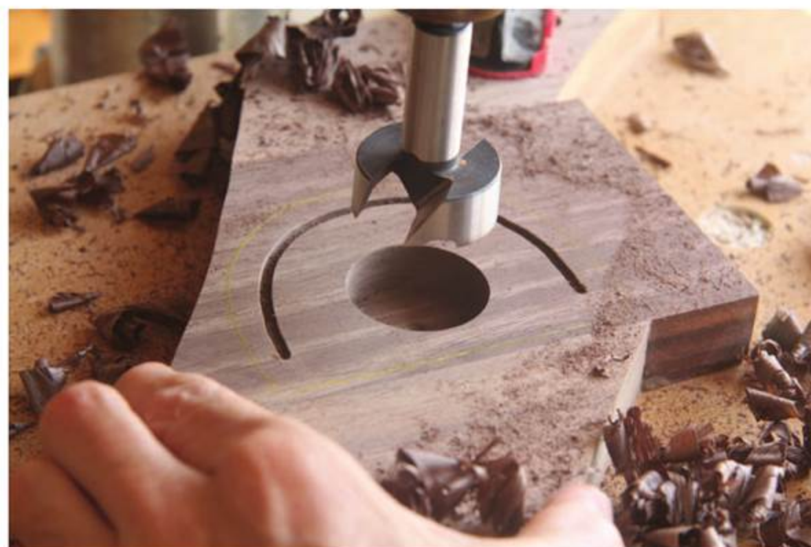
Bore a Hole – Brown finds a 1-1/2" diameter hole works perfectly for tea lights. Drilling it to the perfect depth is also important.
