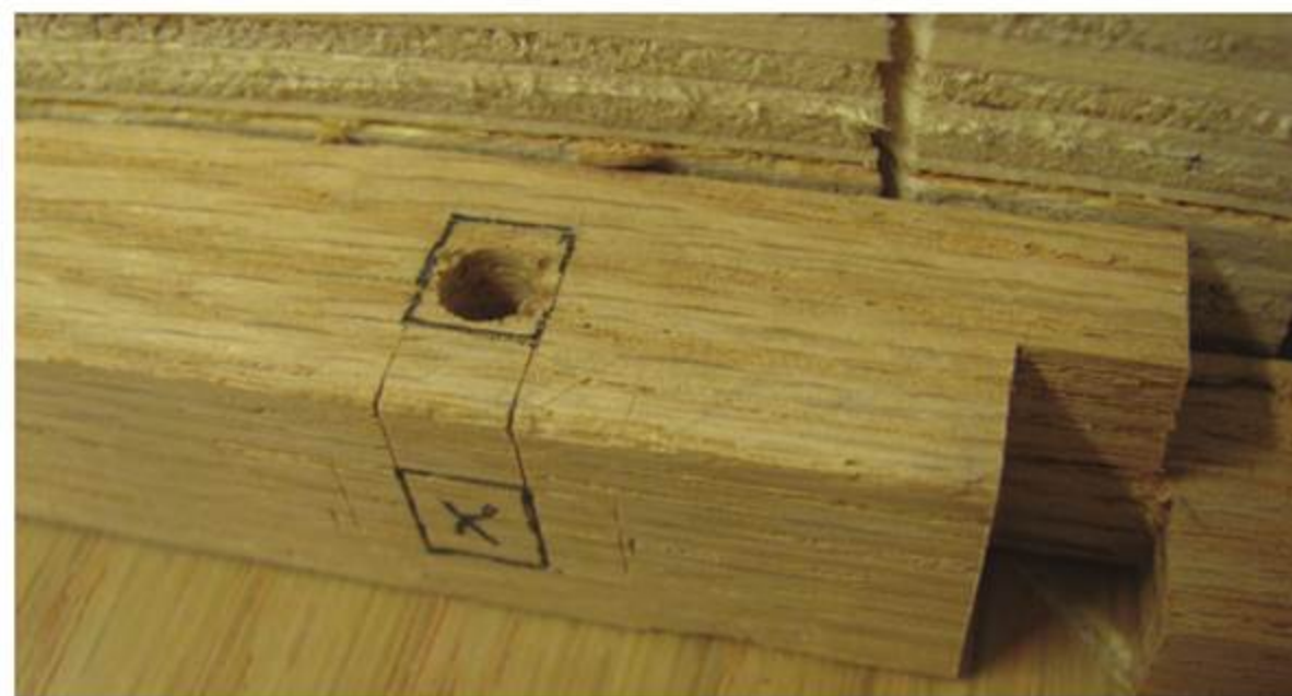
Drill the Chisel – Use a slightly undersized bit to bore a hole in the square mortise before chiselling out the waste to form a square cavity.
