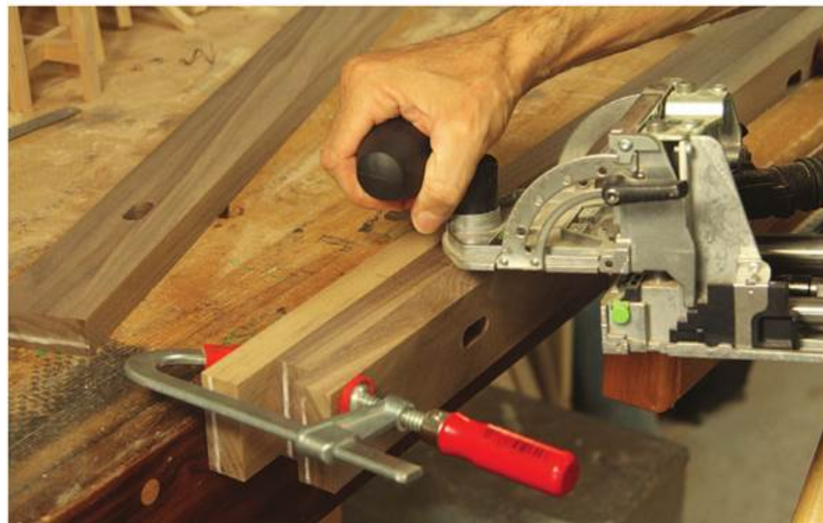
Quick Mortises – The Domino DF 700 makes quick work of mortises. Brown ganged together three legs to offer a larger surface for his machine's fence to reference from.
