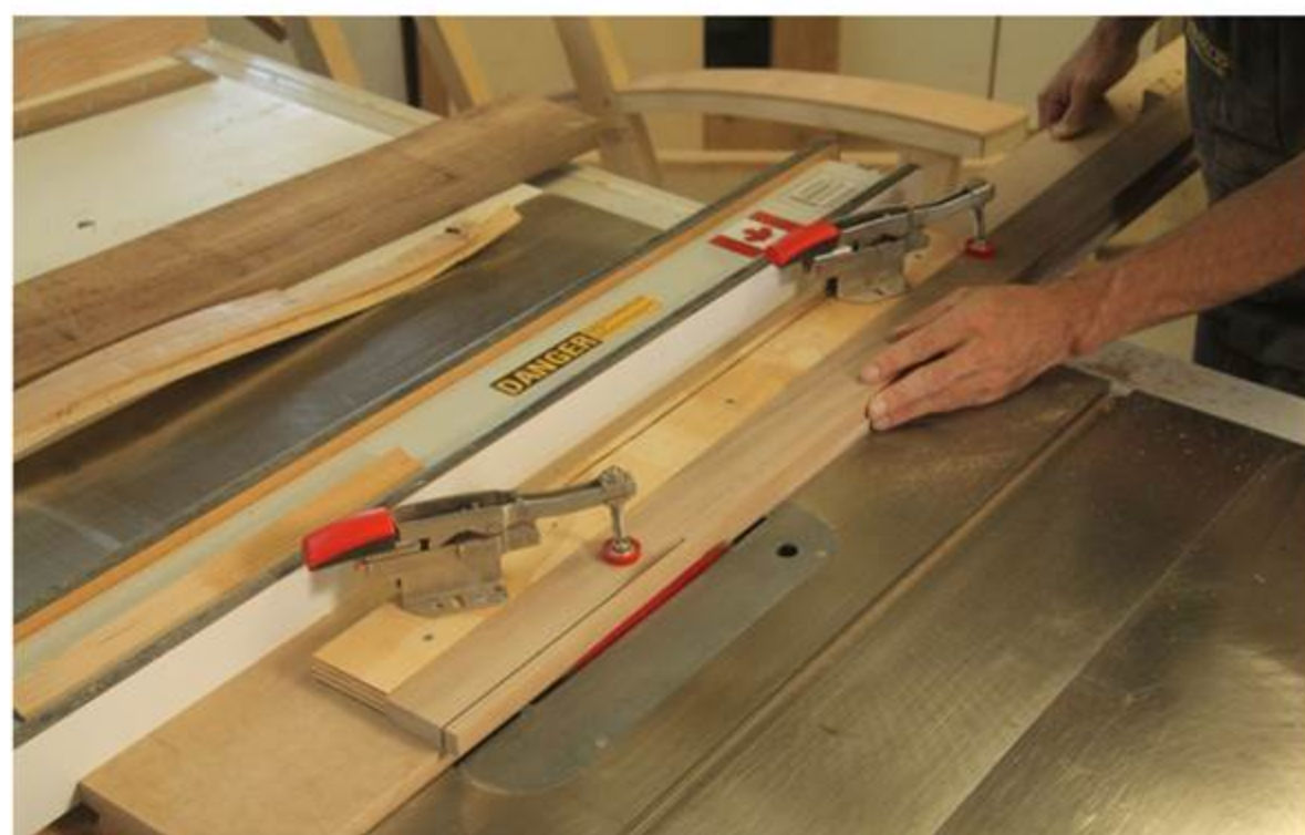
Taper the Sides – Though this operation could also be completed with a bandsaw, Brown chose the table saw to cut the tapers on both sides of each leg.
