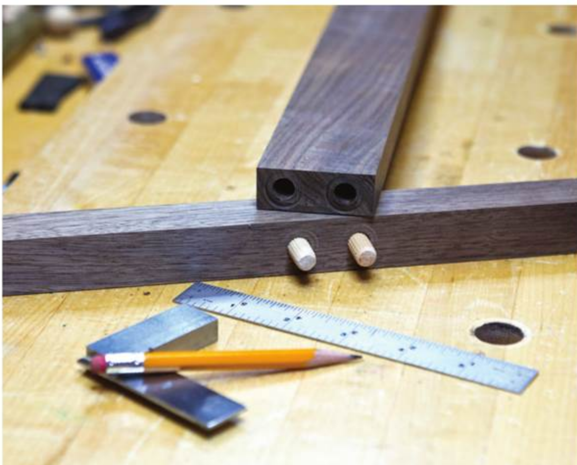
Simple and Strong – A pair of fluted dowels keep the leg-to-foot joint tight. You can use a jig or dowel centers to drill the holes.
