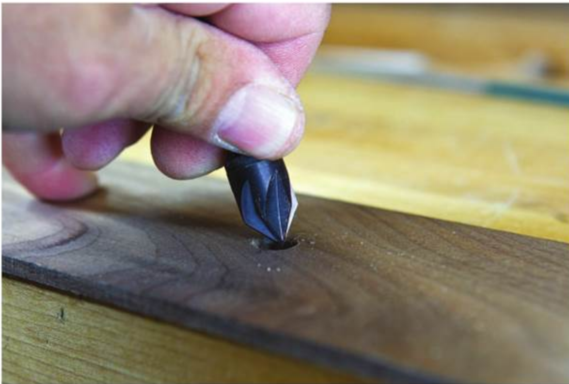
Ease Sharp Edges – A countersink bit or a round file will help ease the sharp edges around the cord hole and ensure the cord doesn't fray.
