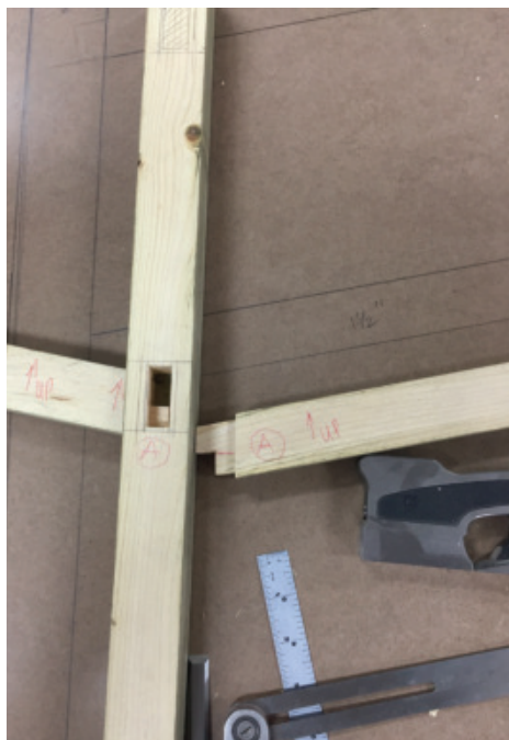
Mock-Up – Maniotakis made a full-sized mock-up of the mortise and tenon joint before starting on the real thing. This allowed him to design and size the joinery to provide the most strength.
