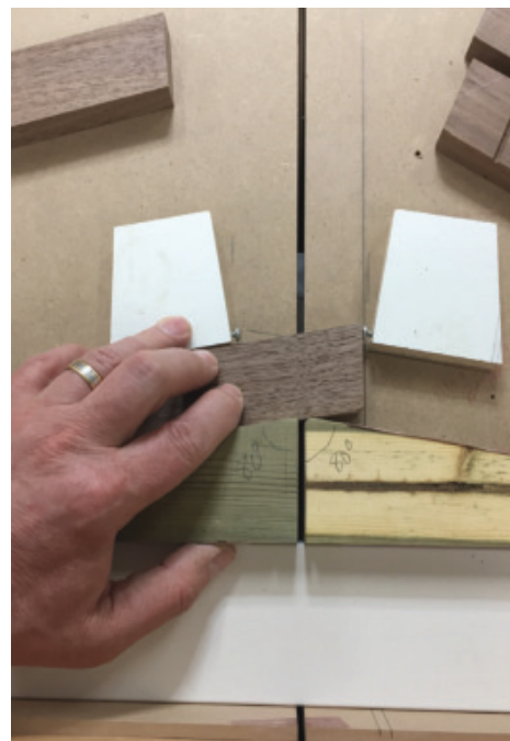
Angled Tenons – With the help of a pair of angled fences, and a couple of stop blocks, Maniotakis easily machined angled tenons on the ends of each rail.
