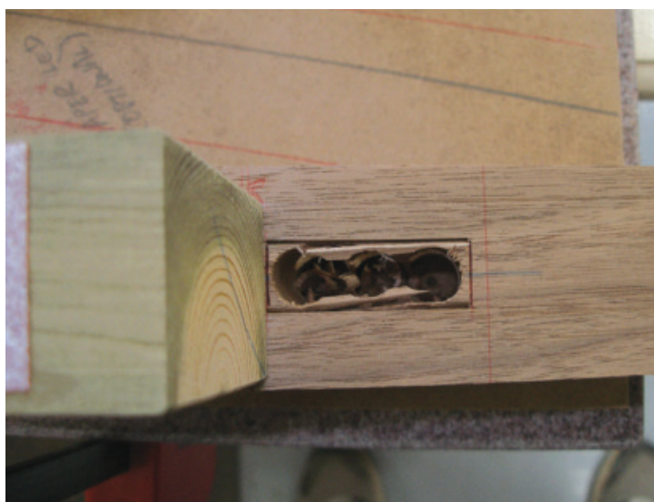
Lower Mortises – Once he drilled out the majority of the waste with a drill bit, Maniotakis used his angled blocks as a chisel guide to help chop the lower mortises. With the block clamped in place, he could place his chisel on the end of the block.
