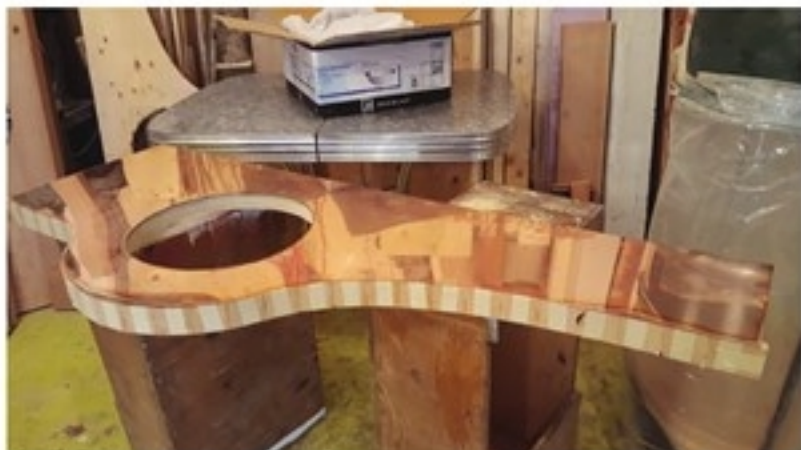
Rough Cut Copper – Rough out the countertop shape and sink hole.
