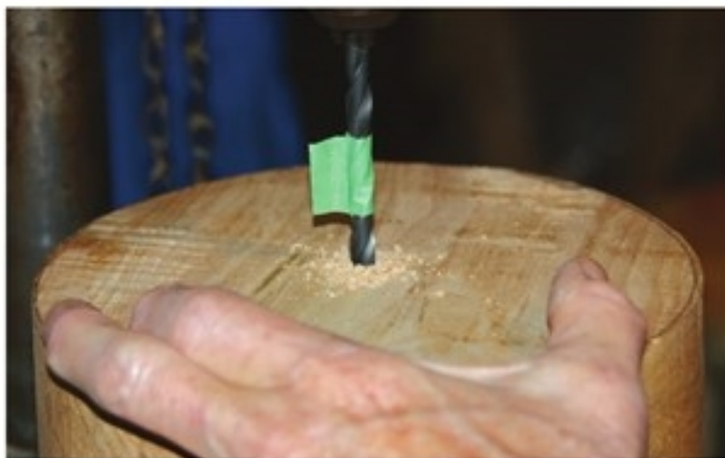
Woodworm Screw – A hole drilled in the blank will allow Cusworth to secure the blank to his lathe.
