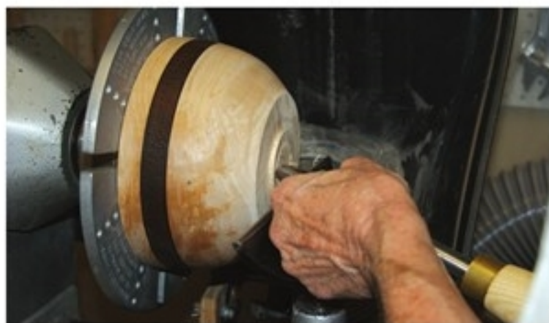
Concave Bottom – Remove the tenon, and create a slightly concave bottom. This will help protect against the bowl rocking on your table when it's complete.
