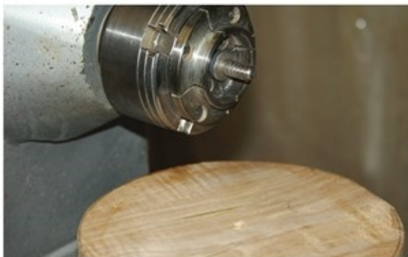
Spin it On – The hole in the back of the blank will thread right onto the Woodworm screw, and ready the blank for turning.
