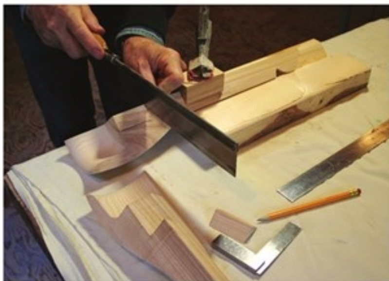
Another Quick Trim – The shoulder for the rail to sit against is created with a hand saw.
