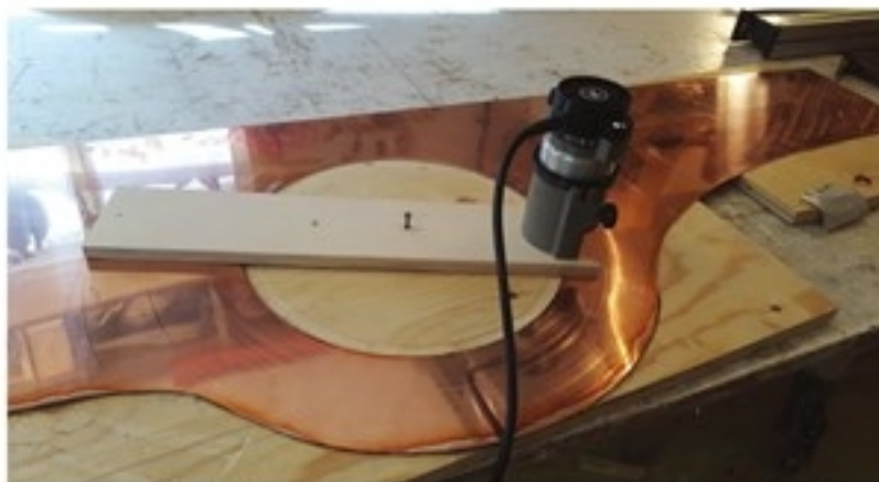
Finish Cut Sink Hole – To avoid damage to the sink, this edge needs to be final and finish sanding before the copper is glued down.
