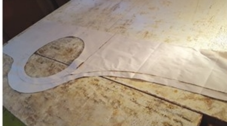
Final Design Template – You can include a lot of information on a top-view drafting. You can even cut out parts to use as subtemplates, like this under-the-counter shelf Schmidt may add later.
