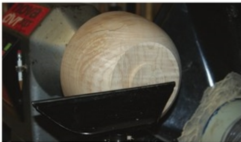
Turn a Tenon – Cusworth shapes the outside of the bowl, then adds a tenon on the bottom of the blank that will be used to secure the workpiece while turning the inside of the bowl.
