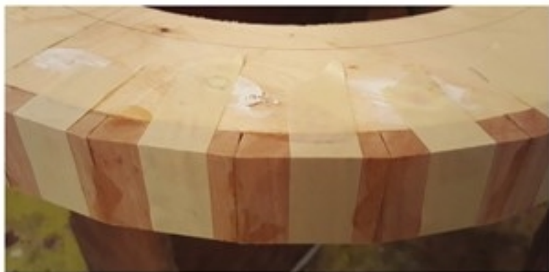
Mark Edge of Sink – Use your router to cut an inset the depth of the sink lip.
