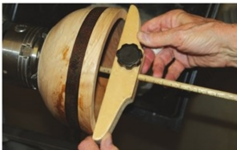
Depth Gauge – A shop-made depth gauge will help you tell exactly how deep your turning is.
