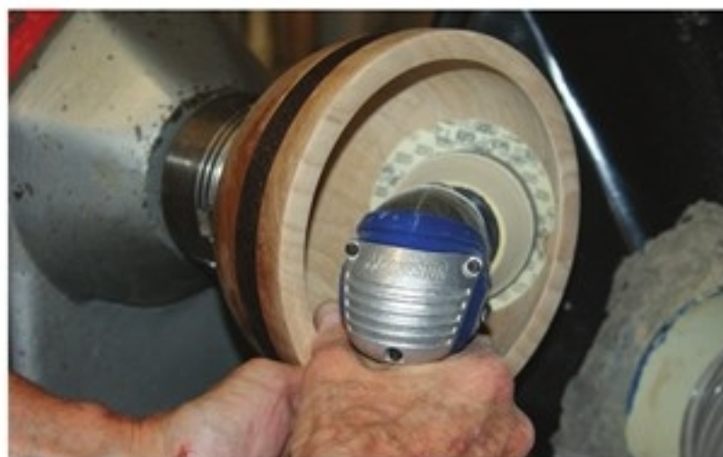
Power Sanding – Sand the inside surface of the bowl to produce a nice, even finished piece.
