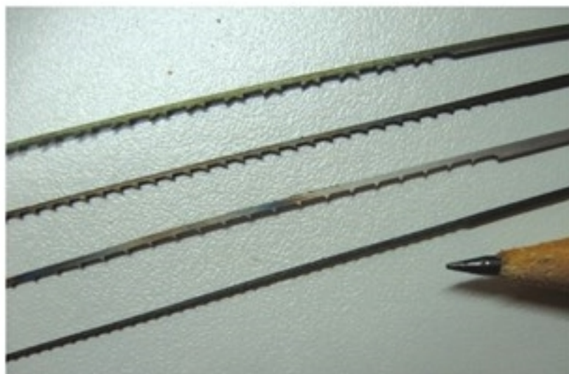
Blade Types – From top to bottom: crown tooth, standard blade, skip tooth reversing and fine reversing blade. Wong finds the bottom two most useful for jigsaw puzzles.
