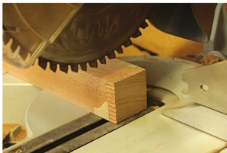
Cut the Lid Off – Because the four sides are finish sanded, Brown adds masking tape where the cut will exit the workpiece. This helps prevent splinters from forming.
