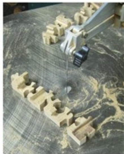
Final Cuts – With the puzzle cut into two layers, it's time to cut the individual pieces out. Be careful not to create pieces that are too weak, as short grain can be your enemy.
