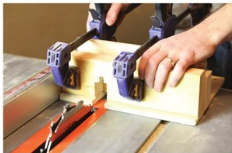
Machine Half Laps in Shelves - Be sure to use an offcut at the back when making your pass through - this will prevent any snipe from affecting a finished shelf. Jessup does this operation with a dedicated jig, but a mitre gauge with a fence to fully support the workpiece can also be used.
