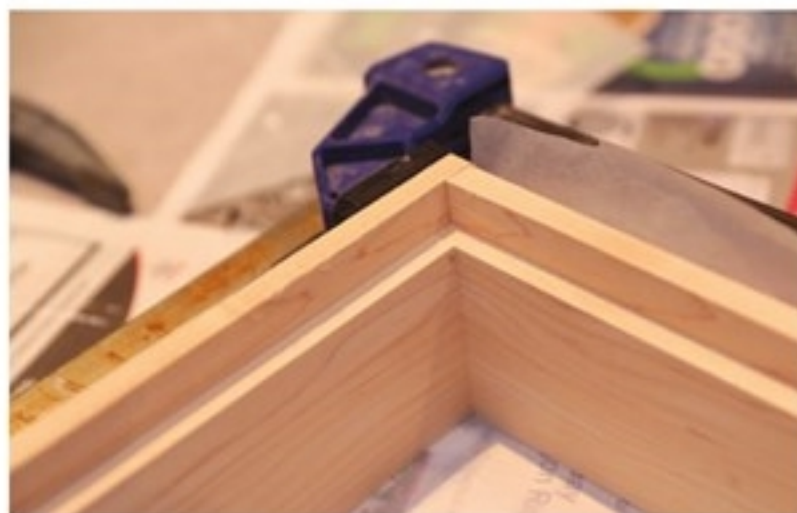
Box Assembly - Use parchment paper over each clamp surface to prevent any glue squeeze-out from sticking the box to the clamp. Ensure the shell is square before leaving it to dry.
