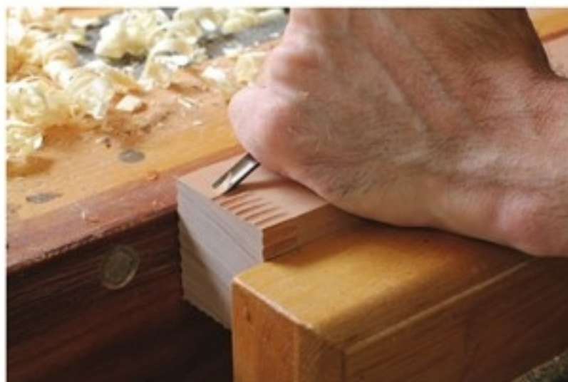
Add Texture – Once the blank has been cut to finished width in both directions, and the top surface has been squared off, Brown adds texture to the sides. For now texture is only added to the top of the box.
