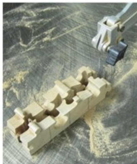
3D Puzzle Pieces – One option is to cut the strips on edge, turning the project into a multi-layer puzzle.
