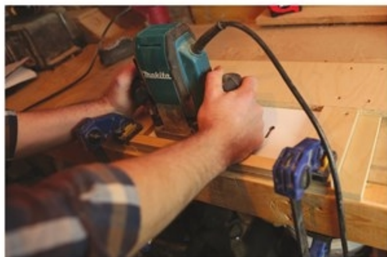
Rout the Keyhole Slots - Jessup has developed a jig to make routing the keyholes more efficient and accurate, but to do just one tie box you can simplify the process. With the back fixed in place, all that is needed is a straight edge for the base of the plunge router for reference, and a start-and-stop block to limit the travel of the router.
